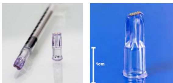
Figure 2-9. Hollow microneedle. MicronJet 600 Needle, device containing 3x0.6mm length; NanoPass Technologies Ltd., Nes Ziona, Israel.
