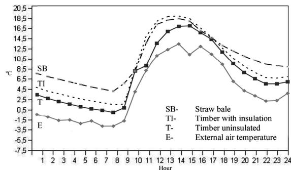
Figure 3: Actual dry-bulb temperatures recorded in physical test chambers 16<sup>th</sup> July 2010, coldest day recorded to-date.
