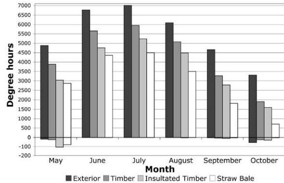
Figure 5: Heating (+) and cooling (-) degree hours calculated from dry-bulb temperature readings in physical test chambers. During winter months May-October 2010
