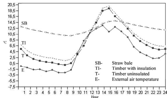
Figure 2: Simulation of dry-bulb temperatures with TAS software 16<sup>th</sup> July 2010, coldest day recorded to-date.
