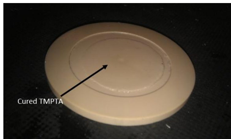
Figure 3-24: Result of the UV dispersion test. The TMPTA was cured by the UV LED held against the glass using the setup shown in Error! Reference source not found. By measuring the size of the cured TMPTA the extent of the dispersion could be determined.
