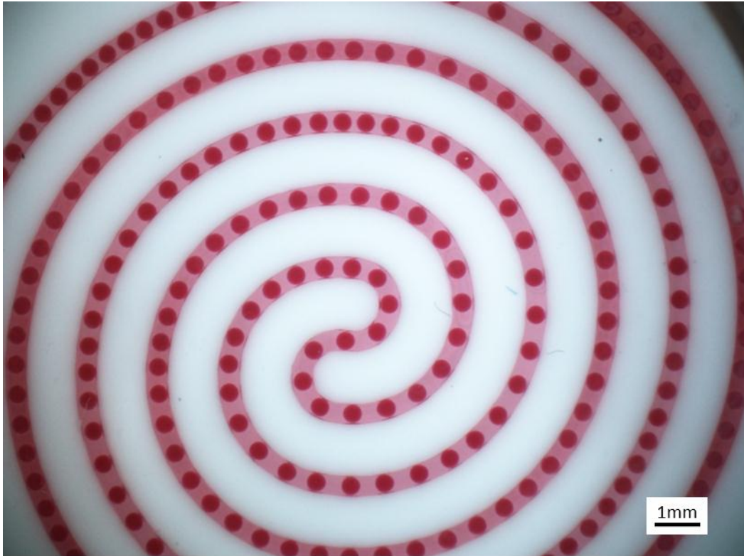
Figure 3-28: TMPTA droplets, in a mineral oil/hexane carrier solution, created on sphere production chip three travelling through the curing region. Droplets appear to have been made in a relatively consistent manner with little variation in their spacing prior to UV curing. Once curing was initiated blockages occurred on a regular basis.
