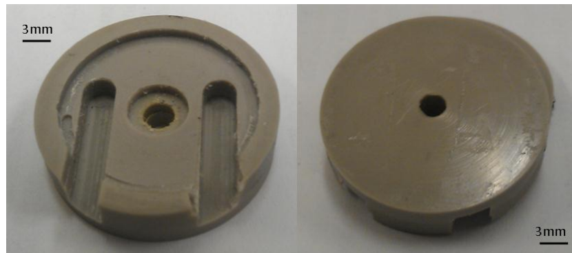
Figure 3-25: LED housing viewed from both the bottom (right) and the top (left). The LED and wiring is placed in the grooves (shown on the left). The housing is then placed against the glass with the bottom of the housing (shown on the right) placed into contact with the glass.
