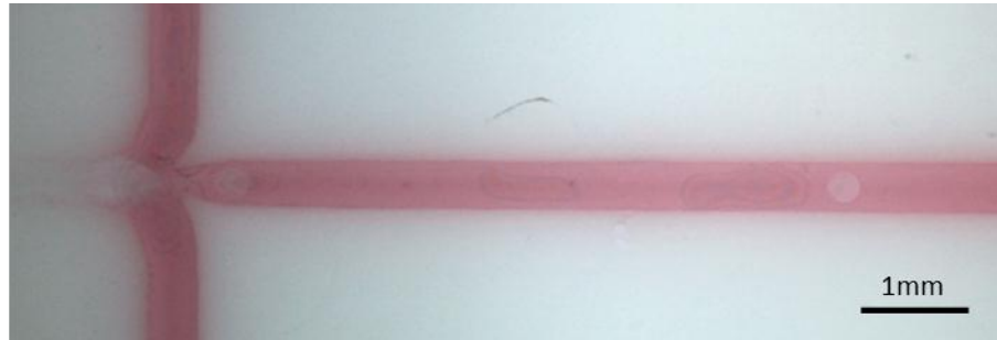
Figure 3-32: Image of the flow focusing junction creating droplets of TMPTA (white) in hexane/oil solution (red). Flow is from left to right.
