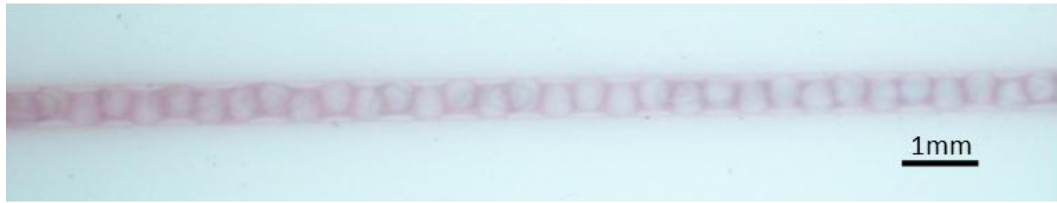
Figure 3-19: Photomicrograph of sphere production chip one showing a chain of cured TMPTA spheres stuck together causing a blockage in the channel.
