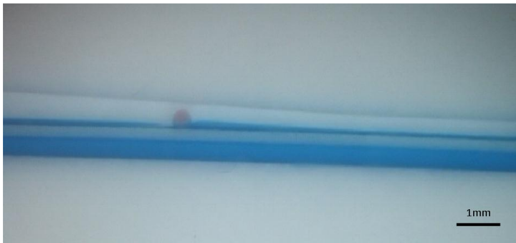
Figure 4-45: Photomicrograph of an alginate sphere (red) being transferred from mineral oil without glacial acetic acid (blue) to mineral oil containing the acid (clear). Flow is from left to right.
