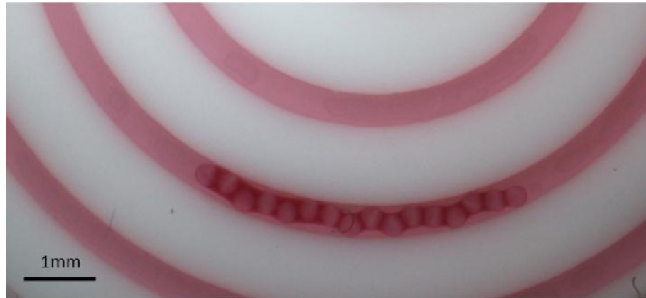
Figure 3-27: Photomicrograph of a TMPTA blockage in the curing spiral on sphere production chip three. Droplets have come into contact during curing and are therefore stuck together.
