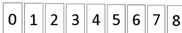
Figure 5-10: Scale illustrations of the average cross-section of the focusing region channel when subjected to a parallel stretch of a given length. The number within each box indicates the extent of the prescribed displacement length (mm). An average is taken of the width and depth data shown in Figure 5-7 and Figure 5-9. The channels have the following width x depth dimensions. 0mm: 80 x 140 \mu\text{m} . 1mm: 79.13 x 138.48 \mu\text{m} . 2mm: 78.26 x 136.96 \mu\text{m} .
