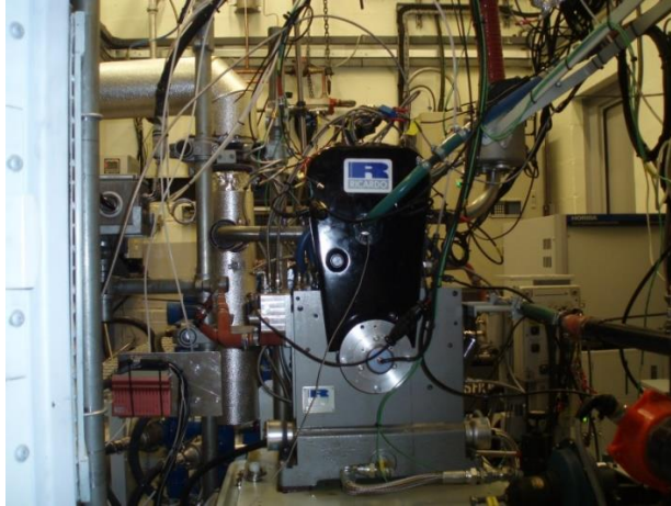
Figure 3.7: Photograph of the single-cylinder spray guided direct injection engine installed on a Ricardo test bed.
