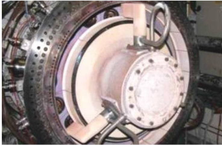
Figure 3.3: Photograph of the combustor exit on a Rolls-Royce fully annular combustor rig, reproduced from [92].
