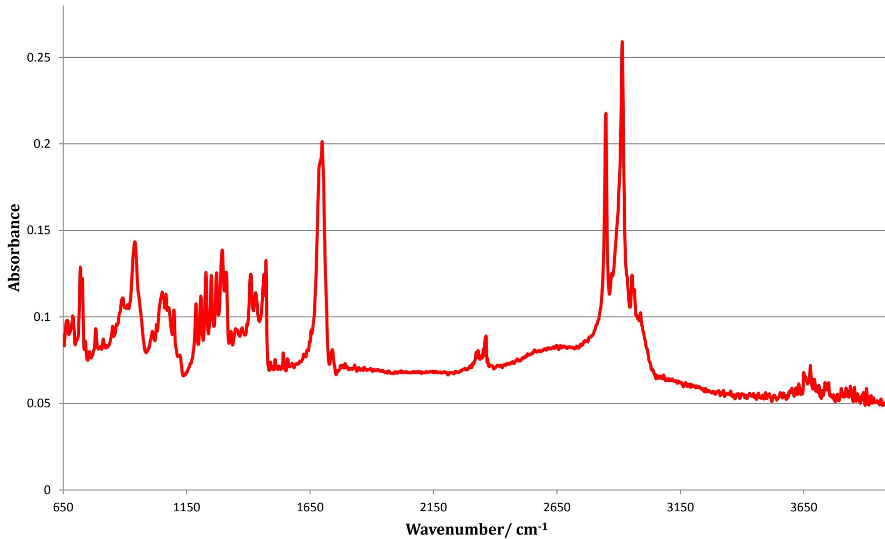
Figure 32 FTIR Spectra of Calcium Palmitate
