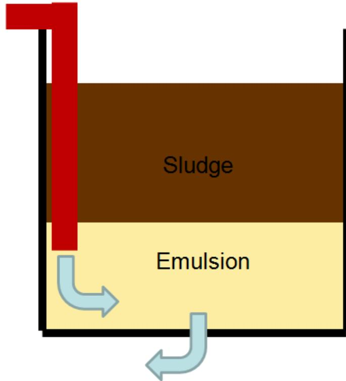
**Figure 46 Cut-Out View of a Wastewater Storage Tank at the Factory**
