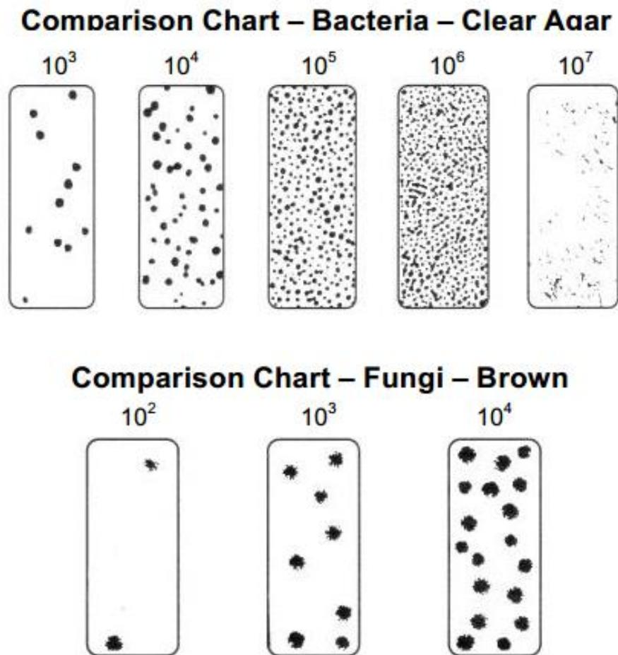
Figure 8 Dipslide Bacterial/Fungal Count (WET, 2005)
