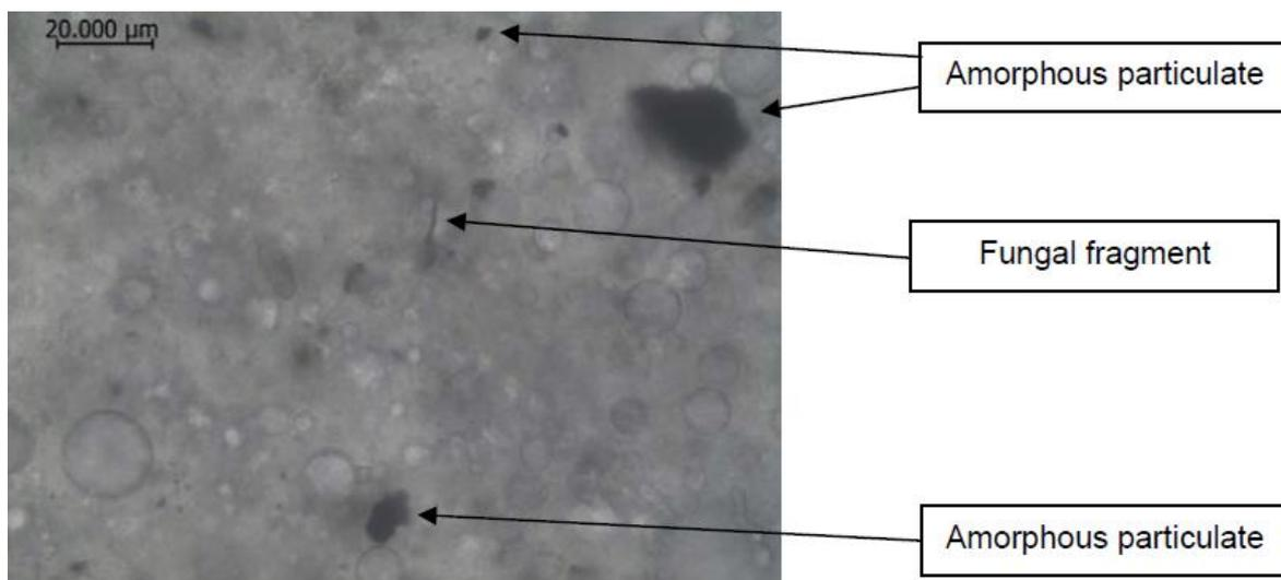
**Figure 19 Microscopic Image of Emulsion within Sludge 2 (ECHA, 2012)**
