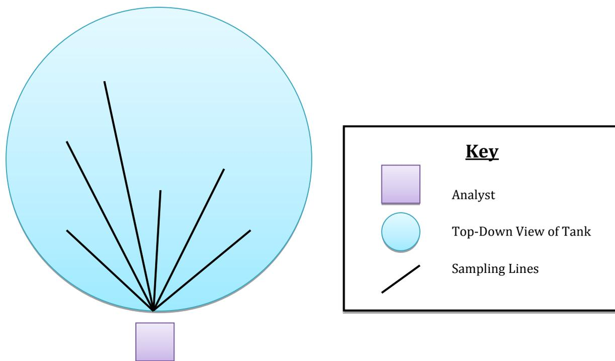
**Figure 6 Sampling of the Tanks Using Bucket and Rope Method**
