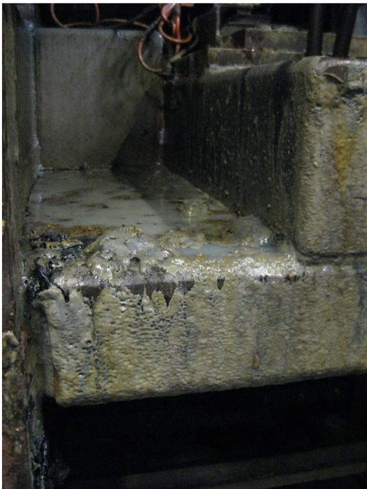
Figure 11 Suspected Biofilm in a Washing System
