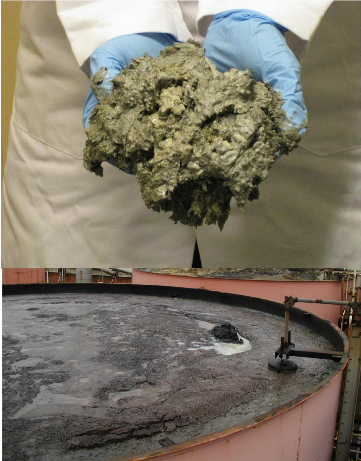
**Figure 2 Examples of Floating Oil-Based Sludge**
