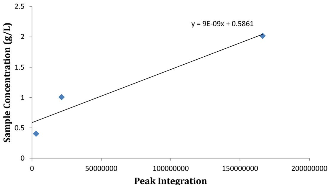
Figure 9 Calibration Curve for Palmitic Acid on the GC-MS
