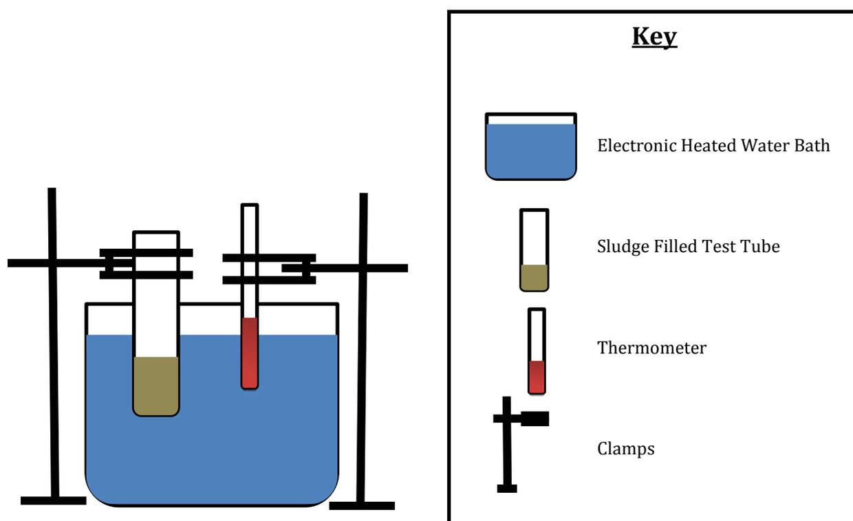
Figure 7 Water Bath Setup for Determination of Sludge Melting Range
