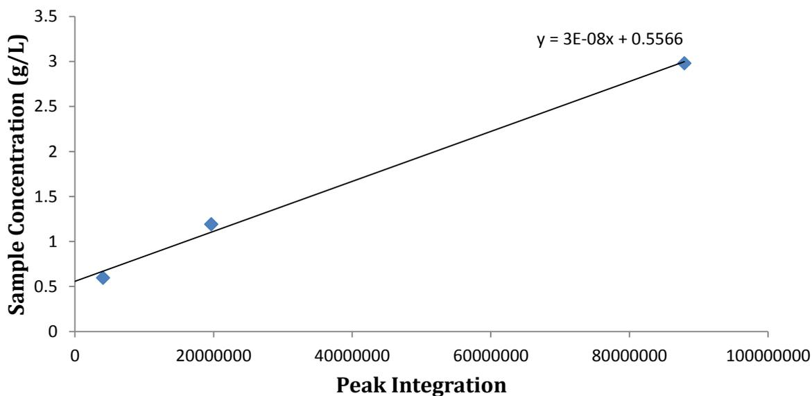
Figure 10 Calibration Curve for Oleic Acid on the GC-MS
