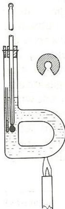
**Figure 4 Example of Melting Point Equipment Setup (Furniss et al, 1989)**
