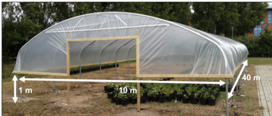
Figure 6.1 Image of modified Polytunnel used as the rain shelter before the start of the drought experiment. Dimensions of width, length and height of gap in plastic are indicated.
