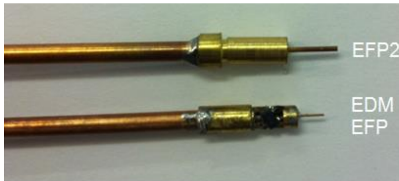
Figure 4.1: Pictorial representation of the reduction in dimensions of the EFP with the use of EDM copper tubes.
