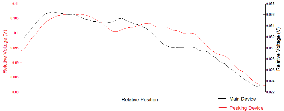
Figure 7.7: Automated spatial resolution scan along the metallisation within section c1 of the main and c2 of the peaking device, showing substantial and coherent variation in the resulting distribution.
