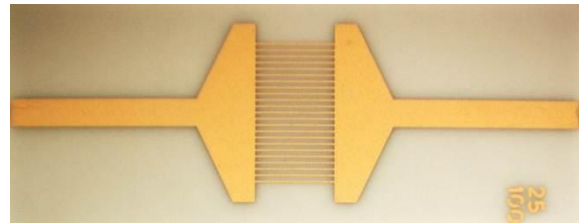
Fig. 4. Resolution test substrate with 25 micron fingers, 100 micron spacing.
