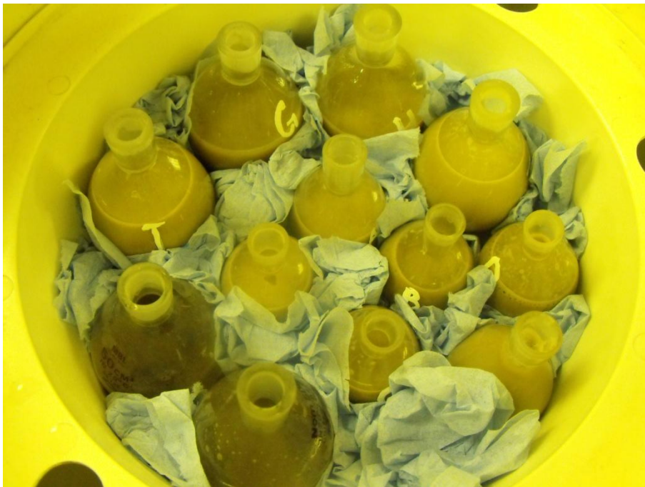
Figure 6-7: Pycnometers with soil samples.
