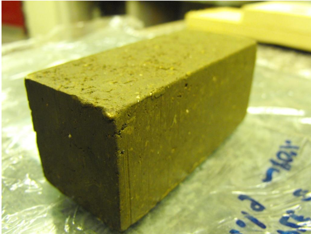
Figure 6-13: Reconstituted sample prepared with the moulder.
