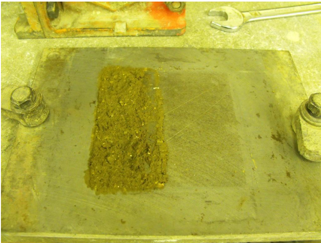
Figure 6-12: Metal base where the samples for the thermal conductivity test were prepared. It can be seen that part of the material stick to the base after preparation. The samples were prepared with additional 1.5 cm height to allow trimming of imperfections at the base.
