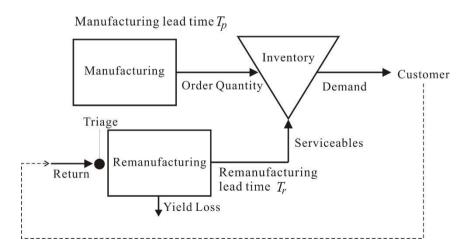
Figure 1. Schematic of material flow
