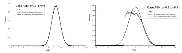
Figure 8. The actual density of the yield verses a normally distributed approximation based on the first two moments
