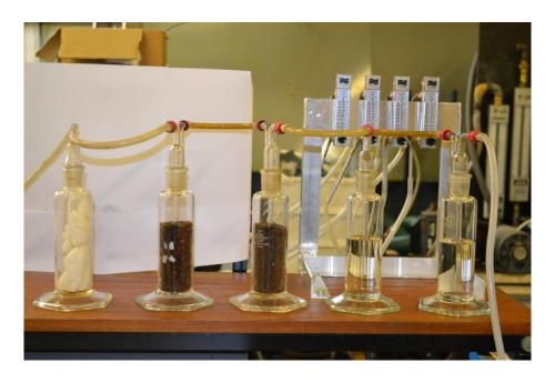
Figure 3.6: A photograph of 5 Dreschel bottles used in the tar trap system
