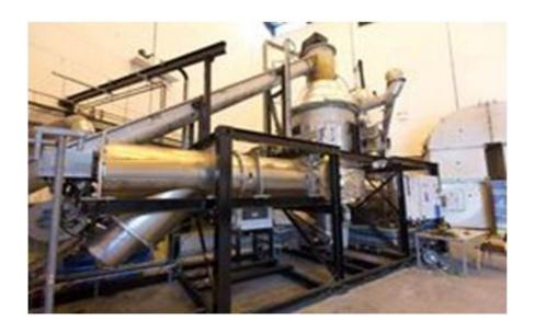
Figure 1.8: Commercial rig 2: Small scale semi-batch pyrolyser
