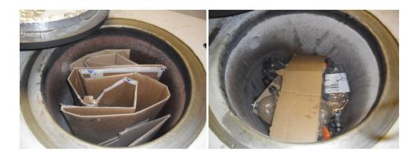
Figure 3.10: Photographs of the cardboard for Run 1 (left) and cardboard and PET for run 2 (right) in the pyrolysis chamber of commercial rig 1
