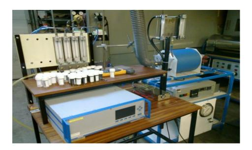
Figure 3.3: A photograph of the pyrolysis reaction rig with Rosemount NGA 2000 gas analyser
