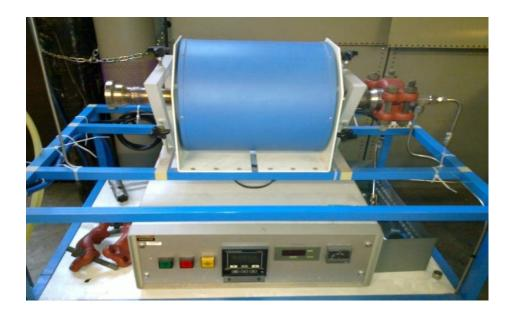
Figure 3.1: A photograph of the horizontal tube furnace
