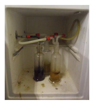
Figure 3.11: A photograph of the three Dreschel bottles inside freezer with 80 ml of IPA collecting tars during run 2
