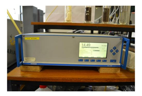
Figure 3.7: A photograph of the Rosemount NGA 2000 gas analyser
