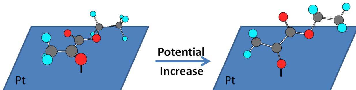
**Figure 6.13** Schematic changes of the orientation of EP on Pt surface with the increase of the potential.
