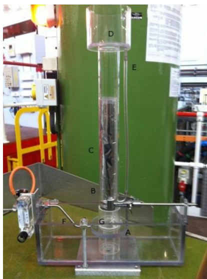
Figure 2.8; SANS sample environment for studying foams.
