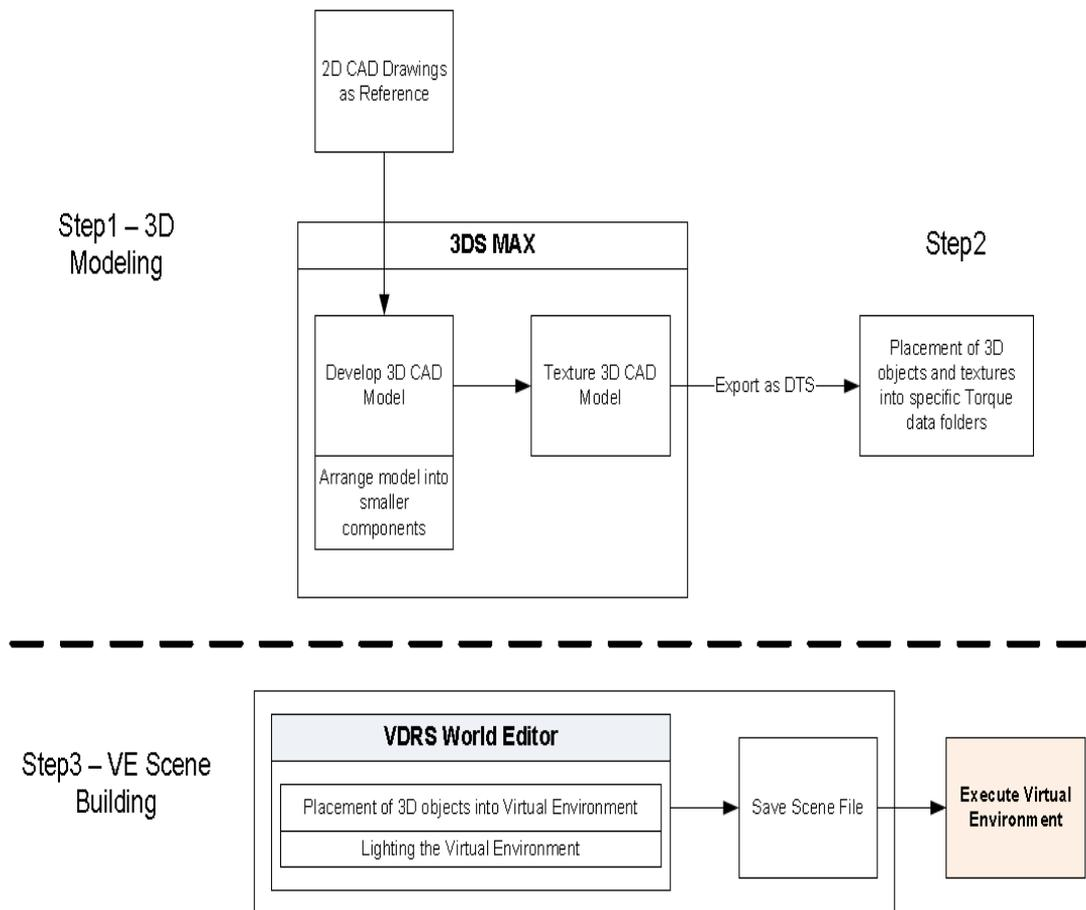
Figure 2.9 The workflow from 3D CAD into the VDRS (Shiratuddin 2011)
