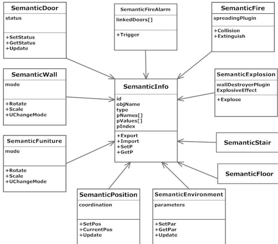
Figure 3.4 Interactive diagram between classes for dynamic scenarios generation
