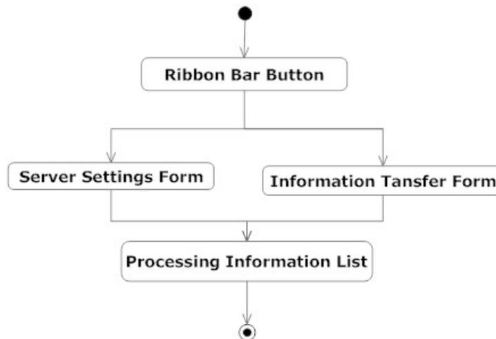
Figure 4.3 The appear order of forms contained in the Revit plugin
