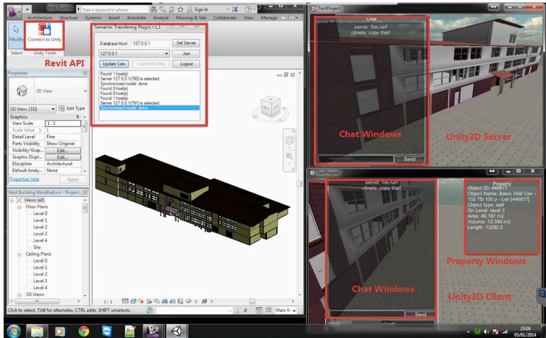
Figure 5.1 Autodesk Revit plugin to extract building information to the BIM-VE
