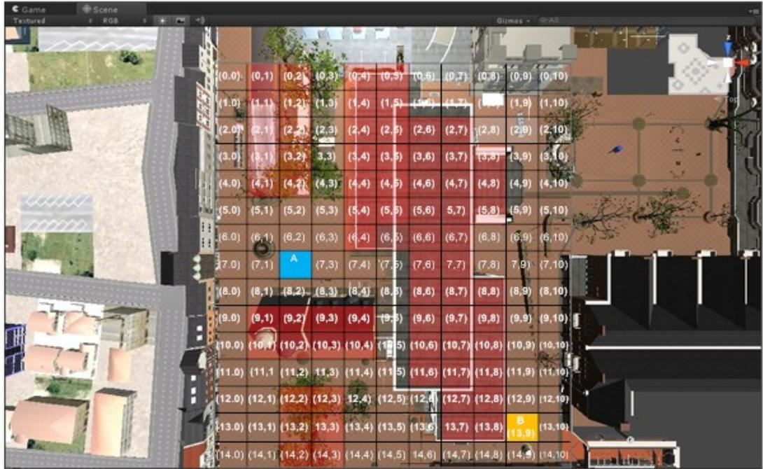
Figure 4.17 Define the world within the grid coordinate (obstacle tiles in red colour area)
