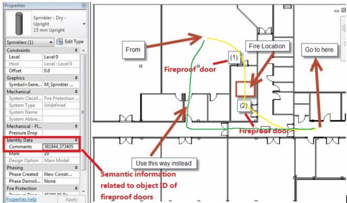
Figure 5.20 The scenario of the fire alarm works with semantic information to automatically change the fire evacuation path ((1) and (2) are fireproof doors which IDs are 381844 and 373405 and referenced to the fire alarm/sprinkler; yellow route is original evacuation path and the green route is the alternative path when fire alarm is activated)
