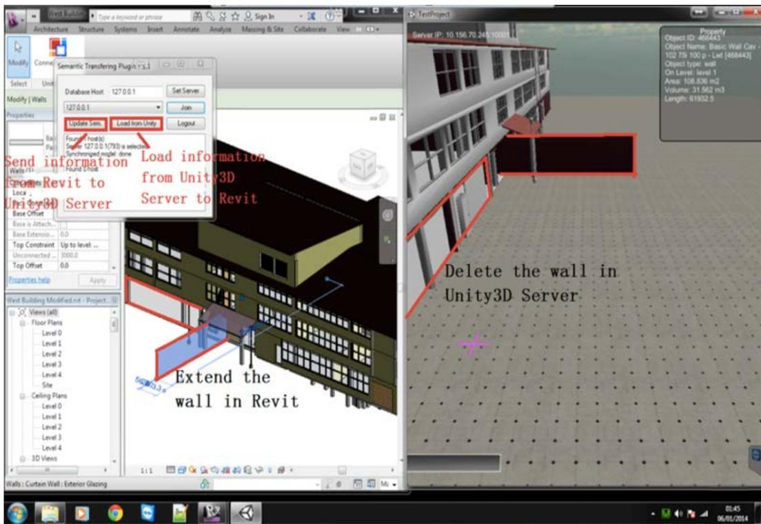
Figure 5.17 The bi-directional information transferral of the Revit API for building design
