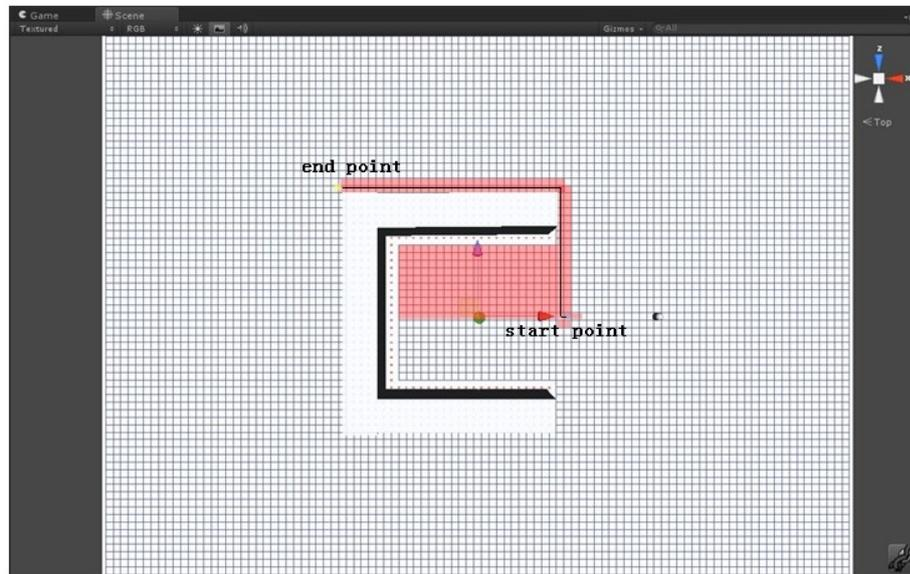
Figure 4.11 The shortest path from start point to end point based on A\* space searching algorithms
