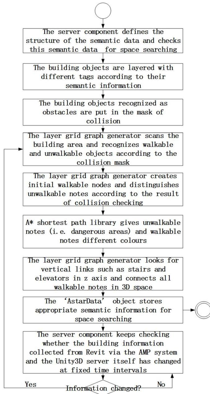
Figure 4.20 Workflow to create preliminary coloured 3D discretised space for shortest evacuation path
