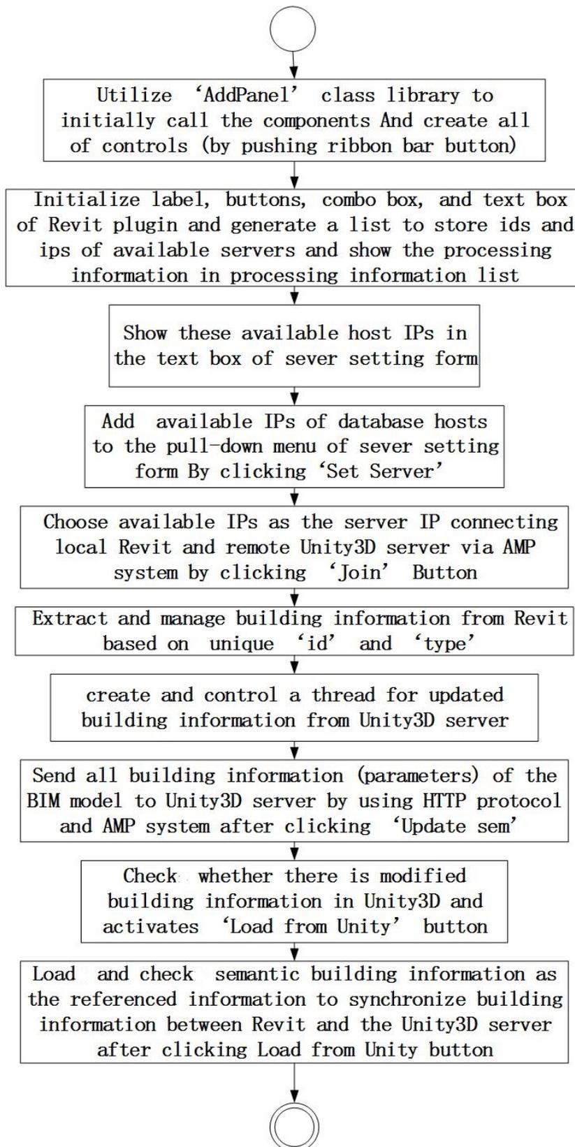
Figure 4.4 The basic workflow process that goes on inside of the plug-in
