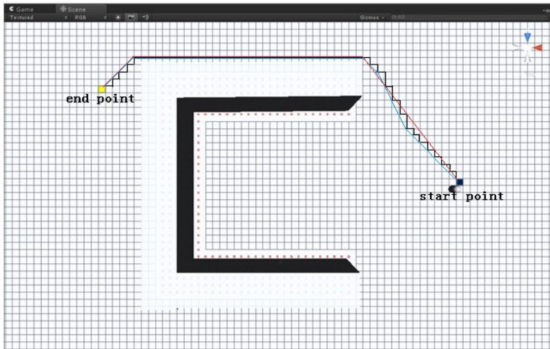
Figure 4.12 The shortest path generated by A\* algorithm with different  $h(x)$
