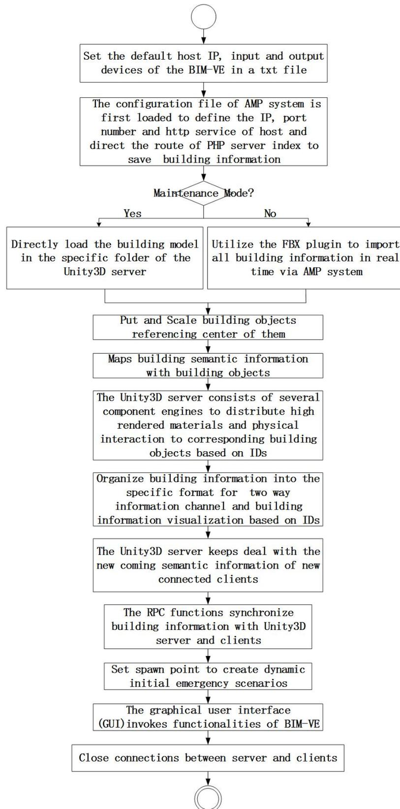
Figure 4.8 The workflow of server-clients framework for information and functionality control
