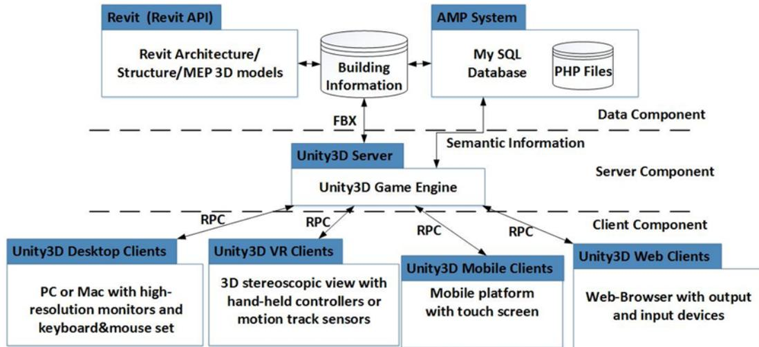
Figure 3.2 System Architecture
