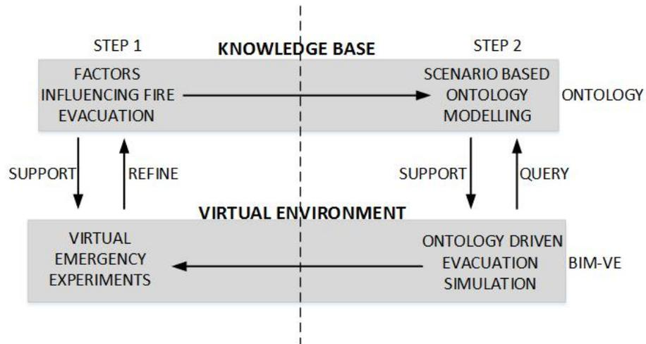
Figure 4.38 Two steps to organise the evacuation ontology and enable evacuation simulation
