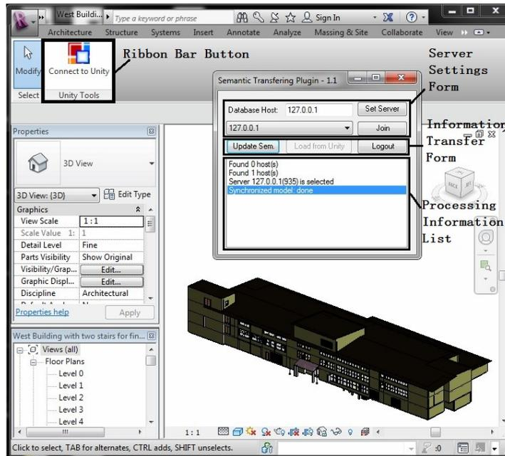
Figure 4.2 The layout of the forms within the Revit plugin
