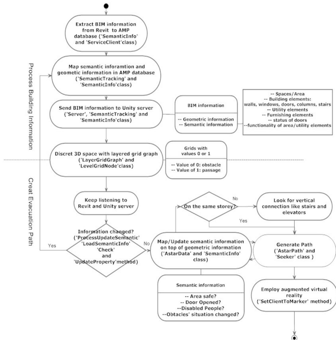
Figure 4.19 The workflow with associated classes and methods for the implementation of the path finding algorithm in the BIM-VE
