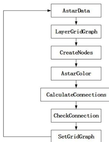
The flowchart of main classes and methods to generate coloured layered grid graph
