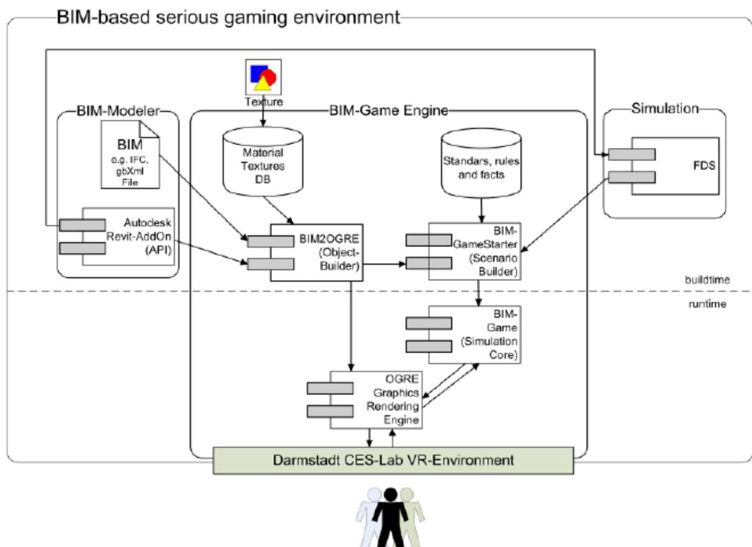
Figure 2.8 BIM-based serious gaming environment (Rüppel and Schatz 2011b)
