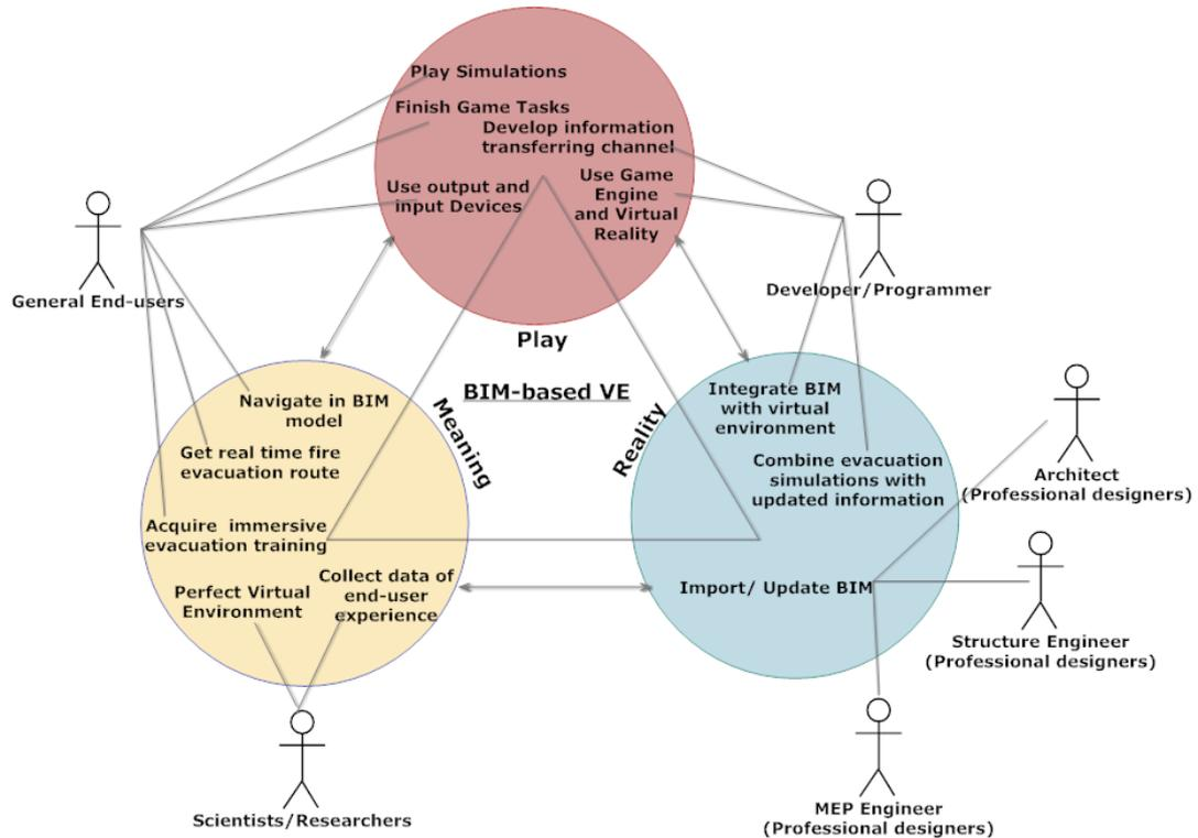
Figure 3.1 Adapted TGD based framework for BIM-VE development
