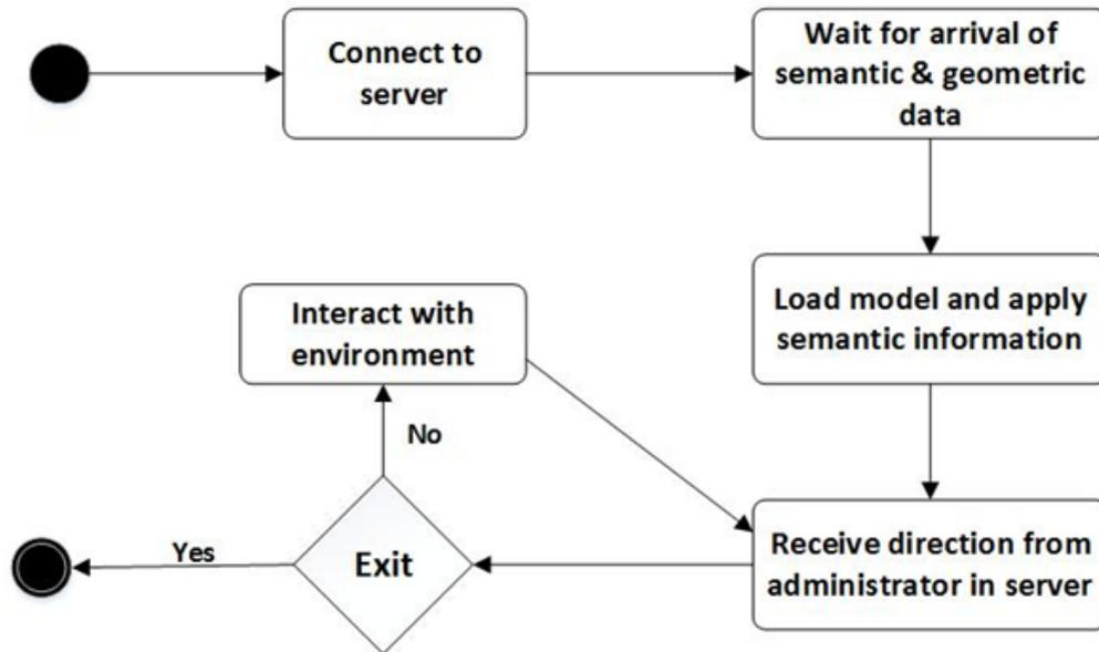
Figure 3.6 Client end work flow
