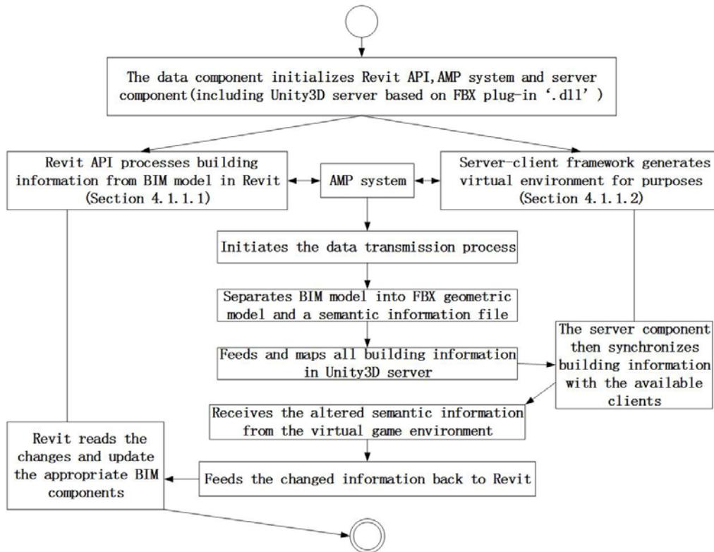
Figure 4.1 AMP system for two way information communication
