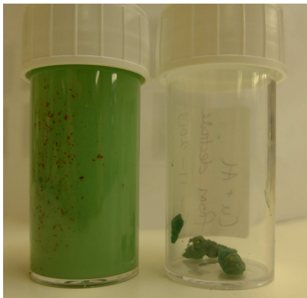
Figure 91: Unfiltered Cwm Rheidol sludge and dried sludge produced in the EC reactor after 60 min treatment time with Cu + Al electrodes.
