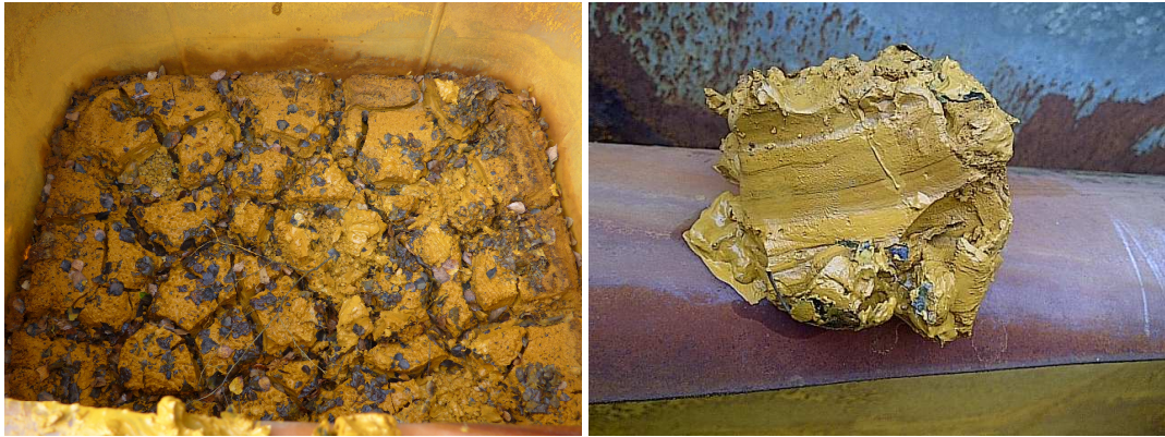
Figure 35: Left is the ochre bed of the VFR after having been drained. Right is a section of the ochre bed taken for lab analysis.
