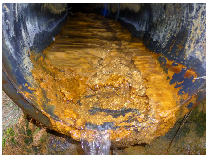
Figure 71: Sampling location of the Cwm Rheidol pipe sludge at the end of the No. 9 adit drainage pipe. Width of pipe 300 mm.
