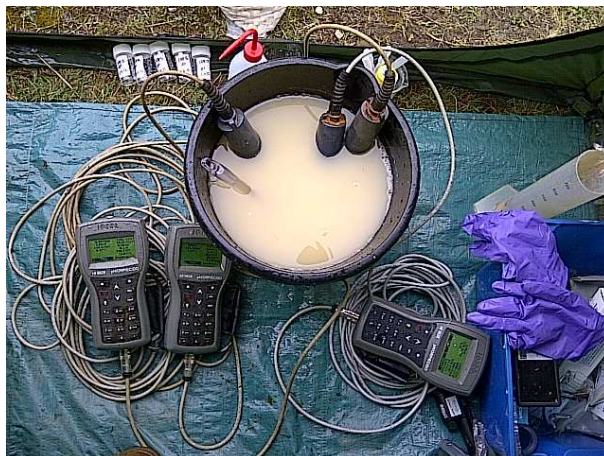
Figure 32: Cwm Rheidol mine water with limestone added.
