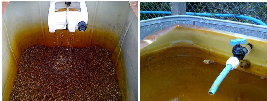
Figure 27: Initial stages of filling the VFR. Left: Shortly after seeding the VFR; right: First time filled VFR plus inflow pipe.
