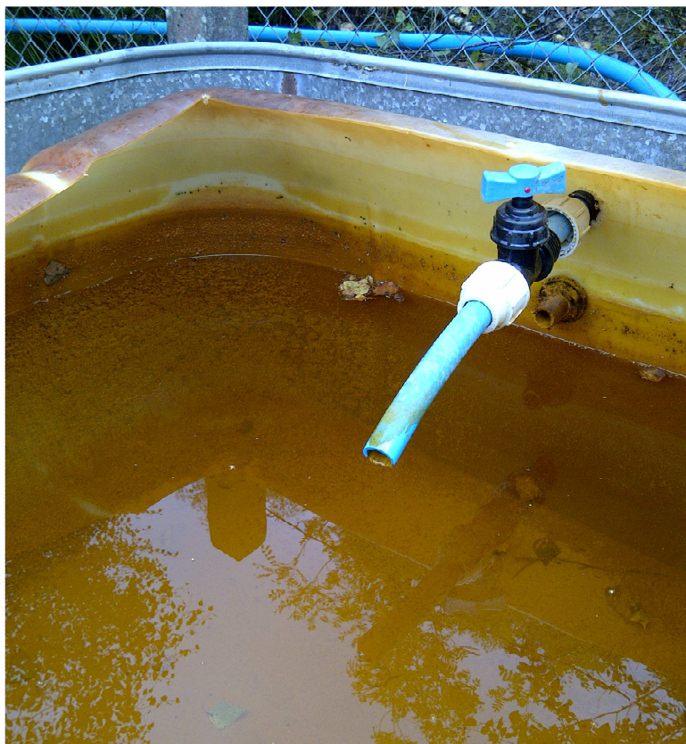
Figure 72: Height of the Fe precipitates in the VFR during the trial is approximately 40 cm from the top of the gravel. Inflow temporarily turned off.
