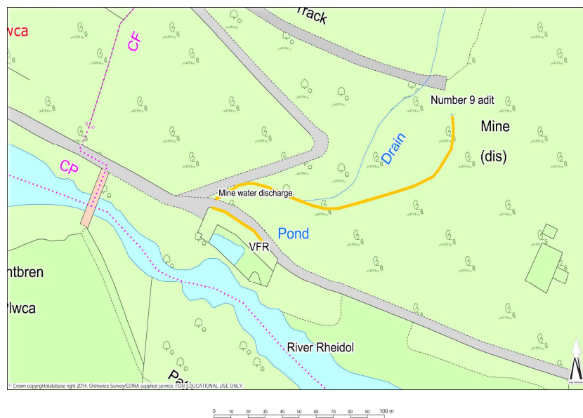
Figure 29: Map showing the aerial position of the VFR at the old filter bed area at the Cwm Rheidol site. The orange line shows the feed pipe from the number 9 adit into the tank. Digimap ® – © Crown copyright/database right 2014. Ordnance Survey/EDINA supplied service. FOR EDUCATIONAL USE ONLY.
