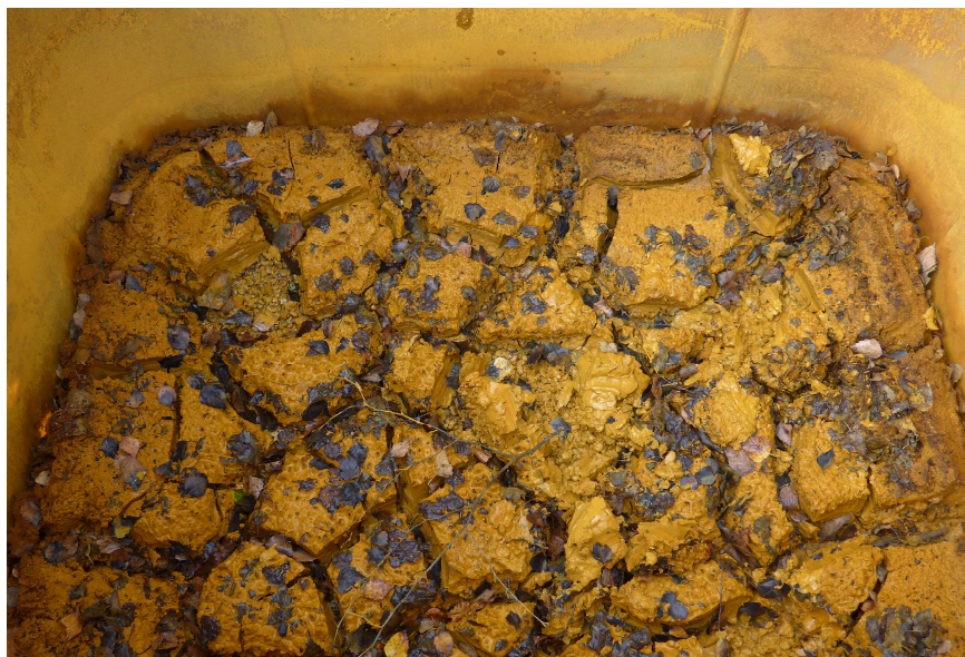
Figure 73: Height of Fe precipitates in the VFR after it had been drained is approximately 6–7 cm from the top of the gravel bed.
