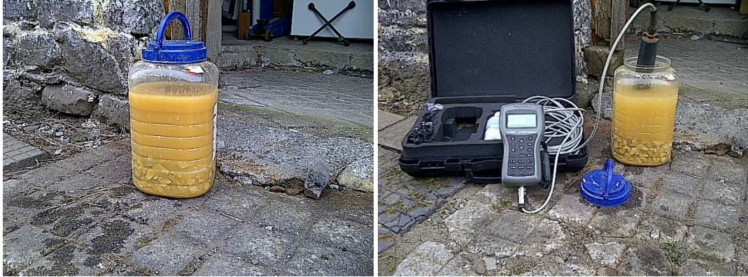
Figure 33: Left image is the Limestone reactor (closed system) Right image, parameters being measured prior to the stripping phase.
