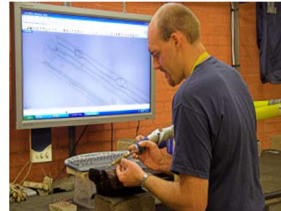
Figure A.5 Geometry capture using FAROArm Source: Newport Museum Service
