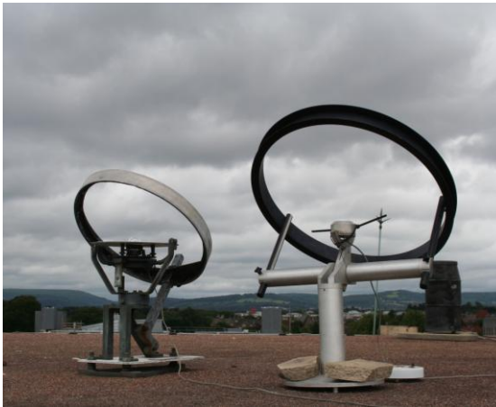
Figure 3: External illuminance meter on the roof of the university building
