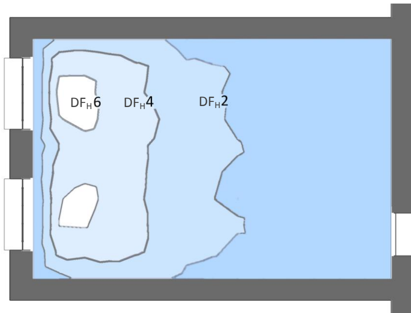
Figure 8.8: Horizontal DF contour plan of Case Study room
