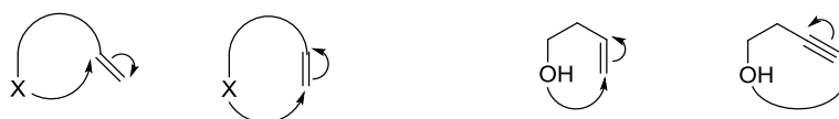
Scheme 30. Example of an exo and endo reaction (left); 5- endo -trig and 5- endo -dig cyclisations (right).
