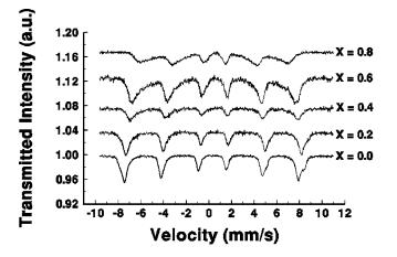
FIG. 1. Raw transmission Mossbauer data for  $CoFe_{2-x}Cr_xO_4$  where x = 0.0, 0.2, 0.4, 0.6, and 0.8 (in order, bottom to top).
