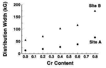
FIG. 4. Hyperfine distribution width as a function of Cr content (x) in  $CoFe_{2-x}Cr_xO_4$ . (Identification of A and B sites is discussed in the text.)
