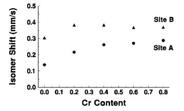
FIG. 5. Isomer shift as a function of Cr content (x) in  $CoFe_{2-x}Cr_xO_4$ . (Identification of A and B sites is discussed in the text.)
