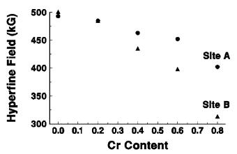
FIG. 3. Hyperfine field strength as a function of Cr content (x) in  $CoFe_{2-x}Cr_xO_4$ . (Identification of A and B sites is discussed in the text.)
