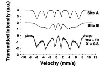
FIG. 2. Experimental Mossbauer data and fit with two six-line hyperfine patterns for  $CoFe_{1,2}Cr_{0,8}O_4$  (*x*=0.8).
