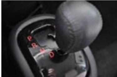
To start, depress the foot brake and release the parking brake. For shift lever position "P" to "D" and go releasing the foot brake progressively, causing their movement was ahead.
