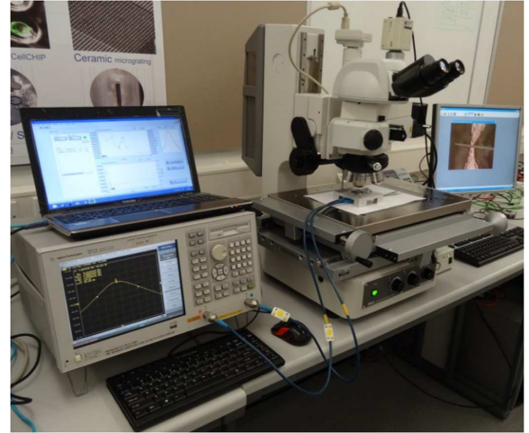
Fig. 9. Photograph of the assembly of the sensor, network analyzer, laptop computer and optical microscope to aid positioning of the polystyrene microspheres in the gap region.
