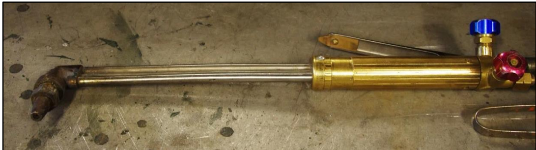
Figure 6.1 Oxypropane torch used by practitioner PA.
