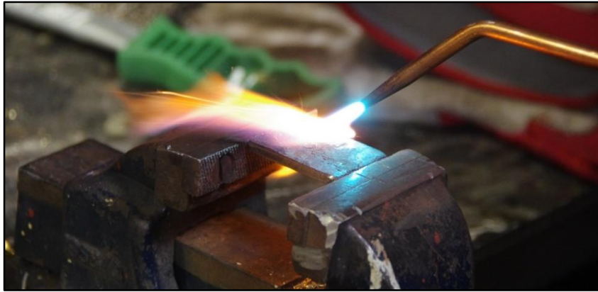
Figure 6.6 Position of the oxyacetylene torch relative to the sample during flame cleaning by practitioner PC.
