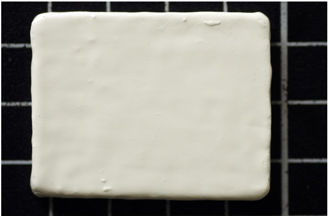
Figure 5.38 Sample HSII08 showing pinholes in cured System A topcoat (scale of background squares 10 x 10mm).
