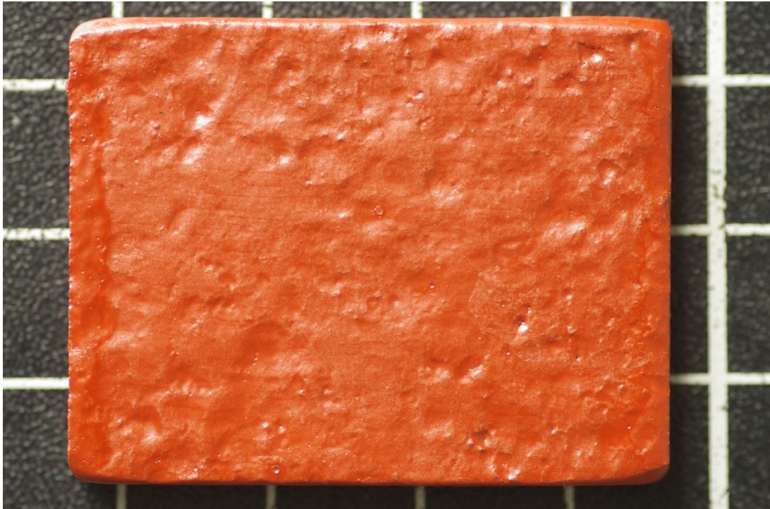
Figure 5.39 Sample HSII16 showing pinhole holidays in cured System B primer (scale of background squares 10 x 10mm).
