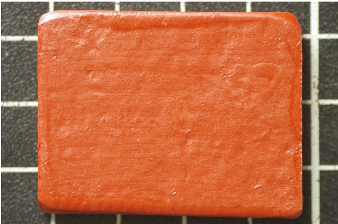
Figure 5.40 Sample HSII13 showing brushstrokes in cured System B primer (scale of background square 10 x 10mm).
