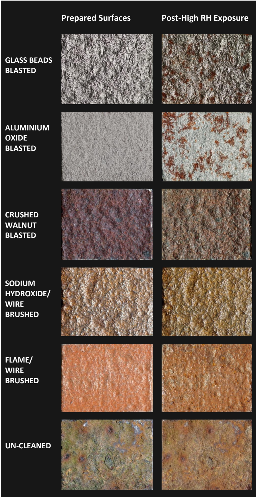
Figure 5.19 Comparison of prepared and post- high RH exposure surfaces. Images show sample surfaces of 30mm x 40mm.
