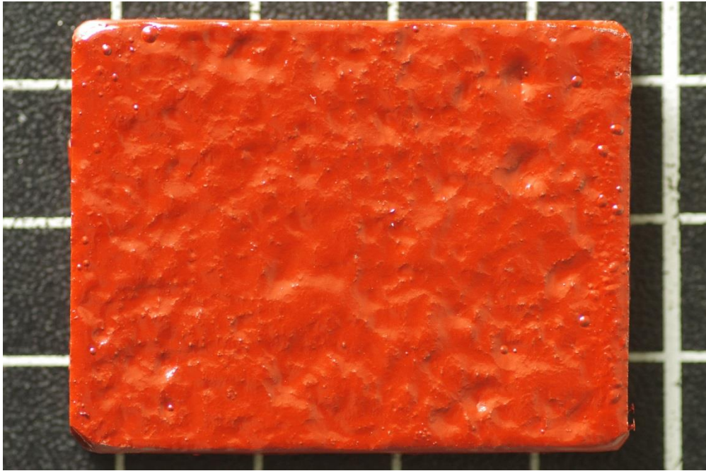
Figure 5.35 Sample HSII08 showing bubbles in System A primer after curing (scale of background squares 10 x 10mm).
