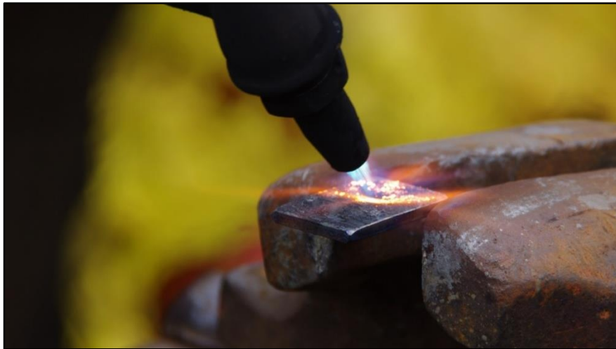
Figure 6.4 Luminescence of coating and oxide vestiges under flame (practitioner PB).
