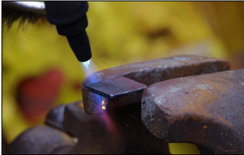
Figure 6.3 Position of the flame relative to the sample during flame cleaning by practitioner PB.
