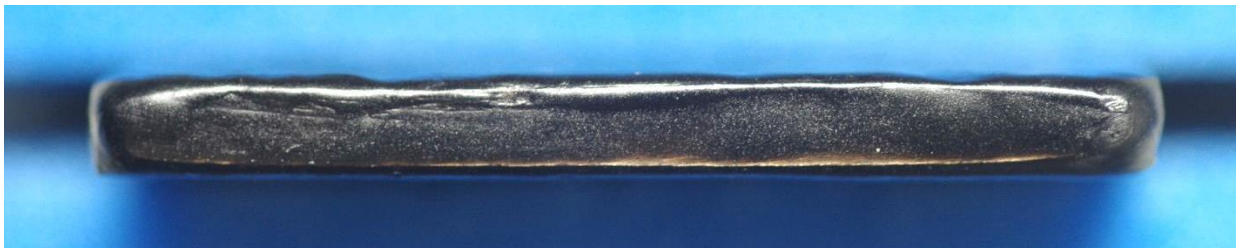
Figure 5.44 Sample HSII28 showing run back of cured Coating C from edges (sample area shown 40mmx4mm).
