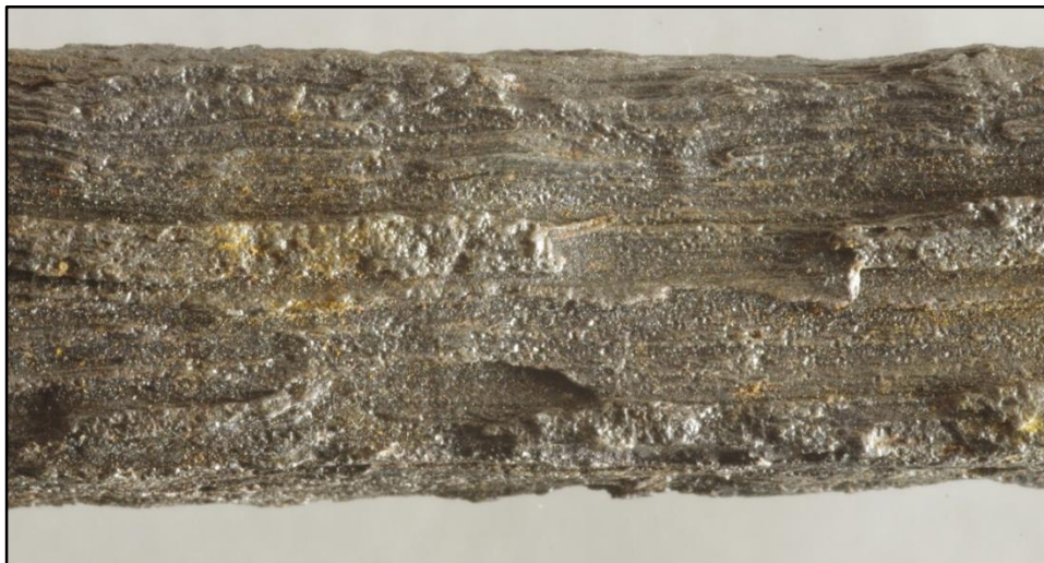
Figure 2.9 Lamellar corrosion of early wrought iron railway wedge.
