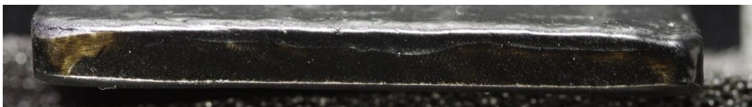
Figure 5.63 Sample HSII26 after exposure to 90%RH for 540 days showing no visible corrosion even where coating build is very low on edges (sample area shown 40mm x 4mm).
