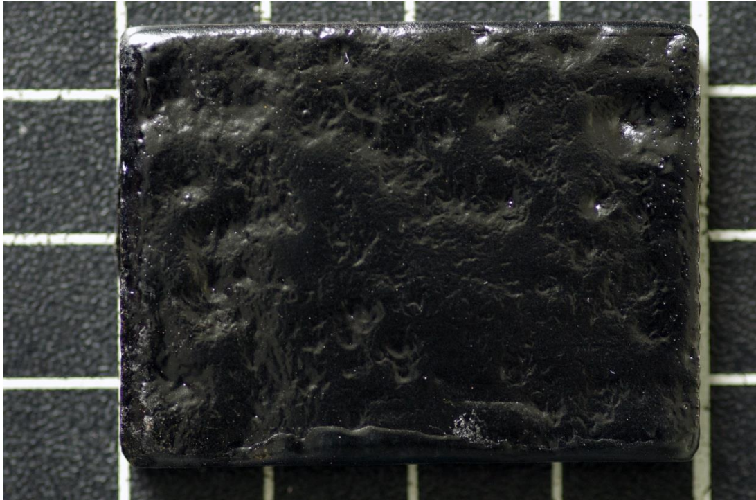
Figure 5.43 Sample HSII26 showing pinholes in Coating C after curing (scale of background squares 10 x 10mm).
