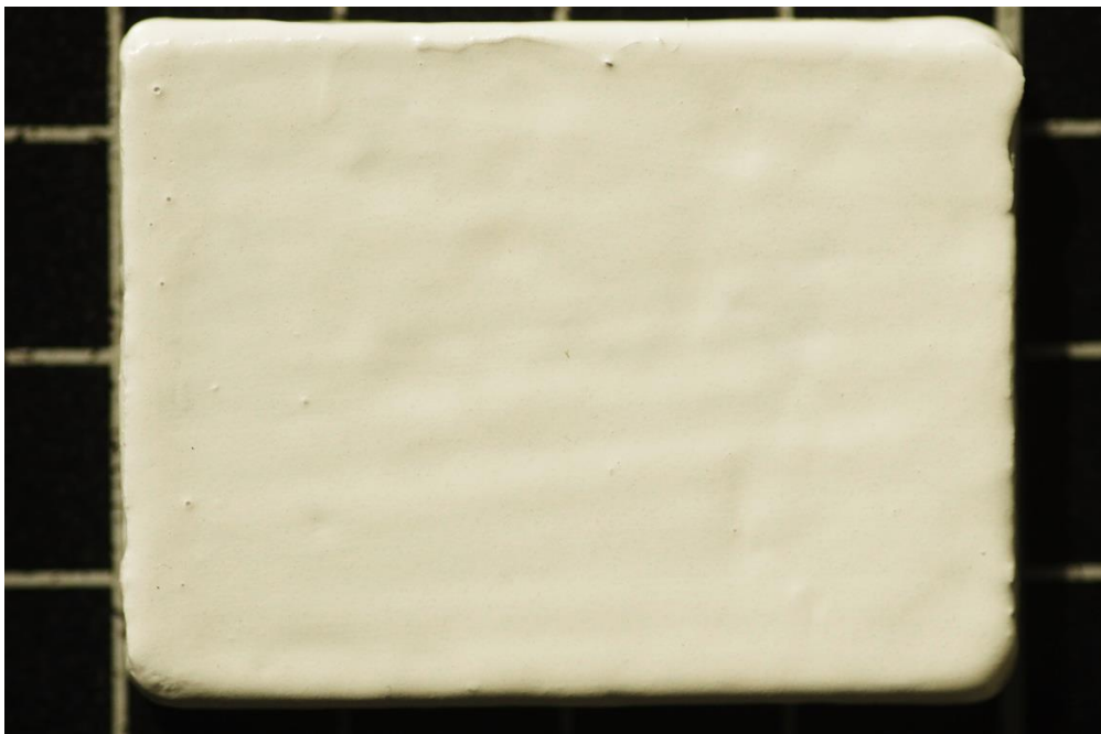
Figure 5.36 Sample HSII04 showing pinhole holidays in cured System A build coating (scale of background squares 10 x 10mm).
