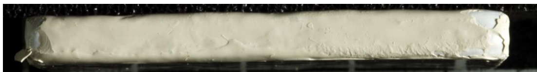
Figure 5.60 Sample HSII02 showing damage to topcoat of System A after 90%RH exposure (scale of background scale 10mm between white lines).
