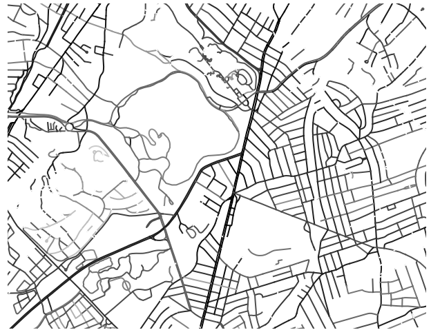
Figure 5: The linearity feature of each street segment in Figure 4 is represented by a grayscale map where black corresponds to a value of one while colours approaching white correspond to a value of zero.
