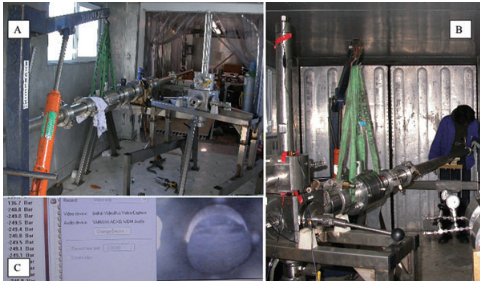
Fig. 2. Photograph of (A) the PRESS core cutting and manipulation system, with the DeepIsoBUG core slicer separate.
