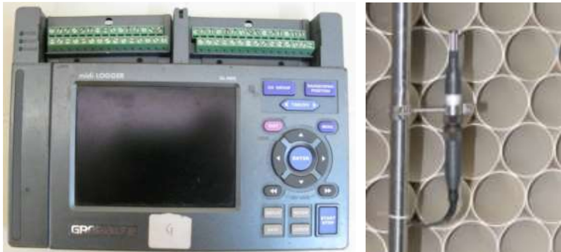
Figure 50 GL450 midi LOGGER (Left) Temperature / RH sensor (Right)
