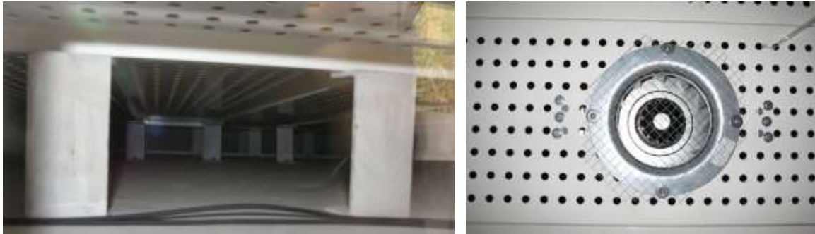
Figure 42 Lower section of the testing chamber (Left) Centrifugal fan at the perforated panels (Right)
