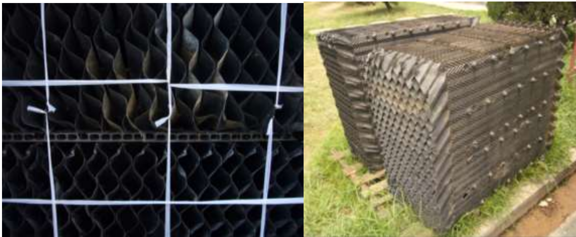
Figure 22 Front view of the fill (Left) and a pack of cooling tower fill (Right)
