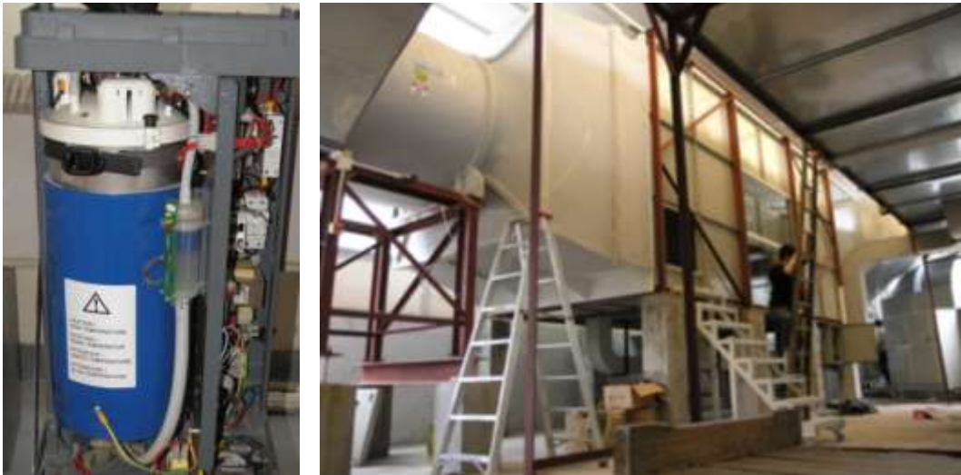
Figure 37 Water boiler that controls the moisture content of the discharge air inlet (Left) testing chamber for scaled cooling tower visible plume test (Right)
