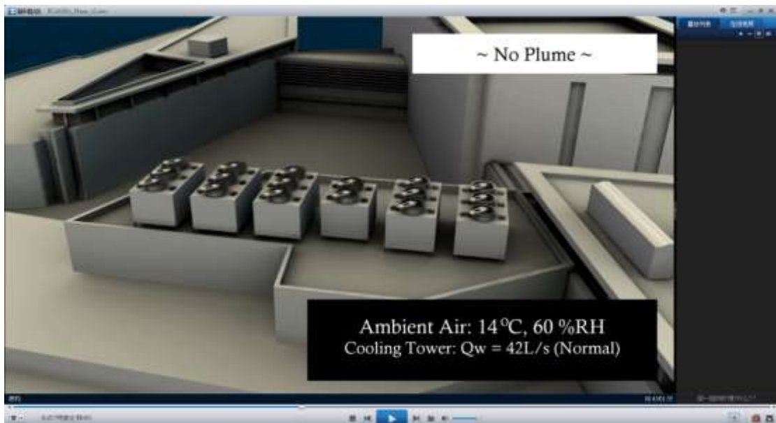
Figure 115 Transient graphical results of flow pattern of cooling tower discharge
