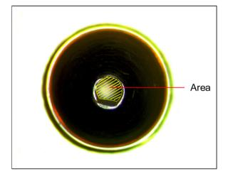
Fig. 2. A representative image to illustrate the area of capsule puncture that was recorded and quantified using ImageJ software.
