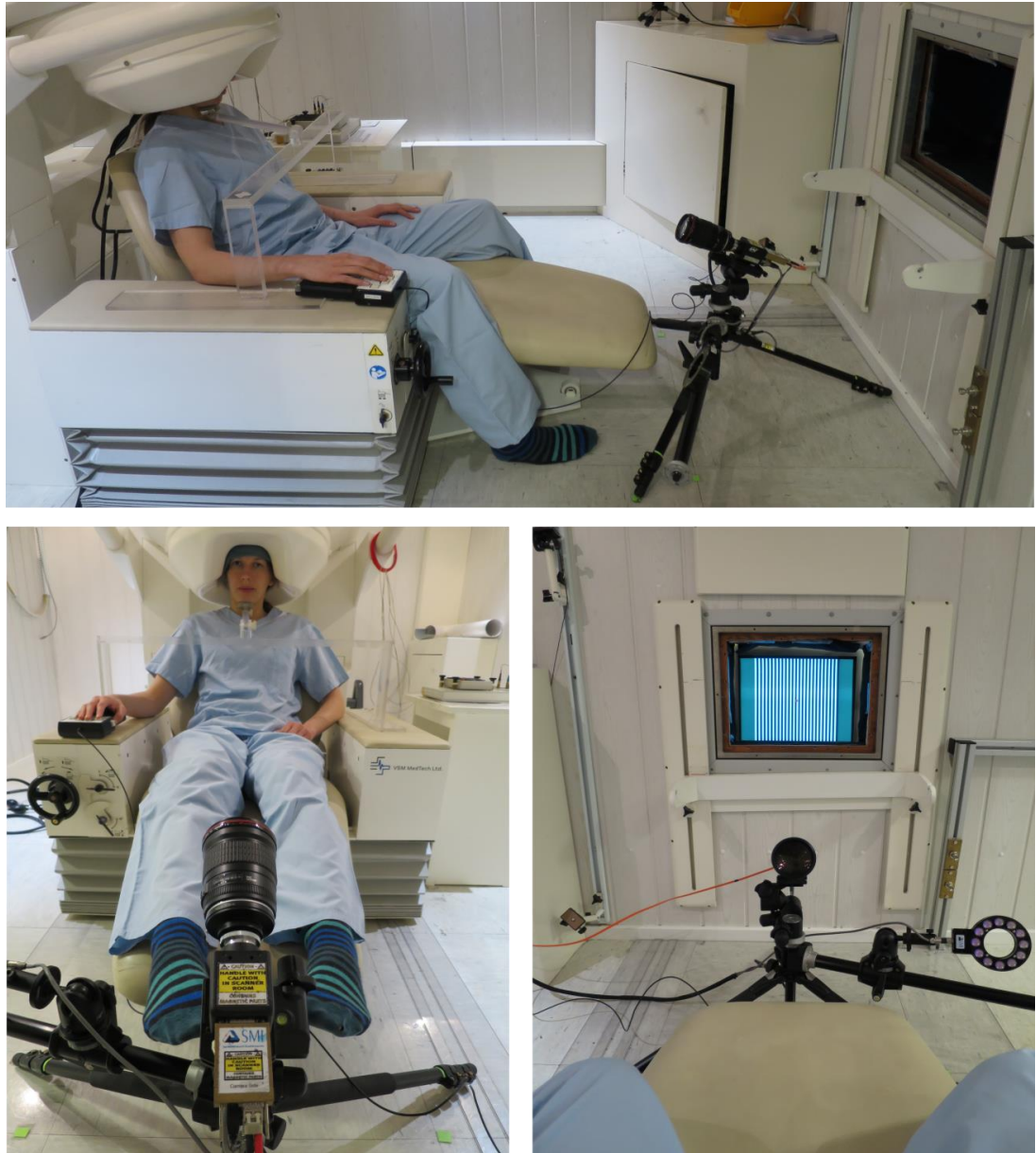
Figure 2-3. Experimental setup for simultaneous MEG and eye tracking. Top , an overview of the MEG magnetically shielded room with the eye tracker placed between the participant and the monitor display. Bottom left , view of the eye tracker and the participant from the monitor's perspective. Bottom right , view of the eye tracker and the monitor from the participant's perspective. The infrared illumination unit is placed to the right of the eye tracker camera.
