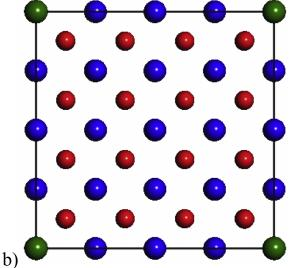
FIG. 2. a)  $Th_7U_1O_{16}$  b) a  $Th_{31}U_1O_{64}$  supercells.
