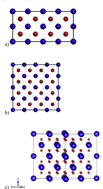
FIG. 1. a) 1x1x2 supercell, b) and c) 2x2x2 supercell face and side views of  $ThO_2$ , where the Th atoms are represented by the blue spheres and the O atoms are represented by the red spheres.
