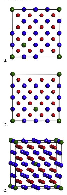
FIG. 8.  $Th_{30}U_{2}O_{64}$  where Th is represented in blue, U in green, and O in red. a. Configuration 4 (38% probability); b. Configuration 5 (41% probability); c. Lowest probability structure.
