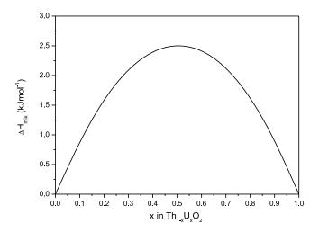
FIG. 10.  $\Delta H_{mix}$  calculated using a 1x1x2 supercell.
