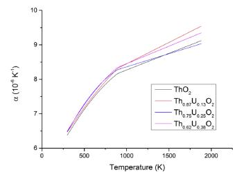
FIG. 14. Coefficient of thermal expansion of  $Th_{(1-x)}U_xO_2$  solid solutions.
