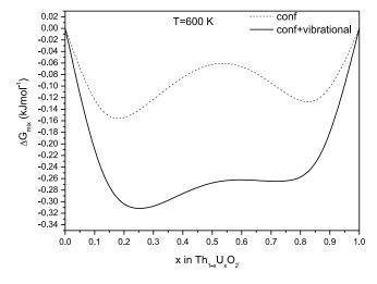
FIG. 12.  $\Delta G_{mix}$  at 600 K showing the configurational and the configurational and vibrational effects.
