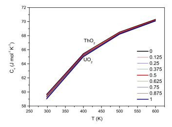
FIG. 13. Constant volume heat capacity of  $Th_{(1-x)}U_xO_2$  solid solutions.
