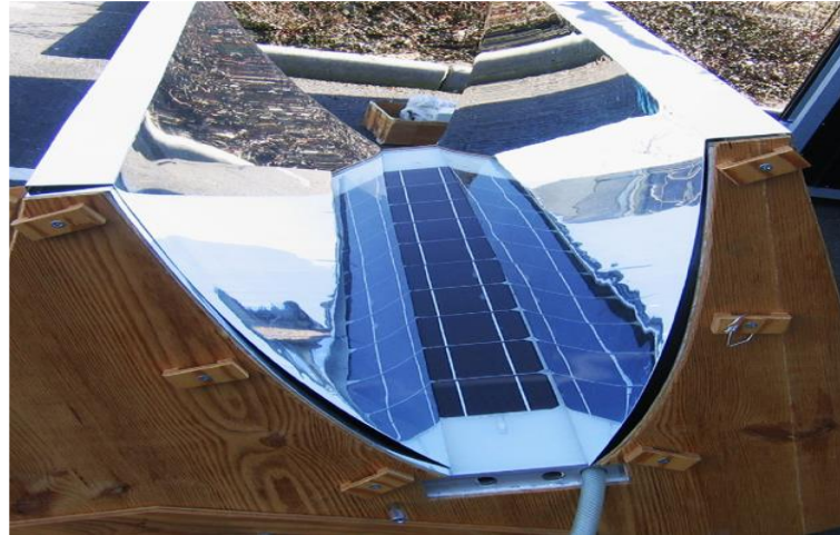
Figure 2. 17 The truncated compound parabolic concentrator showing removable reflectors and a 10-cell module string [73]
