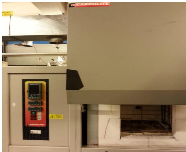
Figure 6. 5 Furnace used for the working electrode
