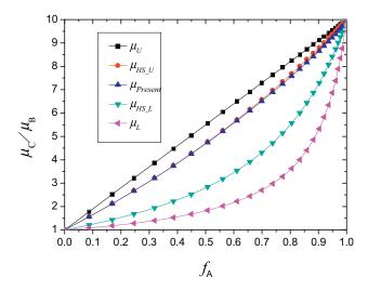
Fig. 3. Effects of  $f_A$  on the effective conductivity of type-I composite materials with  $\mu_A/\mu_B=10.$
