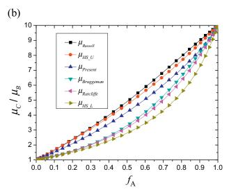
Fig. 5. Effects of  $f_A$  on the effective conductivity of type-II composite materials with  $\mu_A/\mu_B=10$ . (a) Comparison with classical bounds; (b) comparison with some theoretical models.
