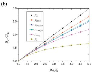
Fig. 4. Effects of  $\mu_A/\mu_B$  on the effective conductivity of type-II composite materials: (a)  $f_A=0.104$ ; (b)  $f_A=0.5$ .
