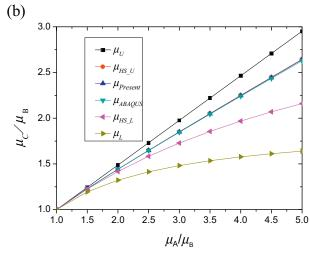
Fig. 2. Effects of  $\mu_A/\mu_B$  on the effective conductivity of type-I composite materials: (a)  $f_A=0.271$ ; (b)  $f_A=0.488$ .
