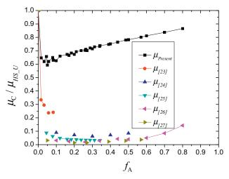
Fig. 6. Comparison between the experimentally measured results<sup>[23–27]</sup> and our prediction for the type-II composites. Results are normalized by the Hashin and Shtrikman's upper bound.
