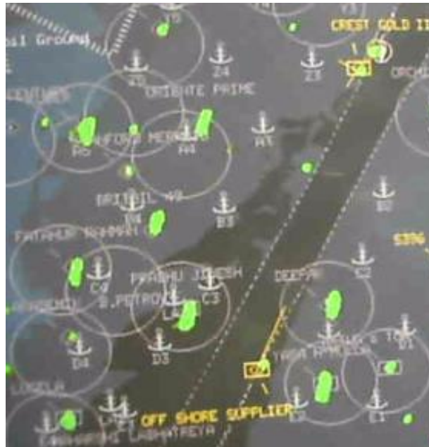
Figure 4. 5: Stationary vessels in grey colour, marked by grey circles; anchored on either side of the main channel
