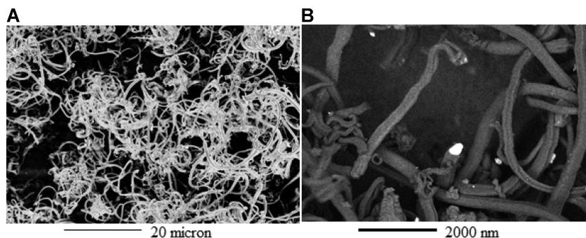
**Figure 9.** TEM analysis of spent 1% Au/C catalyst prepared using aqua regia after use for 24 days. (A) Low magnification showing the extent of carbon nanofibers formed on the catalyst. (B) Higher magnification showing the gold nanoparticle at the tip of the carbon nanofiber.
