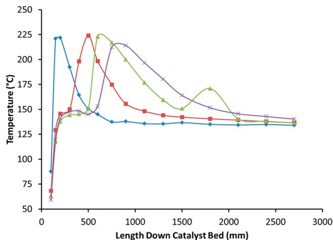
**Figure 13.** Temperature profile down catalyst bed of full scale commercial reactor at different VCM yields showing the migration of the exotherm region down the catalyst bed at different catalyst productivities. Catalyst = 0.1%  $\text{Au}/\text{C}$  prepared by supporting  $\text{Na}_3\text{Au}(\text{S}_2\text{O}_3)_2$  on carbon extrudates. Blue = ca. 10 kg VCM/kg cat; red = ca. 500 kg VCM/kg cat; green = ca. 600 kg VCM/kg cat; purple = ca. 1000 kg VCM/kg cat.
