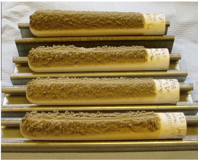
Fig. 7. Impact of the blend composition on the slagging tendency (5% miscanthus in the foreground rising to 25% in the background).
