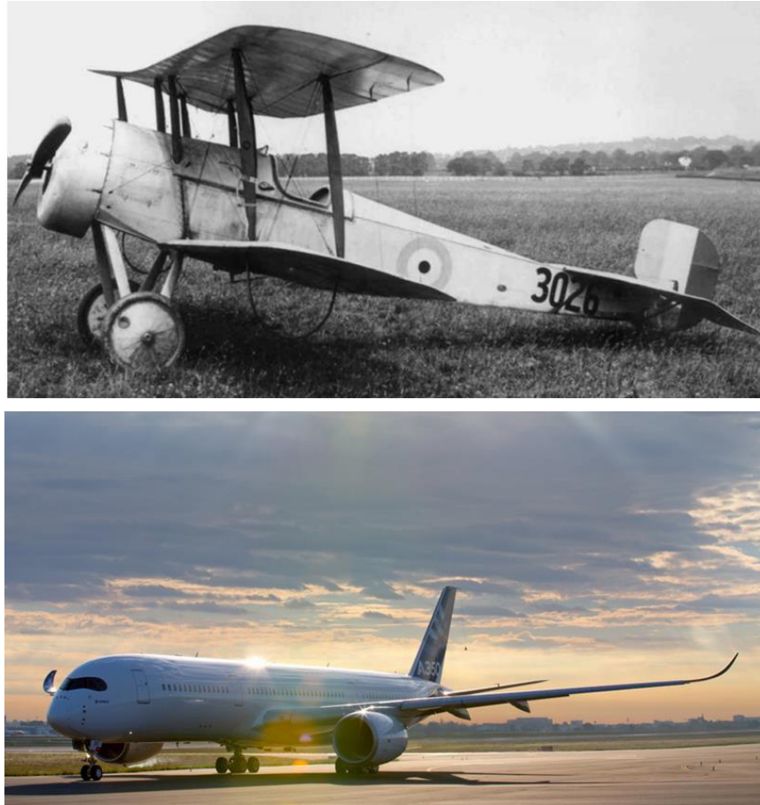
Figure 2.1: Aircraft from the early stages of the 20 th and 21 st Centuries. Top: World War I Bristol Scout predominantly made from wood and fabric with wire bracing, figure reproduced from Jakab (1999); bottom: Airbus A350 XWB predominantly made from aluminium and advanced composites, figure reproduced from Avioners (2014)
