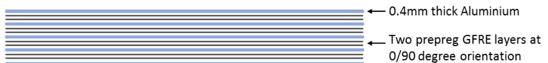
Figure 4.2: schematic representation of GLARE layup
