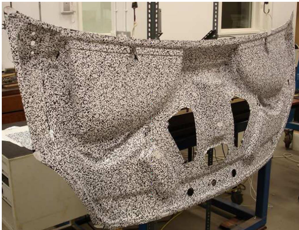
Figure 3.19: Example of DIC speckle pattern from a study on a car bonnet, figure reproduced from Wang et al (2012)
