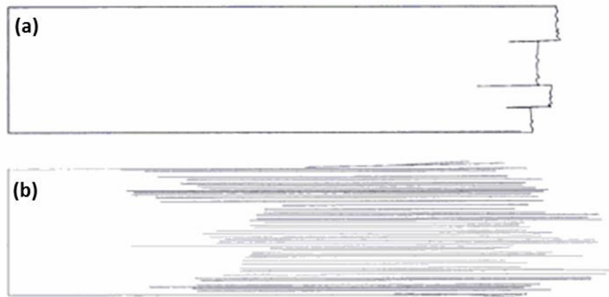
Figure 2.5: Example of the appearance of carbon fibre coupon specimens which have failed as a result of (a) brittle fibre fracture under large single loading (b) fibre fracture by fatigue, figures reproduced from Harris (2003)
