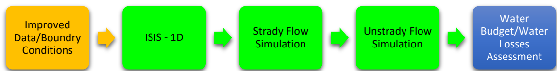
Figure 4.6 Procedure for developing the required information for the water budget/water losses assessment using a hydrodynamic model.
