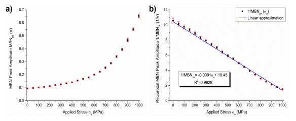
Fig. 4.17 a) MBN peak amplitude as a function of applied stress for SAE9310 TS2 sample; b) Dependence of reciprocal MBN peak amplitude on applied stress approximated with linear function. Red bars reflect the standard deviation from the mean data values.
