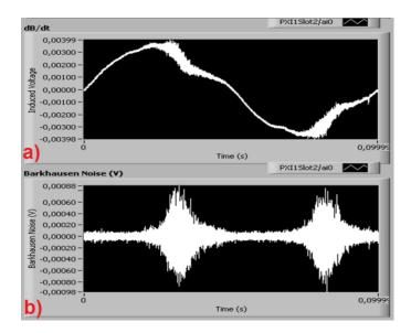
Fig. 3.35 a) Original voltage data obtained from the output of Barkhausen sensor; b) High-pass filtered Barkhausen signal.
