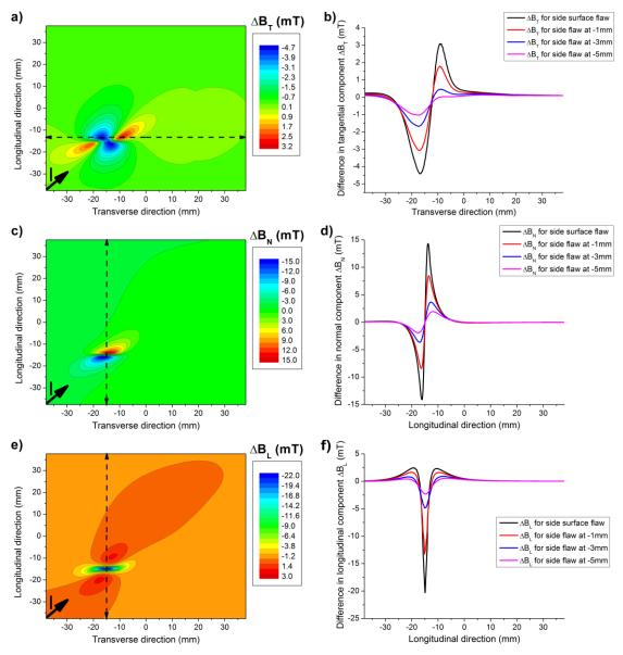
Fig. 5.39 Differential distributions of: a) tangential component; c) normal component and e) longitudinal component of magnetic field above surface side-flawed rail energised diagonally. Numerical profiles of differential perturbations in b) tangential component; d) normal component and f) longitudinal component of magnetic field probed above diagonally energised rails with surface and sub-surface flaws.
