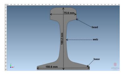
Fig. 5.10 Cross-section of analysed rail with indicated sub-sections and main dimensions.
