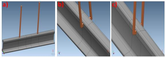
Fig. 5.12 Illustrations of modelled beryllium-copper electrodes applying current: a) in longitudinal direction; b) in transverse direction; c) at 45°to longitudinal and transverse planes of rail.
