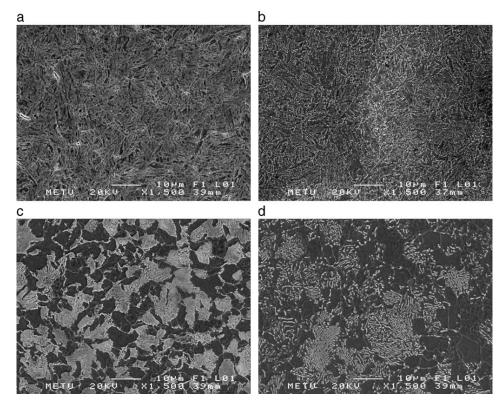
Fig. 3.44 SAE 1040 steel microstructures studied with Magnetic Barkhausen Noise: a) as-quenched martensite; b) tempered martensite; c) fine pearlite-ferrite, d) coarse pearlite-ferrite [90].
