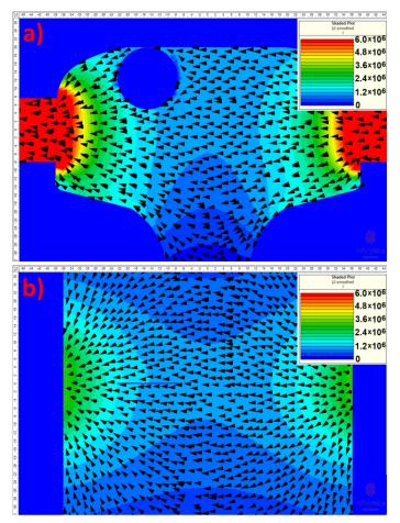
Fig. 5.30 Distributions of current density **J** within a) transverse cross-section and b) longitudinal crosssection of tangentially energised rail with side transverse flaw.
