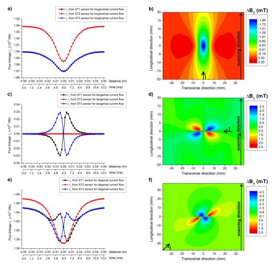
Fig. 5.51 Flux linkage signals from tangential sensors ST1, ST2 and ST3 probed above rails with surface centre flaws energised: a) longitudinally, c) tangentially and e) diagonally. Corresponding distributions of effective changes in tangential component  $\Delta B_T$  obtained above rails with surface centre flaws energised: b) longitudinally, d) tangentially and f) diagonally.
