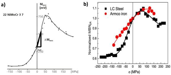
Fig. 3.52 Non-monotonic variation of MBN peak amplitude with applied stress for a) 22NiMoCr 37 pressure vessel steel; b) low carbon steel and Armco iron [100, 101].
