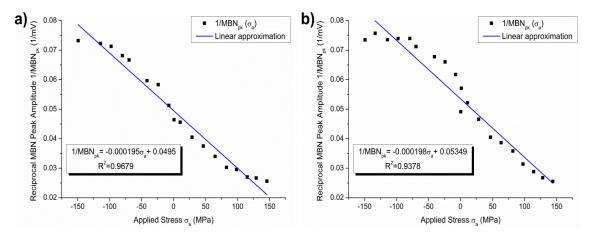
Fig. 4.32 a) & b) Linear approximations of the relations between the reciprocal MBN peak amplitude with ascending and descending stresses applied to pipeline steel sample. Based on the results of Jagadish et al [121].
