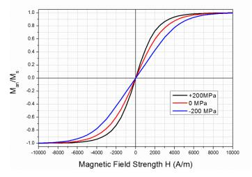
Fig. 2.11 Anhysteretic magnetisation curves for ferromagnetic material with positive magnetostriction at zero stress and under applied stresses of -/+200MPa.
