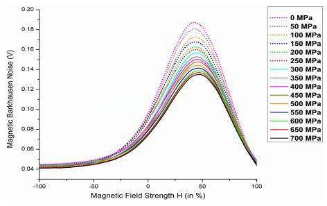
Fig. 4.21 Magnetic Barkhausen Noise signal envelopes obtained for TS2 sample under various applied tensile stress.
