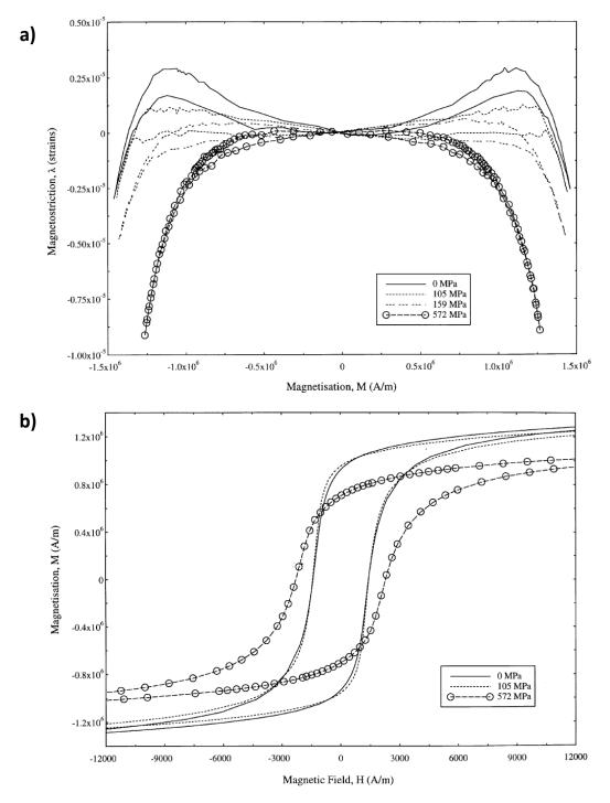
Fig. 3.31 a) Magnetostriction loops for 0.86%C steel subjected to various tensile stresses; b) Hysteresis loops for 0.86%C steel under different tensile loads [69].
