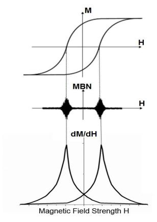
Fig. 2.19 Relation between the magnitude of Barkhausen Noise and magnetisation dynamics [21].
