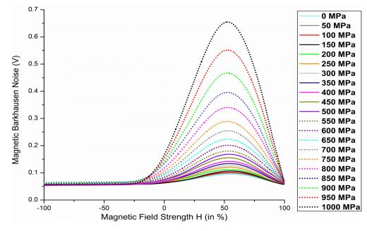
Fig. 4.16 Magnetic Barkhausen Noise signal envelopes obtained for TS2 sample under various applied tensile stress.
