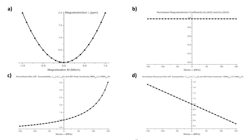
Fig. 4.1 a) Parabolic approximation of hysteresis-free magnetostriction curve with  $b=2\times10^{-18}$ ; b) Normalised magnetostriction coefficients b and b' invariant with stress; c) Normalised maximum differential susceptibility  $\chi'_{Hc}$  and MBN peak amplitude MBN<sub>pk</sub> as functions of stress; d) Dependence of normalised reciprocal maximum differential susceptibility  $1/\chi'_{Hc}$  and reciprocal MBN peak amplitude  $1/MBN_{pk}$  on stress approximated with linear function.
