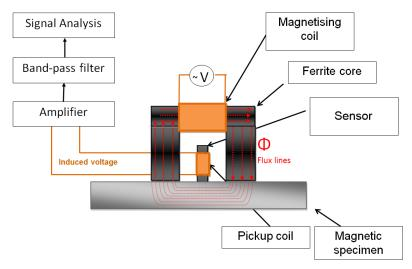
Fig. 3.34 Schematic diagram of typical Barkhausen Noise measurement set-up.
