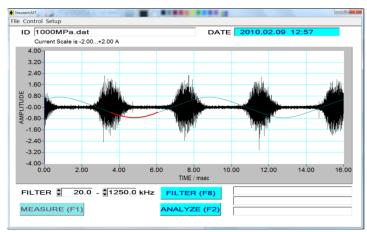
Fig. 4.8 Illustration of Barkhausen voltage bursts acquired with Microscan 600.
