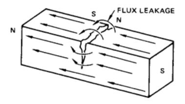
Fig. 3.20 Illustration of magnetic flux leakage in the vicinity of defect in ferromagnetic material.
