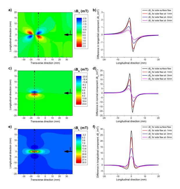
Fig. 5.31 Differential distributions of: a) tangential component; c) normal component and e) longitudinal component of magnetic field above surface side-flawed rail energised in tangential direction. Numerical profiles of differential perturbations in b) tangential component; d) normal component and f) longitudinal component of magnetic field probed above tangentially energised rails with surface and sub-surface flaws.
