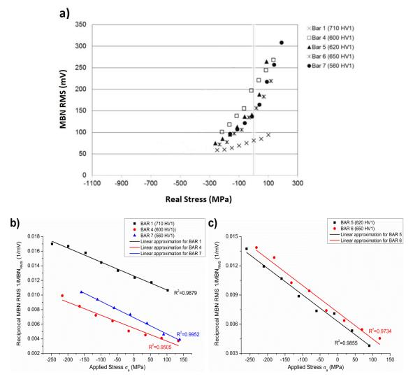
Fig. 4.40 a) a) MBN root-mean-square amplitude as a function of stress applied to EN10084 samples of various surface hardness; b) & c) Dependencies of reciprocal MBN root-mean-square on applied stress for EN10084 samples approximated with linear functions, after Santa-aho [123].
