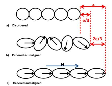
Fig 2.6 Schematic diagram illustrating the magnetostriction in: a) disordered paramagnetic state, b) demagnetised ferromagnetic state, c) ferromagnetic state magnetised to saturation (image reproduced from [5]).
