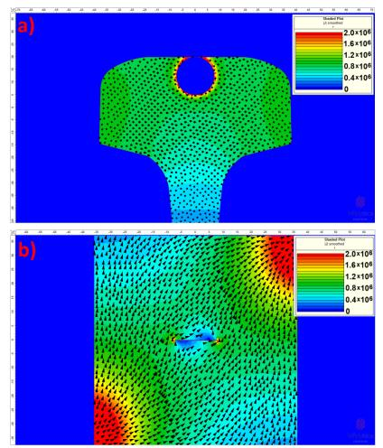
Fig. 5.34 Distributions of current density **J** within a) transverse cross-section and b) longitudinal crosssection of diagonally energised rail with centre transverse flaw.
