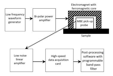
Fig. 4.44 Schematic diagram of MBN set-up for depth profiling analysis.
