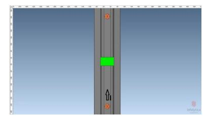
Fig. 5.16 Top view on analysed rail with indicated area (green) within which the magnetic field distributions for unflawed and flawed cases were studied.
