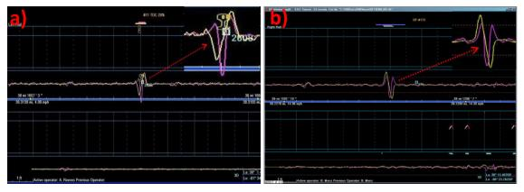
Fig. 5.7 Typical induced voltage signatures indicating the presence of transverse flaw probed with: a) longitudinal sensor SL (purple curve) and normal sensor SN (yellow curve); b) longitudinal sensor SL (purple curve) and tangential sensor ST (yellow curve).
