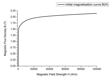
Fig. 5.41 Initial magnetisation curve of M800-65A sensor steel.
