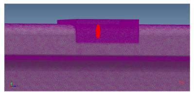
Fig. 5.14 Illustration of very fine mesh of air box encompassing the region above a flawed rail volume.
