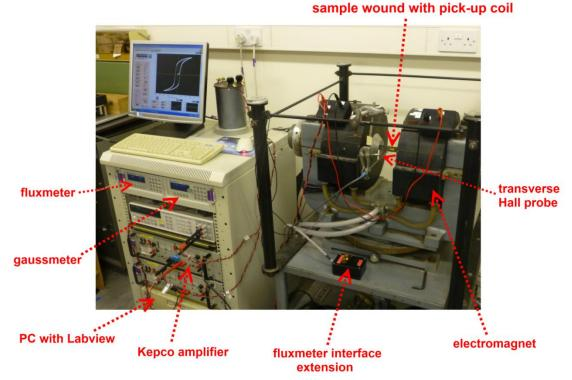
Fig. 4.4 Image of the DC hysteresis loop measurement set-up.
