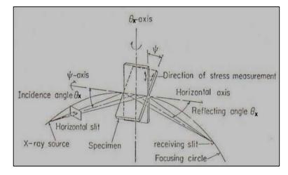
Fig. 3.18 Schematic diagram of residual stress measurement set-up using the  $\sin^2 \psi$  x-ray diffraction technique [49].
