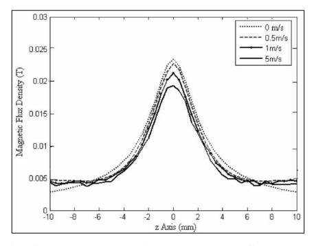
Fig. 3.25 Profiles of the tangential component of MFL density obtained at different inspection velocities for case of cuboid flaw in steel tube [61].
