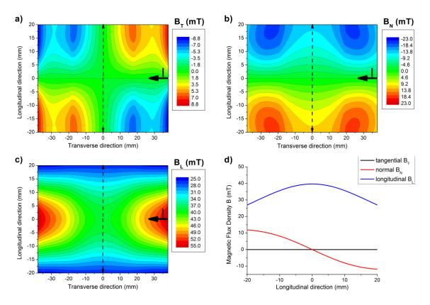
Fig. 5.25 Distributions of a) tangential component; b) normal component and c) longitudinal component of magnetic field at 1mm above central section of tangentially energised unflawed rail; d) Numerical profiles of these magnetic field components probed in the regions indicated by the arrows.
