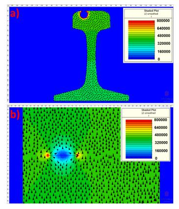
Fig. 5.22 Distributions of current density **J** within a) transverse cross-section and b) longitudinal crosssection of side-flawed rail energised longitudinally.
