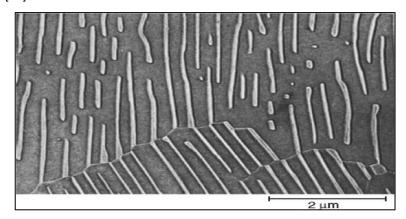
Fig. 3.40 Cementite (dark regions) and ferrite in the form of lamellar microstructure called pearlite [88].
