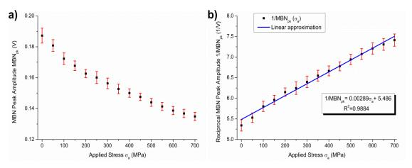
Fig. 4.22 a) MBN peak amplitude as a function of applied stress for SAE6481 TS1 sample; b) Dependence of reciprocal MBN peak amplitude on applied stress approximated with linear function. Red bars reflect the standard deviation from the mean data values.
