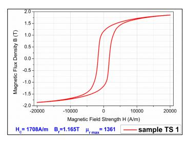
Fig. 4.13 DC hysteresis loop of nitrided SAE6481 sample.
