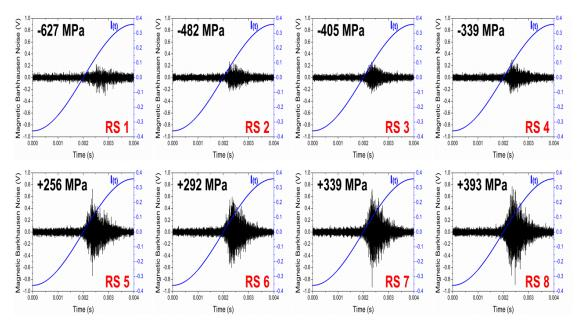
Fig. 4.25 Barkhausen voltage bursts acquired for SAE9310 RS samples with various levels of surface residual stress.
