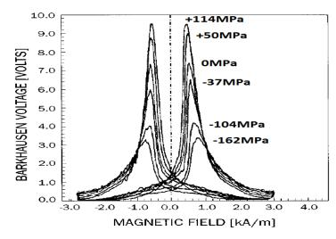
Fig. 3.50 MBN envelopes for XC10 steel subjected to different amplitudes of applied stress [65].
