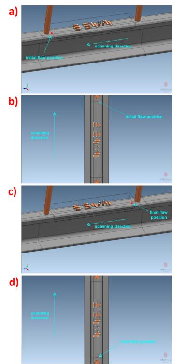
Fig. 5.43 Top and side views on FEM model used to simulate the dynamic flaw inspection with Sperry Induction Sensing Unit.
