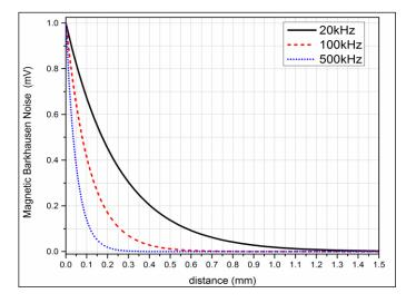
Fig. 4.42 Attenuation curves for MBN signals with frequencies of 20kHz, 100kHz and 500kHz propagating within hypothetical ferromagnetic material.
