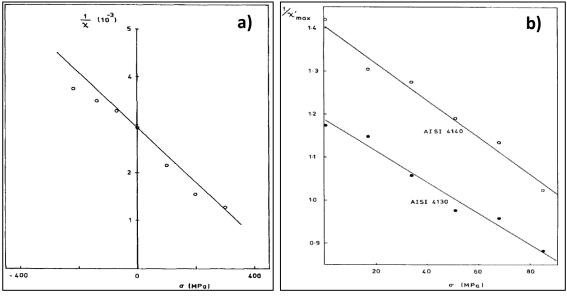
Fig. 3.32 Modelled linear approximation of: a) Reciprocal differential anhysteretic susceptibility at origin as function of stress in AISI 4130 steel; b) Variation of maximum reciprocal differential susceptibility of AISI 4130 and 4140 steels with stress [12, 71].
