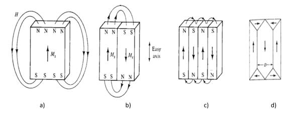
Fig. 2.3 Division of ferromagnetic crystal into domains. Only external H fields are shown [1].
