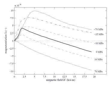
Fig. 3.48 Anhysteretic magnetostriction of iron obtained under different tensile and compressive stresses [92].
