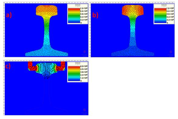
Fig. 5.49 Distribution of current density J in transverse cross-section of rails energised: a) longitudinally;b) diagonally and c) tangentially.
