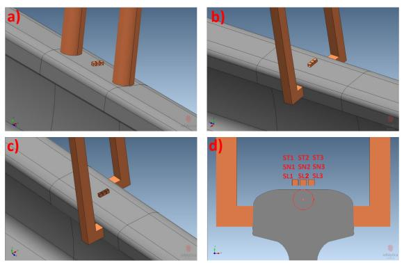
Fig. 5.48 Illustrations of modelled types of beryllium-copper electrodes for applying current in: a) longitudinal direction, b) tangential direction and c) at 45° to longitudinal and transverse planes of rail;d) Transverse view of the model with indicated positions of directional sensors.
