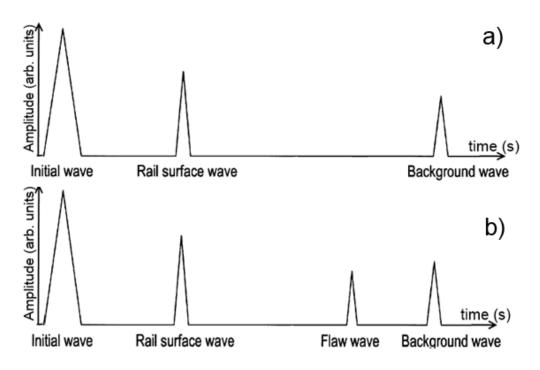
Fig. 3.11 The schematic pulse echo-diagram of signal intensity vs time for a) unflawed rail; b) rail with internal flaw generating an additional intermediate reflection echo.
