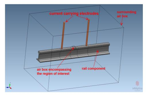
Fig. 5.8 FEM solid model used for static field analysis of energised flawed and unflawed rails.
