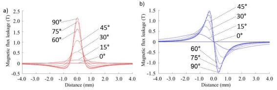
Fig. 3.27 Dependence of a) tangential and b) normal components of magnetic flux leakage on the angle between flaw and magnetic field direction [63].
