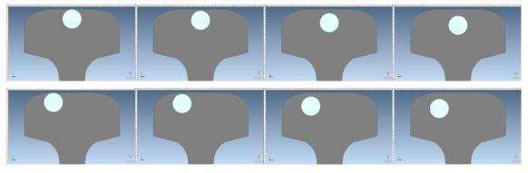
Fig. 5.13 Illustrations of analysed flaw positions within rail's cross-section.
