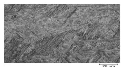
Fig. 3.41 Typical lath martensitic microstructure present in quenched steels with carbon content less than 0.6% [88].
