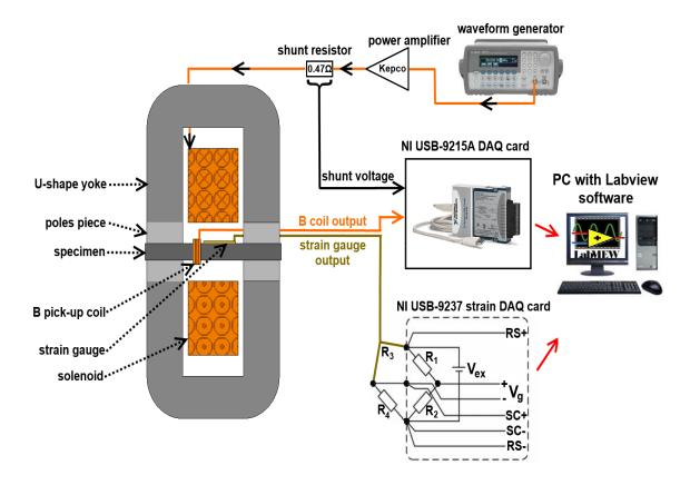
Fig. 4.5 Schematic diagram of the AC magnetostriction measurement set-up.
