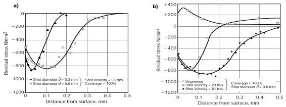
Fig. 3.6 Influence of shot-peening parameters on residual stress depth distributions: a) shot diameter, b) shot velocity [35].
