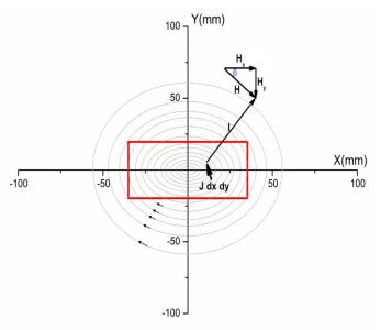
Fig 5.1 Schematic diagram of rectangular current carrying conductor and corresponding circulating magnetic field.
