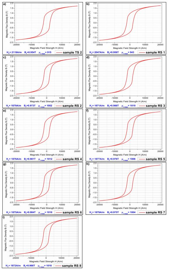
Fig. 4.11 DC hysteresis loops obtained for carburised SAE9310 samples.
