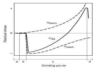
Fig. 3.5 Contributions of the thermal and mechanical components to the effective residual stress after grinding [35]
