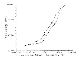
Fig. 4.31 Peak-to-peak amplitude of surface Barkhausen Noise (SBN) obtained by Jagadish for pipeline steel sample under various applied stress [121].
