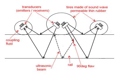
Fig. 3.13 Schematic diagram of the ultrasonic beam reflection from the 90° transverse rail flaw.
