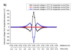
Fig. 5.52 Induced voltage signals from tangential sensors ST1, ST2 and ST3 probed above rails with surface centre flaws energised: a) longitudinally, c) tangentially and e) diagonally at speed rate of 30km/h.
