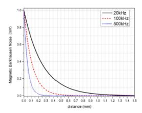
Fig. 1. Attenuation curves for MBN signals with frequencies of 20, 100, and 500 kHz propagating within ferromagnetic material.
