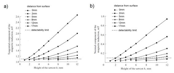
Fig. 3.26 Dependence of a) tangential and b) normal components of magnetic flux leakage on the height of flaw and its distance from rail surface [62].
