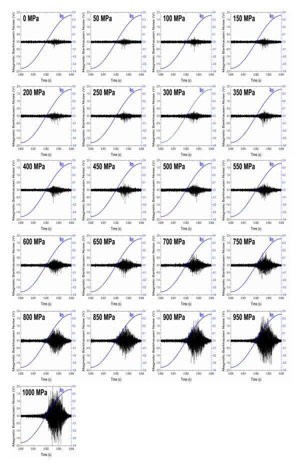
Fig. 4.15 Barkhausen voltage bursts acquired for SAE9310 TS2 sample under various applied tension.
