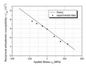
Fig. 5. Reciprocal of MBN peak amplitude for carburized SAE 9310 specimen as a function of applied stress. Compare with Fig. 4.
