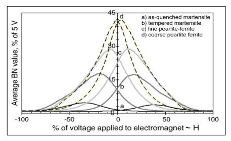
Fig. 3.43 MBN smoothed envelopes obtained for different SAE 1040 steel microstructures [90].
