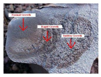
Fig. 3.9 Illustration of the subsequent growth stages of transverse rail defect [38].
