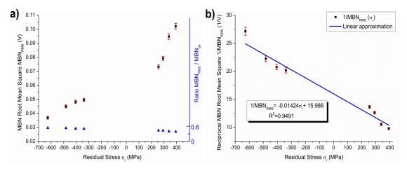
Fig. 4.28 a) MBN root-mean-square amplitude as a function of residual stress of SAE9310 RS samples;b) Dependence of reciprocal MBN root-mean-square on residual stress approximated with linear function. Red bars reflect the standard deviation from the mean data values.
