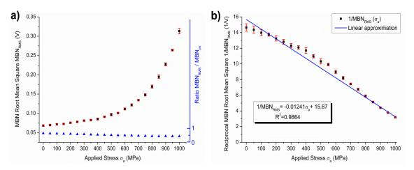
Fig. 4.18 a) MBN root-mean-square amplitude as a function of applied stress for SAE9310 TS2 sample;b) Dependence of reciprocal MBN root-mean-square on applied stress approximated with linear function. Red bars reflect the standard deviation from the mean data values.
