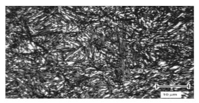
Fig. 3.42 Microstructure of water-quenched AISI 1080 steel showing plate martensite (dark regions) in combination with retained austenite (light regions) [88].
