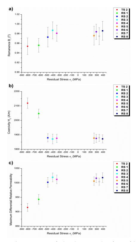
Fig. 4.12 Main DC hysteresis parameters of carburised SAE9310 samples as function of their surface residual stress.
