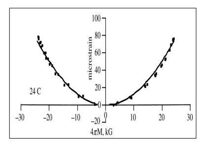
Fig. 2.13 Magnetostriction as function of magnetisation with parabolic approximation in polycrystalline iron cobalt (FeCo+2%V) [14].
