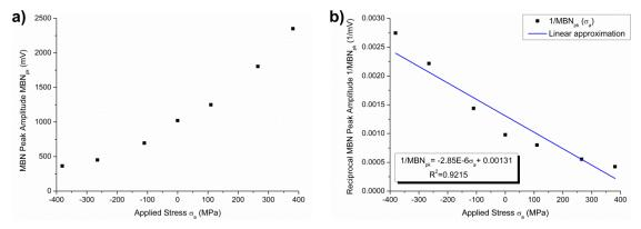
Fig. 4.35 a) MBN peak amplitude as a function of applied stress for EN36 sample with 0.65mm casedepth [91]; b) Dependence of reciprocal MBN peak amplitude on applied stress approximated with linear function.
