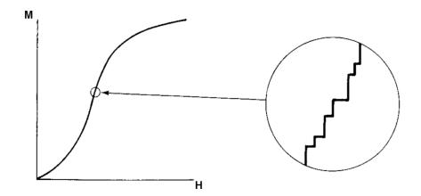
Fig. 2.14 Illustration of discontinuous changes in magnetisation obtained by magnifying a portion of magnetisation curve by factor of  $10^9$  [1].
