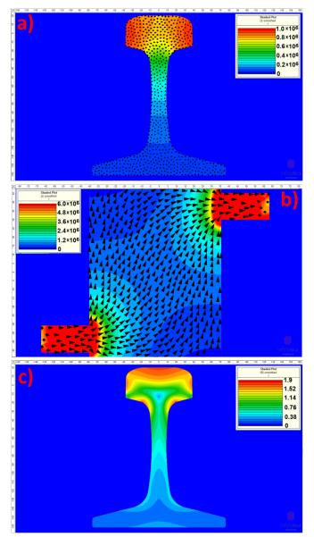
Fig. 5.32 Distributions of current density **J** within a) transverse cross-section and b) longitudinal crosssection of diagonally energised rail; c) Distribution of flux density **B** within transverse cross-section of diagonally energised rail.
