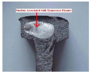
Fig. 3.8 Illustration of transverse defect which nucleated around steel imperfection in rail cross-section [38].
