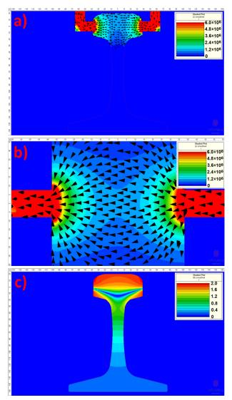
Fig. 5.24 Distributions of current density **J** within a) transverse cross-section and b) longitudinal crosssection of tangentially energised rail; c) Distribution of flux density **B** within transverse cross-section of tangentially energised rail.
