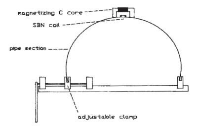
Fig. 4.30 MBN measurement set-up used in work of Jagadish et al [121].
