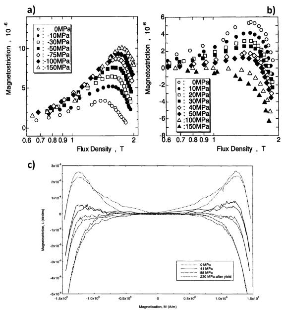
Fig. 4.2 a) & b) Effects of compressive and tensile stresses on magnetostriction curves in JIS-SS400 low carbon steel; c) Influence of tensile stress on magnetostriction butterfly loops in 50D pearlitic steel [69, 111].
