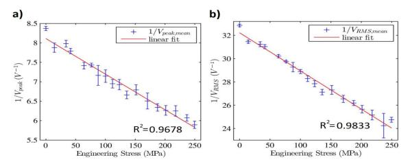
Fig. 4.41 a) & b) Linear approximations of stress dependencies of the reciprocal MBN peak amplitude and reciprocal MBN root-mean-square of ASTM A36 steel, after Kypris [125].
