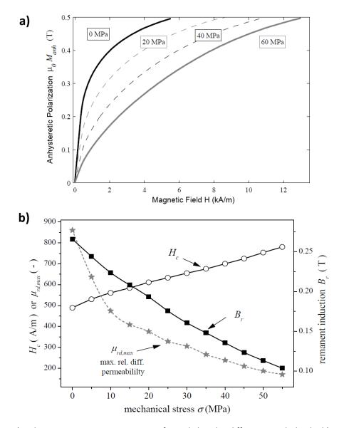
Fig. 3.29 a) Anhysteretic magnetisation curves for nickel under different tensile loads; b) Variation of hysteretic parameters of nickel with tensile stress [70].
