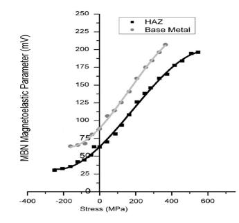
Fig. 3.53 MBN root-mean-square as function of applied stress for API 5L X70 steel before (base metal) and after welding process (HAZ – heat affected zone) [103].
