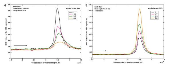
Fig. 4.36 MBN envelopes obtained by Moorthy for the EN36 specimen with carburised case-depth of 0.95mm subjected to various applied stress [91].
