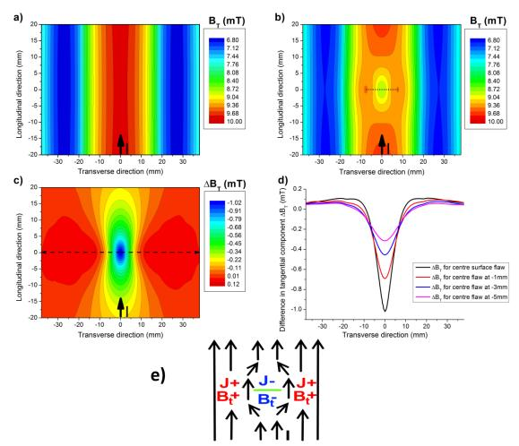
flawed case was subtracted from the corresponding matrix for unflawed case providing a differential distribution  $\Delta B_T$  caused by the flaw, as depicted in Fig. 5.19c.
