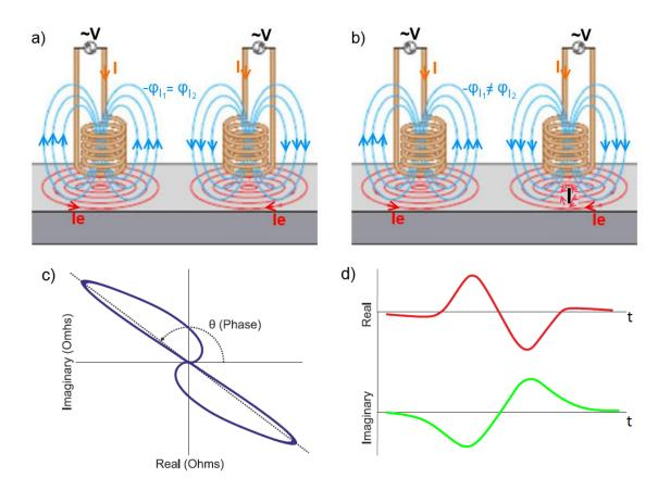
Fig. 3.14 Schematic diagram of EC differential probe positioned above a) unflawed material; b) flawed material with depicted distortion in eddy current flow. A typical output signal from EC differential probe indicating the presence of flaw plotted as c) loop on complex impedance plane; d) real and imaginary parts of impedance vs time [46].
