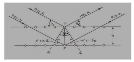
Fig. 3.17 Diffraction of X-rays by a crystal lattice satisfying the Bragg's law [49].
