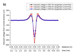
Fig. 5.54 Induced voltage signals from normal sensors SN1, SN2 and SN3 probed above rails with surface centre flaws energised: a) longitudinally, c) tangentially and e) diagonally at speed rate of 30km/h.
