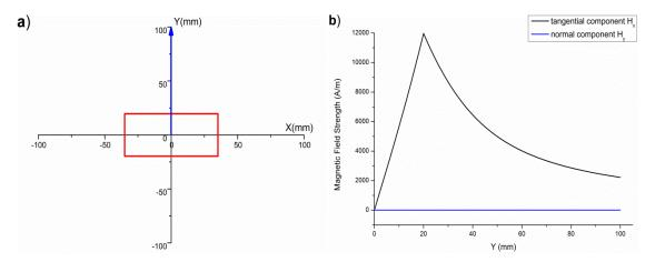
Fig. 5.3 a) Indication of the region in which the profiles of  $H_x$  and  $H_y$  were simulated; b) Values of  $H_x$  and  $H_y$  along the normal direction from centre of the rail head.
