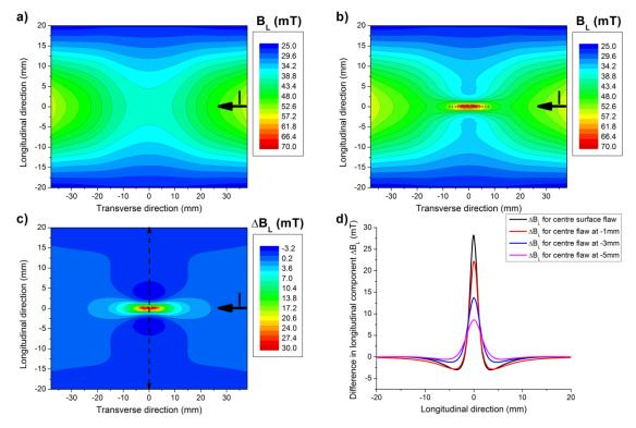
Fig. 5.29 Distributions of longitudinal component of magnetic field at 1mm above tangentially energised: a) unflawed rail and b) flawed rail; c) Differential distribution  $\Delta \mathbf{B}_{L}$  indicating effective perturbation in longitudinal component of magnetic field above surface flawed rail; d) Numerical profiles of differential perturbations in longitudinal component probed above rails with surface and sub-surface flaws.
