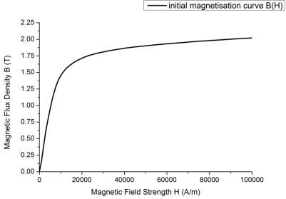
Fig. 5.9 Initial magnetisation curve of R260 rail steel.
