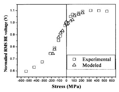
Fig. 3.54 Stress dependence of the normalised root-mean-square of measured and simulated Barkhausen signals obtained for AISI 410 stainless steel [73].
