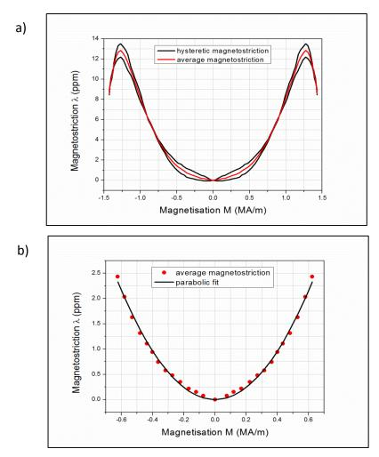
Fig. 2.12 a) Magnetostriction as function of magnetisation  $\mathbf{M}$  in 2% Mn pipeline steel [13]; b) Average magnetostriction as function of  $\mathbf{M}$  with parabolic approximation in low magnetisation region in 2% Mn pipeline steel.
