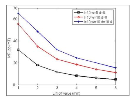
Fig. 3.24 Variation of the peak-to-peak MFL signal with sensor lift-off for three different cases of cuboid defect in steel plate (I-length, w-width, d-depth of the defect) [60].
