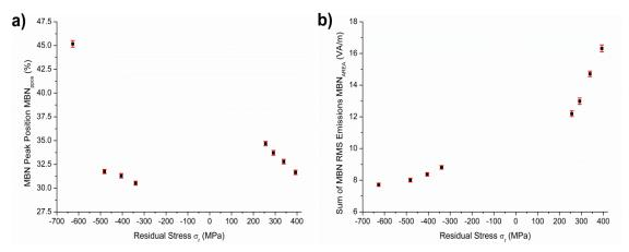
Fig. 4.29 a) MBN envelopes peak positions obtained for SAE9310 RS samples; b) Variation in area of MBN signal envelopes acquired for SAE9310 RS samples. Red bars reflect the standard deviation from the mean data values.
