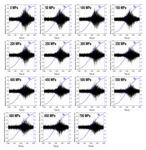
Fig. 4.20 Barkhausen voltage bursts acquired for SAE6481 TS1 sample under various applied tension.
