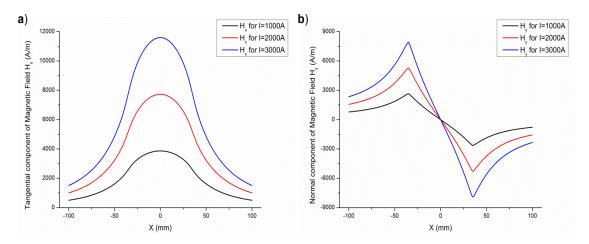
Fig. 5.4 a)&b) Distributions of tangential  $H_x$  and normal  $H_y$  components at 1mm above rectangular rail heads carrying currents of 1000A, 2000A and 3000A.
