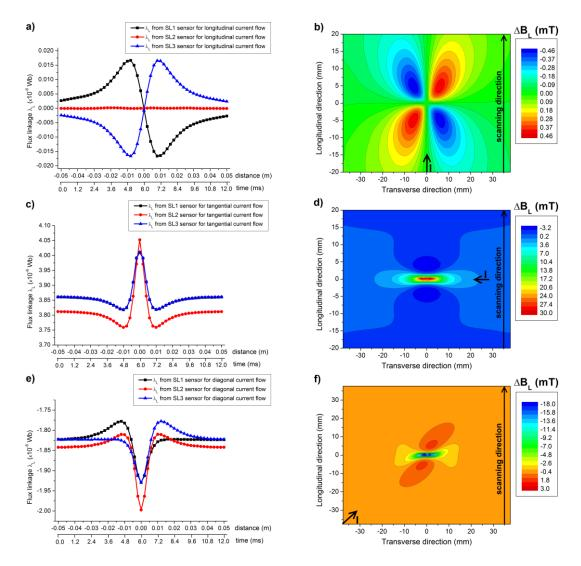
Fig. 5.55 Flux linkage signals from longitudinal sensors SL1, SL2 and SL3 probed above rails with surface centre flaws energised: a) longitudinally, c) tangentially and e) diagonally. Corresponding distributions of effective changes in longitudinal component  $\Delta B_L$  obtained above rails with surface centre flaws energised: b) longitudinally, d) tangentially and f) diagonally.
