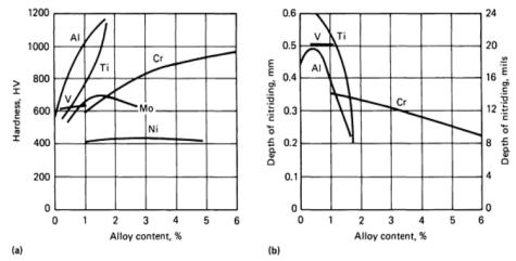
Fig. 3.4 Influence of alloying elements on: a) hardness after nitriding (base alloy, 0.35% C, 0.30% Si, 0.70%Mn) and b) depth of nitriding measured at 400 HV (nitriding for 8 h at 520 °C) [33].
