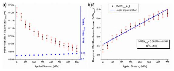
Fig. 4.23 a) MBN root-mean-square amplitude as a function of applied stress for SAE6481 TS1 sample;b) Dependence of reciprocal MBN root-mean-square on applied stress approximated with linear function. Red bars reflect the standard deviation from the mean data values.
