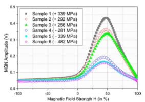
Fig. 6. Envelope curves of the rectified MBN bursts for carburized SAE 9310 specimens for different amplitudes of residual stress.
