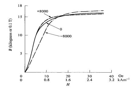
Fig. 3.46 Illustration of Villari reversal in pure iron [1].
