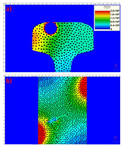
Fig. 5.38 Distributions of current density **J** within a) transverse cross-section and b) longitudinal crosssection of diagonally energised rail with side transverse flaw.
