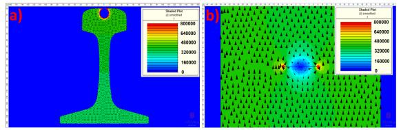
Fig. 5.18 Distributions of current density **J** within a) transverse cross-section and b) longitudinal crosssection of longitudinally energised flawed rail.
