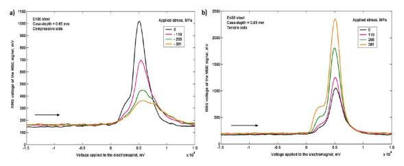
Fig. 4.34 MBN envelopes obtained by Moorthy for the EN36 specimen with carburised case-depth of 0.65mm subjected to various applied stress [91].
