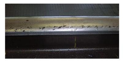
Fig. 3.12 Illustration of the fatigue induced rail head checking [40].
