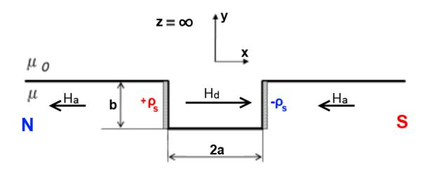
Fig. 3.21 Illustration of the principal of the leakage field dipole model for rectangular flaw proposed by Zatsepin and Shcherbinin [56].
