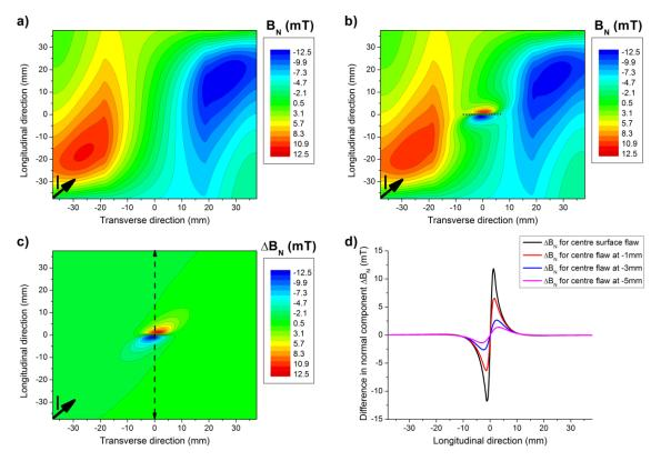
Fig. 5.36 Distributions of normal component of magnetic field at 1mm above diagonally energised: a) unflawed rail and b) flawed rail; c) Differential distribution  $\Delta B_N$  indicating effective perturbation in normal component of magnetic field above surface flawed rail; d) Numerical profiles of differential perturbations in normal component probed above diagonally energised rails with surface and subsurface flaws.
