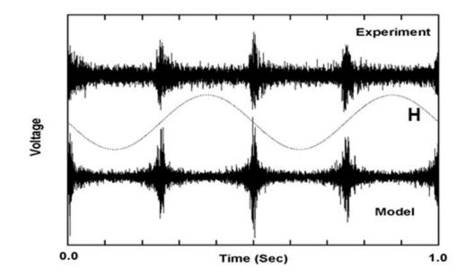
Fig. 2.20 Comparison of experimental and modelled Barkhausen signals obtained for iron specimen with 0.05%C [24].
