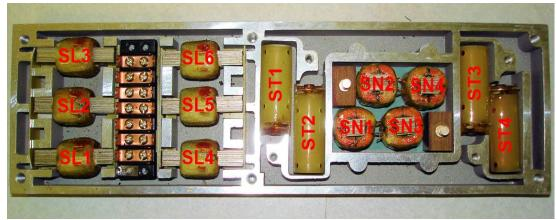
Fig. 5.6 Illustration of the Sperry induction sensors layout.
