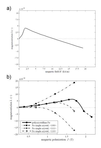
Fig. 3.47 a) Anhysteretic magnetostriction of iron as function of magnetic field; b) Magnetostrictive behaviour of polycrystalline and single crystal iron magnetised along principal directions [92] [93].
