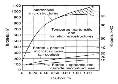
Fig. 3.1 Hardness as a function of carbon content for various microstructures in steels [31].
