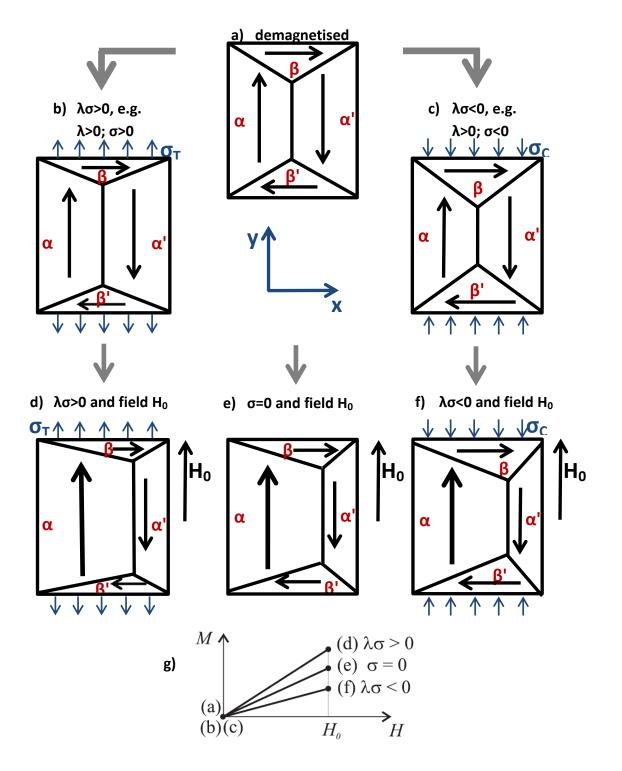
Fig. 2.10 a) to c) Schematic domain structures in unstressed and stressed bcc ferromagnetic material with no external field, d) to f) Schematic domain structures in unstressed and stressed bcc ferromagnetic material subjected to external field  $H_0$ , g) Illustrative plot of changes in magnetisation **M** with applied field  $H_0$  in unstressed and stressed bcc ferromagnetic material.
