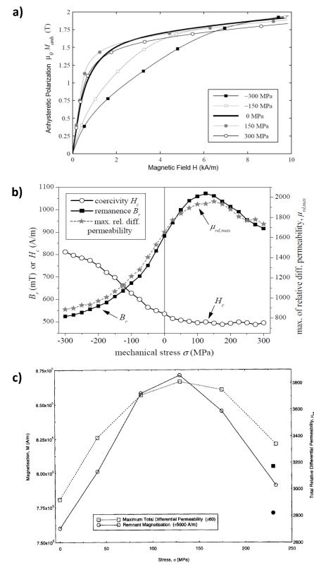
Fig. 3.30 a) Anhysteretic magnetisation curves for low carbon steel under different tensile loads; b) Variation of hysteretic parameters of low carbon steel with applied stress; c) Variation of maximum differential permeability and remanence of 50D pearlitic steel with tensile stress [68,70].
