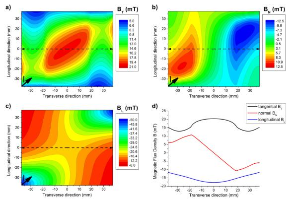
Fig. 5.33 Distributions of a) tangential component; b) normal component and c) longitudinal component of magnetic field at 1mm above central section of diagonally energised unflawed rail; d) Numerical profiles of these magnetic field components probed in the regions indicated by the arrows.
