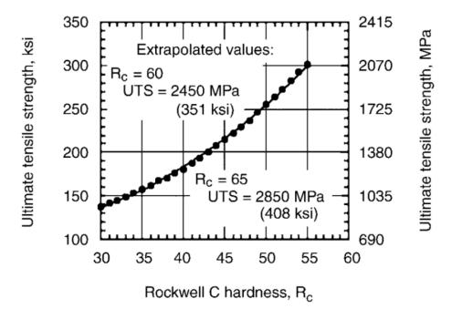
Fig. 3.2 Ultimate tensile stress of quenched and tempered steels as a function of hardness [32].
