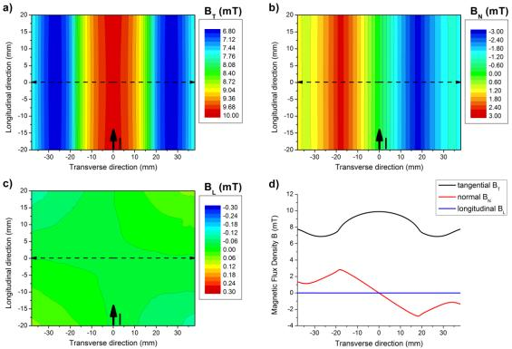
Fig. 5.17 Distributions of a) tangential component; b) normal component and c) longitudinal component of magnetic field at 1mm above central section of longitudinally energised unflawed rail; d) Numerical profiles of these magnetic field components probed in the regions indicated by the arrows.
