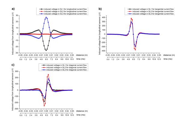
Fig. 5.56 Induced voltage signals from longitudinal sensors SL1, SL2 and SL3 probed above rails with surface centre flaws energised: a) longitudinally, c) tangentially and e) diagonally at speed rate of 30km/h.
