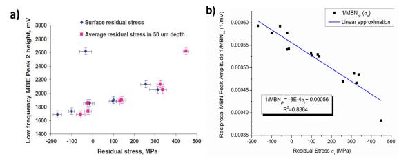
Fig. 4.39 a) Low-frequency MBN peak amplitude as a function of surface residual stress in EN36 samples [122]; b) Dependence of reciprocal low-frequency MBN peak amplitude on residual stress approximated with linear function, after Moorthy et al. [122].
