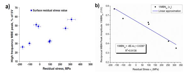
Fig. 4.38 a) High-frequency MBN peak amplitude as a function of surface residual stress in EN36 samples [120]; b) Dependence of reciprocal high-frequency MBN peak amplitude on residual stress approximated with linear function, after Moorthy et al. [122].
