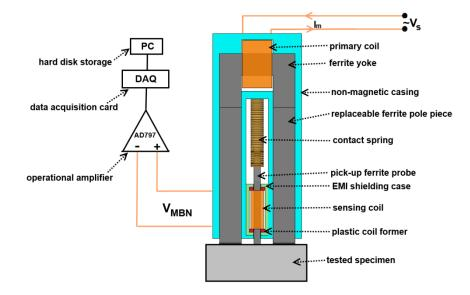
Fig. 4.6 Schematic diagram of the Barkhausen Noise measurement set-up.
