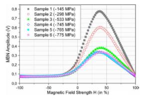
Fig. 7. Envelope curves of the rectified MBN bursts for 32CDV13 specimens for different amplitudes of residual stress.
