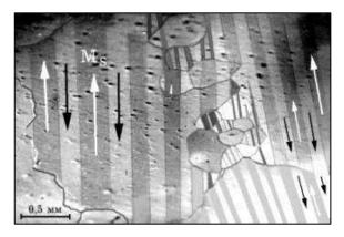
Fig. 2.1 Illustrative representation of domain structure in silicon steel (3% Si-Fe) [3].
