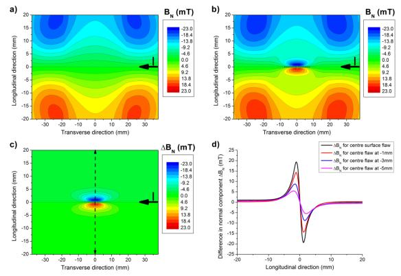
Fig. 5.28 Distributions of normal component of magnetic field at 1mm above tangentially energised: a) unflawed rail and b) flawed rail; c) Differential distribution  $\Delta B_N$  indicating effective perturbation in normal component of magnetic field above surface flawed rail; d) Numerical profiles of differential perturbations in normal component probed above tangentially energised rails with surface and subsurface flaws.
