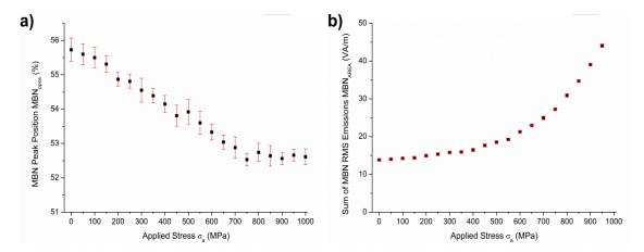
Fig. 4.19 a) MBN envelopes peak positions obtained for SAE9310 TS2 sample under various tension; b) Variation in area of MBN signal envelopes for TS2 sample subjected to different levels of tension. Red bars reflect the standard deviation from the mean data values.
