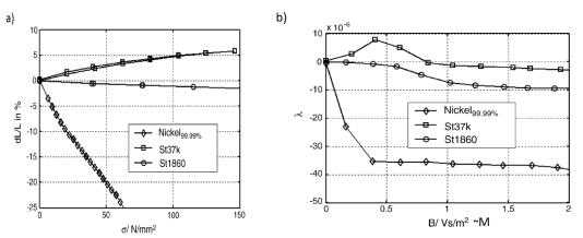
Fig. 3.16 a) Percentage changes in coil inductance with stress obtained from EC evaluation of nickel, St37k and St1860 steels; b) corresponding magnetostriction curves for tested samples of nickel, St37k and St1860 steels [48].
