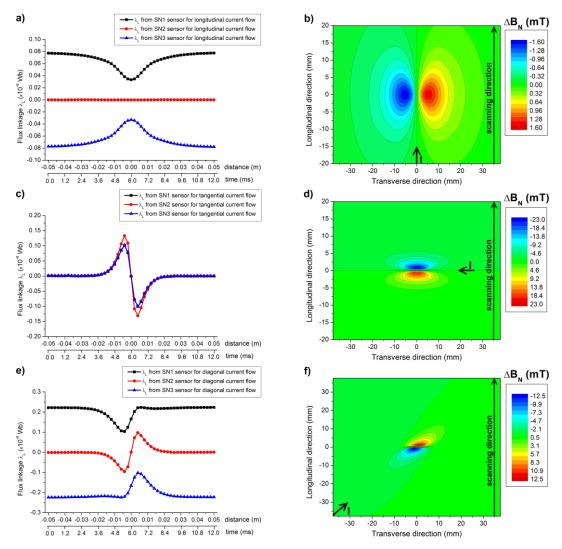
Fig. 5.53 Flux linkage signals from normal sensors SN1, SN2 and SN3 probed above rails with surface centre flaws energised: a) longitudinally, c) tangentially and e) diagonally. Corresponding distributions of effective changes in normal component  $\Delta B_N$  obtained above rails with surface centre flaws energised: b) longitudinally, d) tangentially and f) diagonally.
