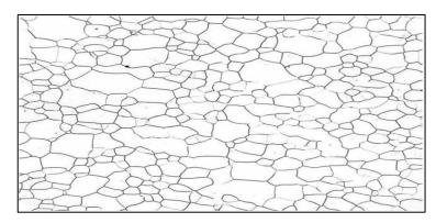
Fig. 3.37 Typical ferritic steel microstructure [88].
