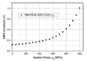
Fig. 2. MBN peak amplitude for carburized SAE 9310 specimen as a function of applied stress.
