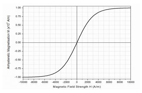
Fig. 2.9 Typical anhysteretic magnetisation curve for ferromagnetic material.
