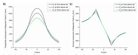
Fig. 5.2 a) Indication of the regions in which the profiles of tangential and normal components of magnetic field were simulated; b) & c) Distributions of tangential  $H_x$  and normal  $H_y$  components at different levels above a rectangular approximation of a rail head carrying current of 3000A.
