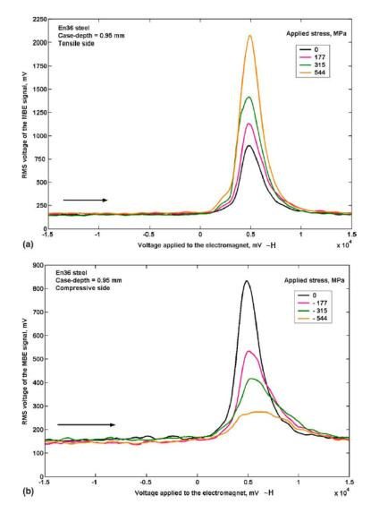
Fig. 3.45 Influence of a) tension and b) compression on Magnetic Barkhausen Noise in EN36 steel [91].
