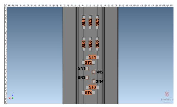
Fig. 5.42 FEM sensor set-up comprising three groups of directional sensors.
