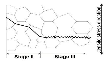
Fig. 3.7 Illustration of fatigue crack growth stages II and III in crystalline material.
