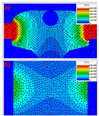
Fig. 5.26 Distributions of current density **J** within a) transverse cross-section and b) longitudinal crosssection of tangentially energised rail with centre transverse flaw.
