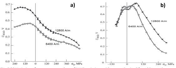
Fig. 3.33 Variation of mean-square values of MAE emissions with stress obtained for: a) low carbon steel and b) nickel, subjected to magnetic fields of 6400A/m and 12800A/m [78].
