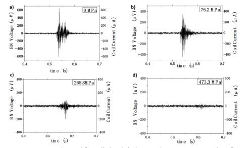
Fig. 3.51 MBN emissions obtained for rolled nickel plates under various magnitudes of tensile stress [109].
