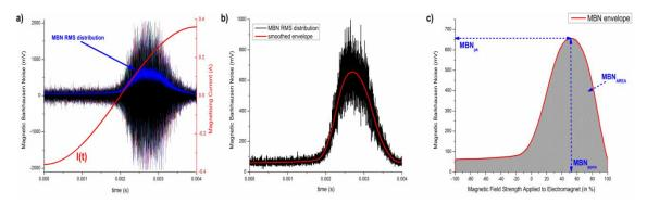
Fig. 3.36 a) Illustration of raw Barkhausen bursts and corresponding root mean square distribution of their instantaneous voltage pulses; b) Extraction of smoothed envelope of MBN RMS distribution; c) Smoothed MBN envelope with indicated analysis parameters.
