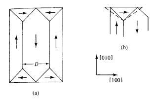
Fig. 2.4. Closure domains of cubic crystal in iron [1].
