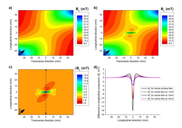
Fig. 5.37 Distributions of longitudinal component of magnetic field at 1mm above diagonally energised: a) unflawed rail and b) flawed rail; c) Differential distribution  $\Delta \mathbf{B}_{L}$  indicating effective perturbation in longitudinal component of magnetic field above surface flawed rail; d) Numerical profiles of differential perturbations in longitudinal component probed above diagonally energised rails with surface and subsurface flaws.
