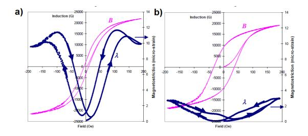
Fig. 3.49 Magnetostriction butterfly loops with corresponding hysteresis signatures obtained for a) ferrite/pearlite and b) martensitic steel microstructures [94].
