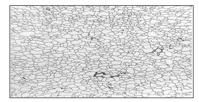
Fig. 3.38 Cementite (dark regions) in the form of particles at ferrite grain boundaries [88].
