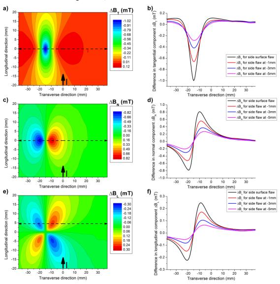
Fig. 5.23 Differential distributions of: a) tangential component; c) normal component and e) longitudinal component of magnetic field above surface side-flawed rail energised in longitudinal direction. Numerical profiles of differential perturbations in b) tangential component; d) normal component and f) longitudinal component of magnetic field probed above longitudinally energised rails with surface and sub-surface flaws.
