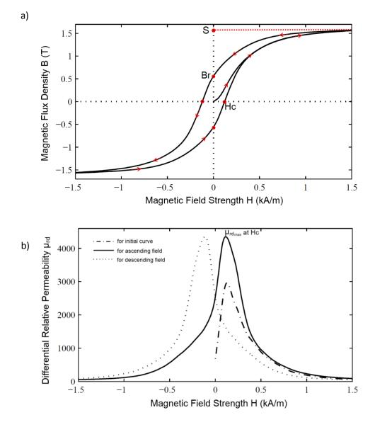
Fig. 2.8 Graphical illustration of magnetisation process in pure iron: a) initial magnetisation curve and hysteresis loop for pure iron; b) differential relative permeability as function of applied field in pure iron.
