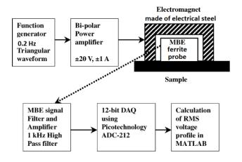
Fig. 4.33 MBN measurement set-up used in work of Moorthy et al [91].
