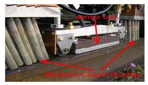
Fig. 5.5 Illustration of Sperry Induction Sensing Unit (ISU).
