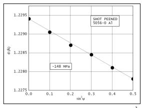
Fig. 3.19 Linear dependence of the measured lattice spacing with  $\sin^2 \psi$  for shot-peened 5056-0 aluminium [50].
