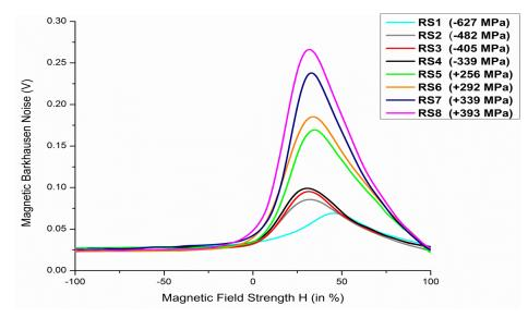
Fig. 4.26 Magnetic Barkhausen Noise signal envelopes obtained for SAE9310 RS samples with various levels of surface residual stress.
