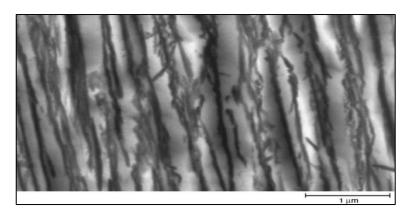
Fig. 3.39 Cementite (dark regions) in the form of filaments dispersed in a ferrite matrix in bainite microstructure [88].
