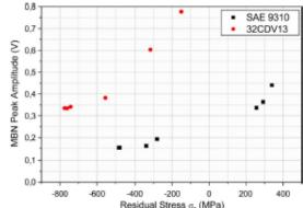
Fig. 8. MBN peak amplitude for carburized SAE 9310 and 32CDV13 specimens as a function of residual stress.
