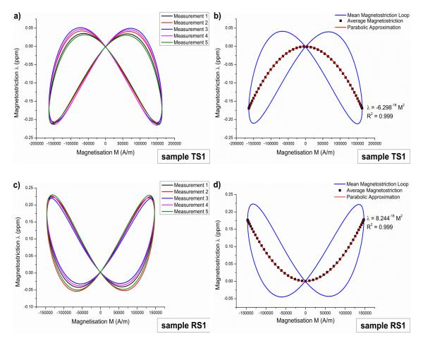
Fig. 4.14 a) & c) Minor AC magnetostriction butterfly loops measured for nitrided SAE6481 and carburised SAE9310 samples, respectively; b) & d) Mean AC magnetostriction butterfly loops for nitrided SAE6481 and carburised SAE9310 samples with corresponding average values of  $\lambda$  vs **M** approximated by parabolic function.
