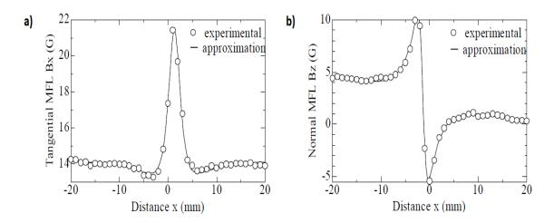
Fig. 3.22 Experimental profiles of tangential and normal components of MFL signals approximated with Z-S dipole model for case of rectangular flaw in steel plate [58].
