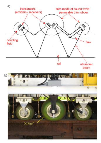
Fig. 3.10 a) Schematic diagram of the principal of ultrasonic rail inspection with Sperry X-fire system (refraction of ultrasonic beams has been neglected), b) photography of the X-fire set-up taken during the in-situ rail testing [40].
