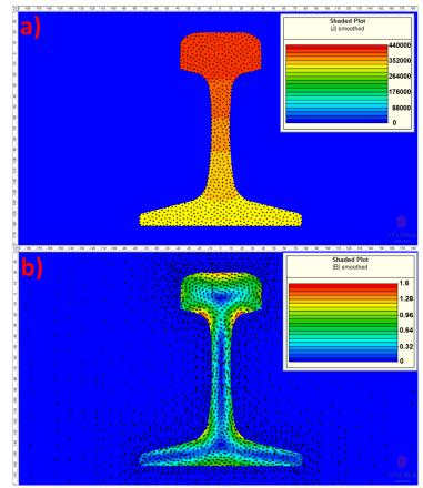
Fig. 5.15 Distributions of a) current density **J** and b) flux density **B** within and outside the unflawed rail energised along the longitudinal direction.
