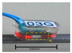
Fig. 3.15 EC stress measurement probe positioned at the surface of tested sample rod with indicated linking flux path [48].
