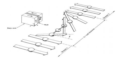
Fig 2.5 Structure of a 180° domain wall (Bloch wall) [1].
