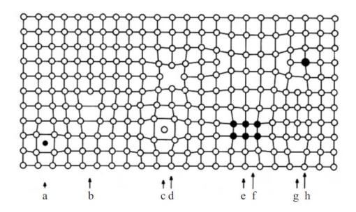
Fig. 2.16 Schematic overview of several types of crystal lattice defects [20].
