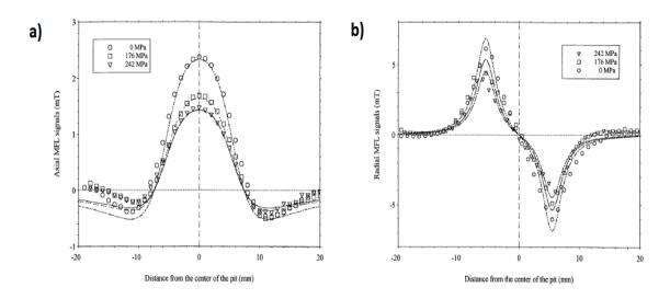
Fig. 3.23 Experimental profiles of tangential and normal components of MFL signals approximated with Z-S dipole model for case of corrosion flaw in steel pipeline subjected to various hoop stresses [59].
