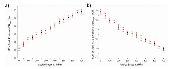
Fig. 4.24 a) MBN envelopes peak positions obtained for SAE6481 TS1 sample under various tension; b) Variation in area of MBN signal envelopes for TS1 sample subjected to different levels of tension. Red bars reflect the standard deviation from the mean data values.
