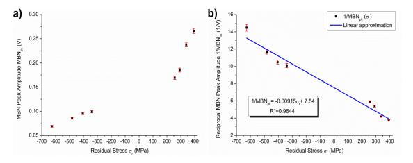
Fig. 4.27 a) MBN peak amplitude as a function of residual stress for SAE9310 RS samples; b) Dependence of reciprocal MBN peak amplitude on residual stress approximated with linear function. Red bars reflect the standard deviation from the mean data values.
