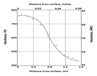
Fig. 3.3 Microhardness depth profile of SAE 8620 steel test bar after gas carburization [33].
