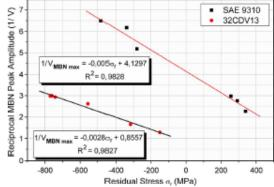
Fig. 9. Reciprocal of MBN peak amplitude for carburized SAE 9310 and 32CDV13 specimens as a function of residual stress.
