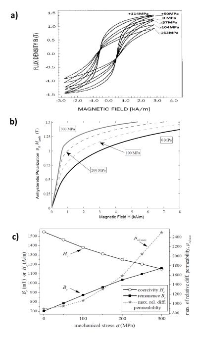
Fig. 3.28 a) Hysteresis loops for XC10 steel subjected to various applied stresses; b) Anhysteretic magnetisation curves obtained for M250 steel under different tensile loads; c) Variation of hysteretic parameters of M250 steel with tensile stress [65, 70].
