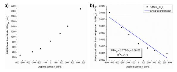
Fig. 4.37 a) MBN peak amplitude as a function of applied stress for EN36 sample with 0.95mm casedepth [91]; b) Dependence of reciprocal MBN peak amplitude on applied stress approximated with linear function.
