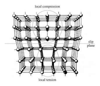
Fig. 2.17 Illustration of the micro-stress distribution around an edge dislocation [20].
