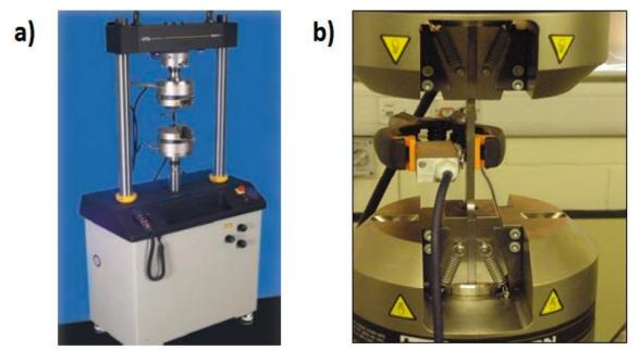
Fig. 4.10 a) Image of Instron 8801 servo-hydraulic system [118]; b) Illustration of the MBN sensor clamped at the centre of gauge section of specimen subjected to tensile stress.
