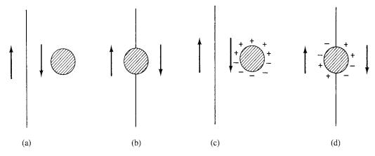
Fig. 2.15 Interaction of domain walls with inclusions [1].
