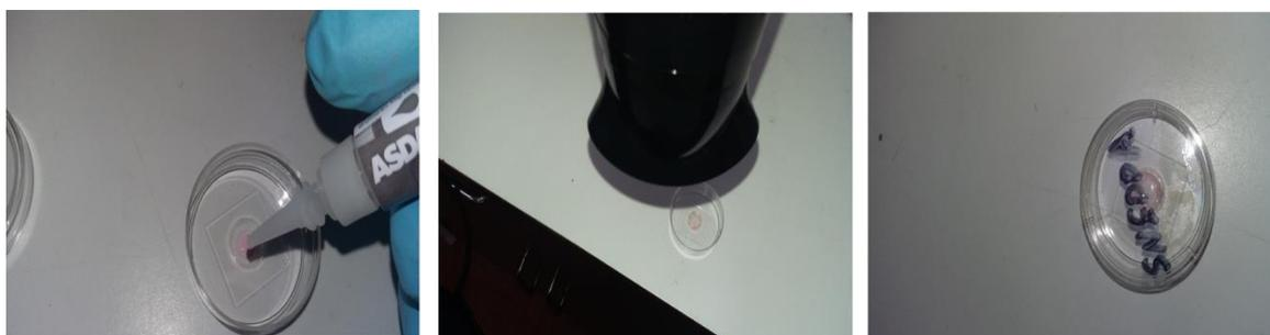
**Figure 2.7:** Measurement of  $\sigma$  by gluing the particles into the glass bottom dish.
