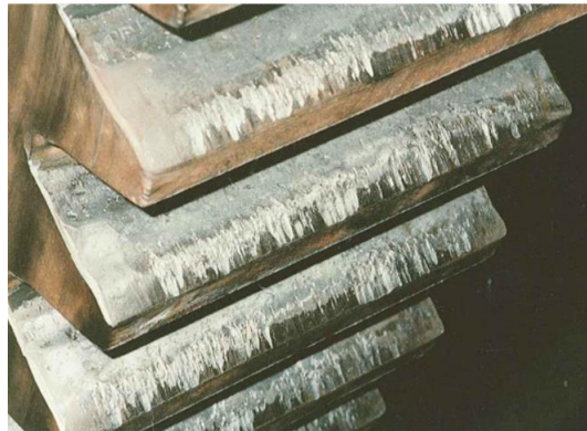
Figure 1.3 - Scuffing due to metal parts rubbing each other at gear teeth.(Novexa.com, 2015)
