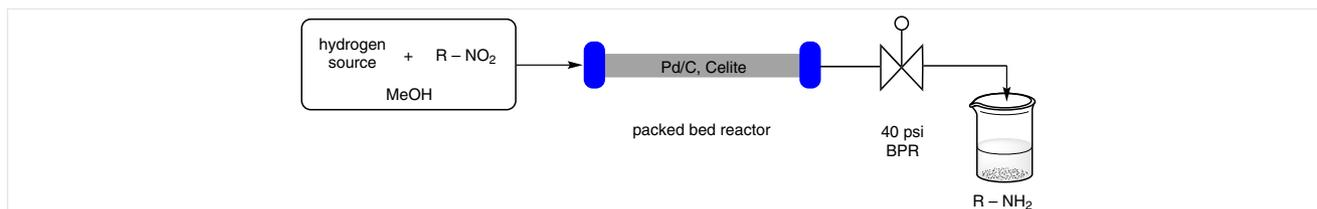
**Figure 1** Flow setup for the reduction of nitro compounds using a packed-bed reactor in flow
