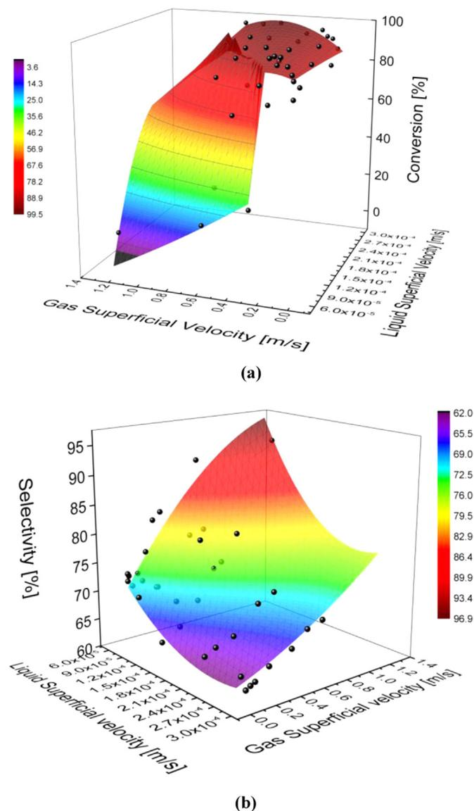
**Fig. 13.** Response surfaces: (a) conversion as a function of gas and liquid superficial velocities; (b) selectivity to benzaldehyde as a function of gas and liquid superficial velocities. In the graphs experimental points are indicated by black spheres.
