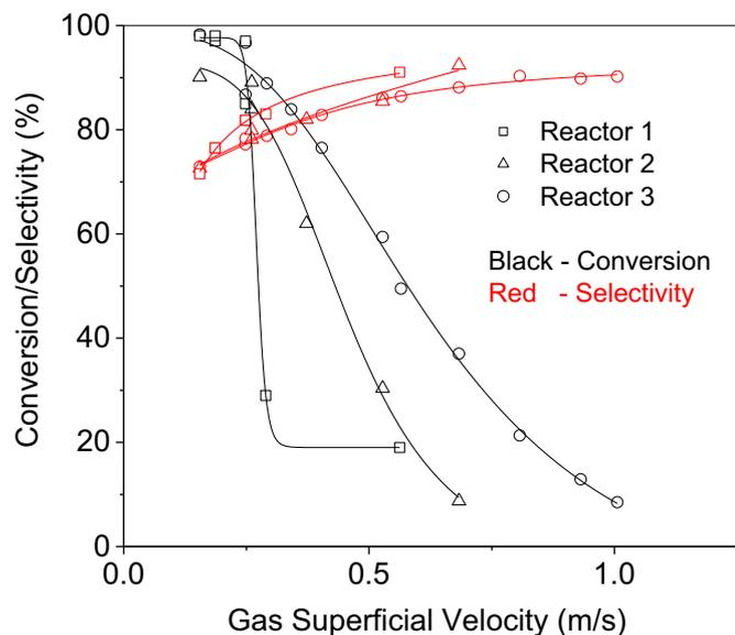
Fig. 9. Repeatability in the gas-continuous (partially wetted) flow regime using three different reactors, each re-packed with a new bed of catalyst. Liquid superficial velocity:  $6.94 \times 10^{-5}$  m/s, Catalyst mass: 1 mg.
