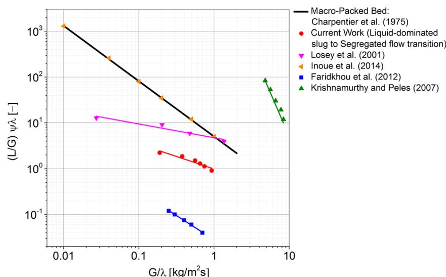
**Fig. 6.** Flow map comparison of a conventional trickle bed reactor: Charpentier and Favier (1975) and micro-packed reactors: Faridkhou and Larachi (2012), Losey et al.
