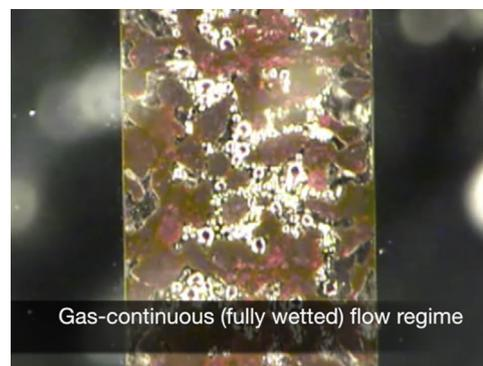
**Video 2.** Optical microscope observation of the hydrodynamics during gas-continuous (fully wetted) flow regime,  $u_L=6.9\times 10^{-5}$  m/s,  $u_G=0.24$  m/s. Supplementary material related to this article can be found online at <http://dx.doi.org/10.1016/j.ces.2016.03.018>.
