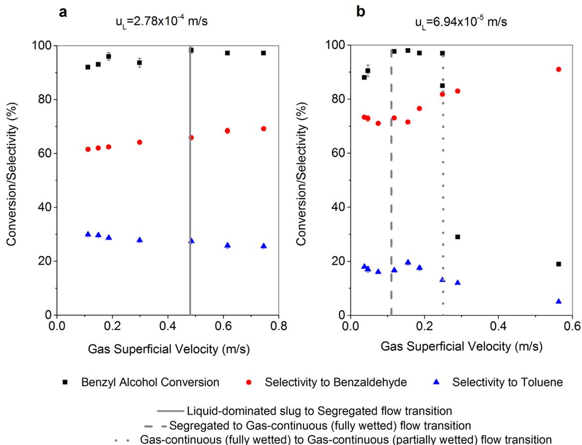
**Fig. 7.** Conversion of benzyl alcohol and selectivity to benzaldehyde and toluene at various flow regimes obtained by increasing gas flow rate. (a) Liquid-dominated slug transitioning into segregated flow regime at liquid flow rate  $3 \mu\text{l}/\text{min}$  (b) segregated transitioning into gas-continuous (fully wetted) and subsequently to gas-continuous (partially wetted) flow regime at liquid flow rate  $0.75 \mu\text{l}/\text{min}$ .
