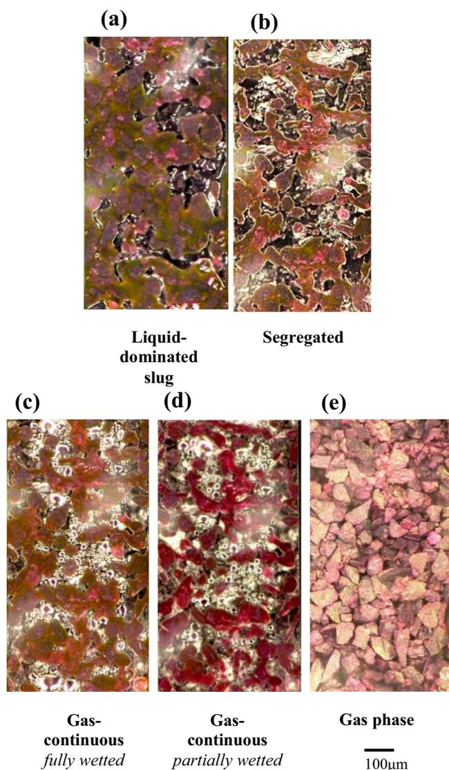
**Fig. 4.** Microscope images of the micro-packed bed reactor showing the flow regimes corresponding to Fig. 5. (a) Liquid-dominated slug (b) segregated (c) gas-continuous (fully wetted) (d) gas-continuous (partially wetted) and (e) gas phase.
