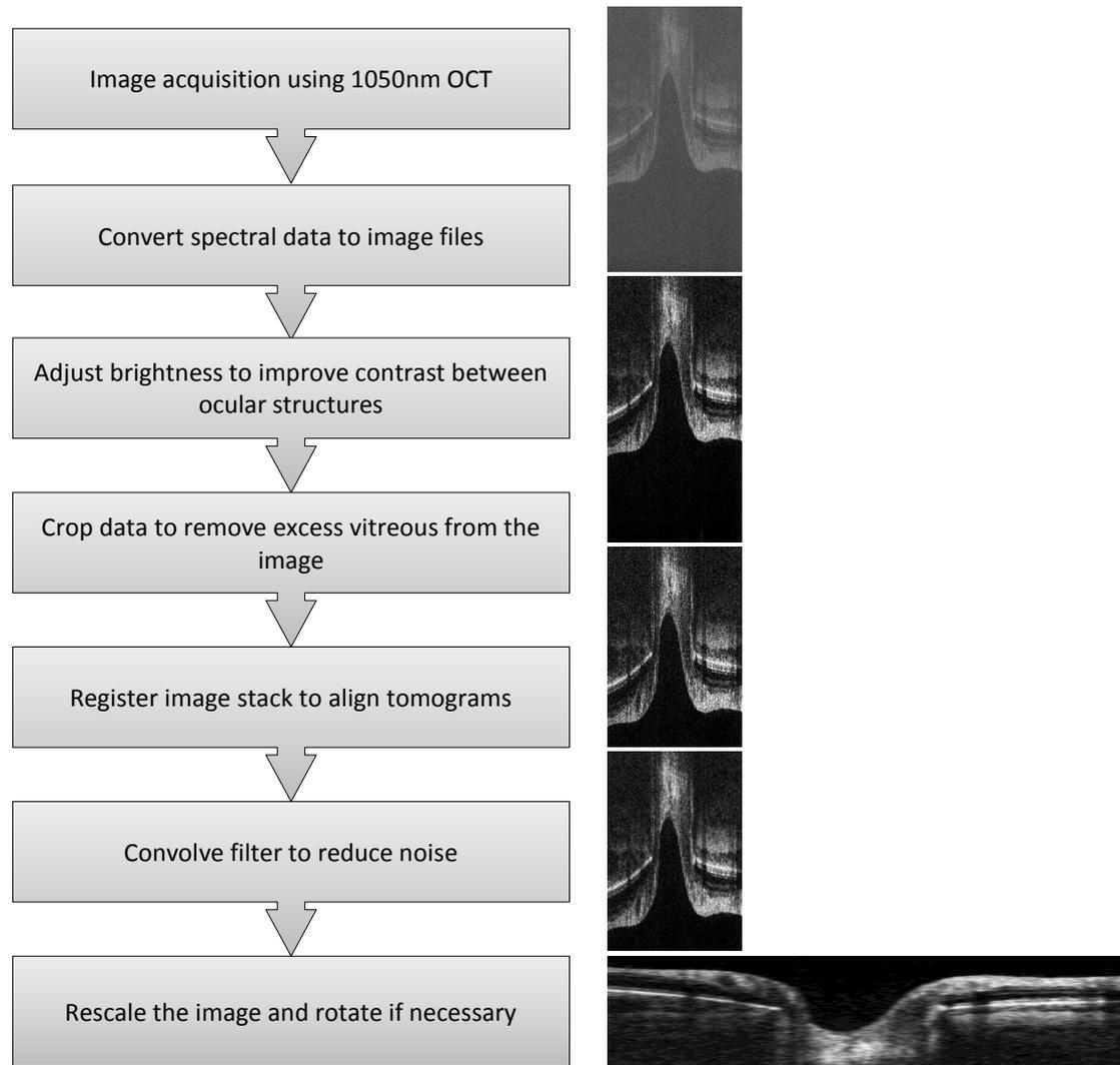
Figure 2.1: Flow chart showing data processing stages prior to measurements.
