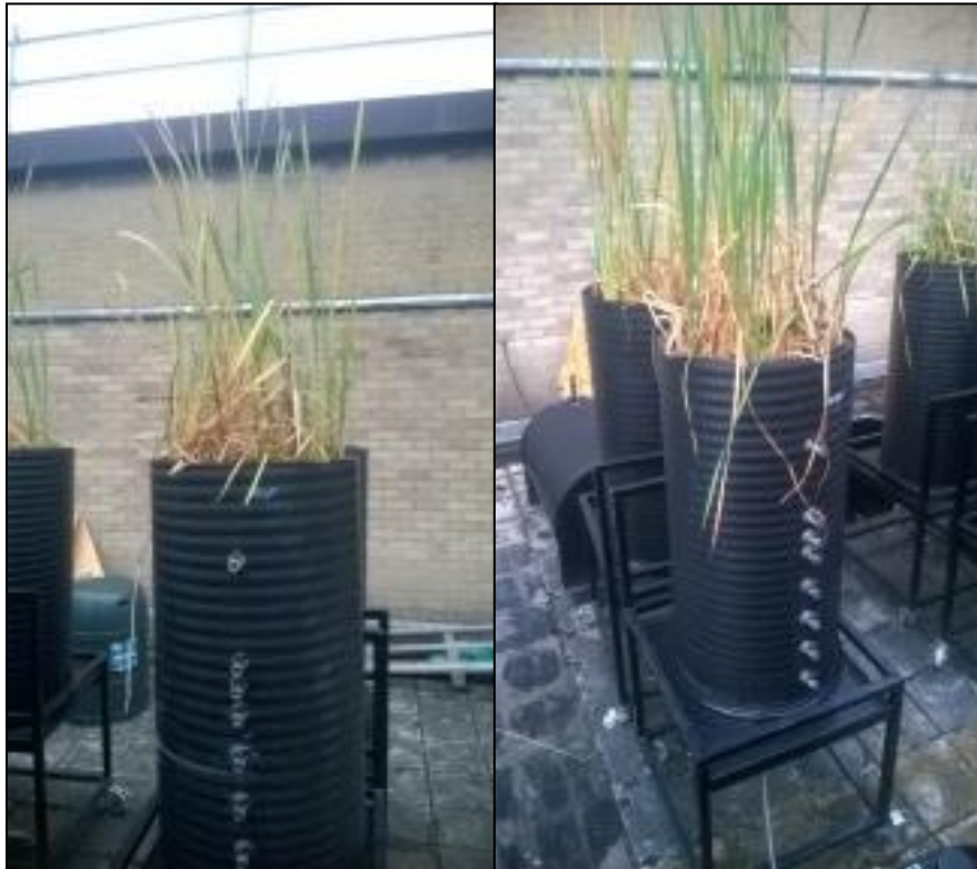
Figure 5-15 - Visible evidence of plant die off on 27/10/14
