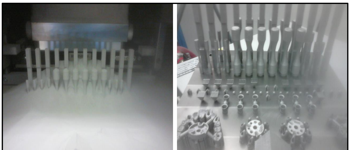
Figure 4 - Images Showing Completed Build and Powder to be swept to Overflow
