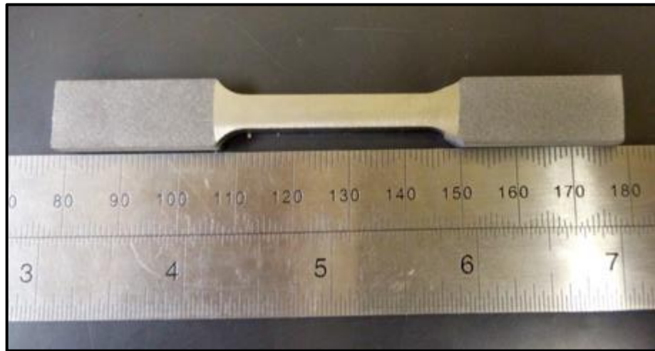
Figure 36 - Image of Machined Tensile Test Specimen.
