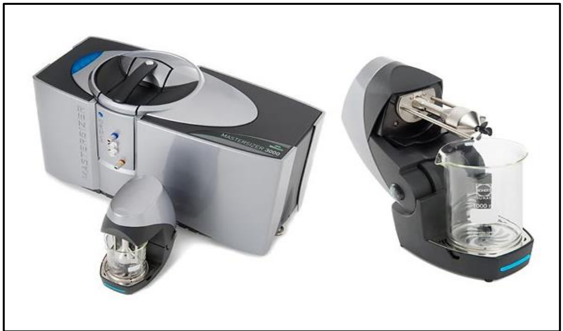
Figure 9 - Image Showing Malvern Mastersizer 3000 with Centrifugal Pump and Stirrer Unit (Malvern, 2015).
