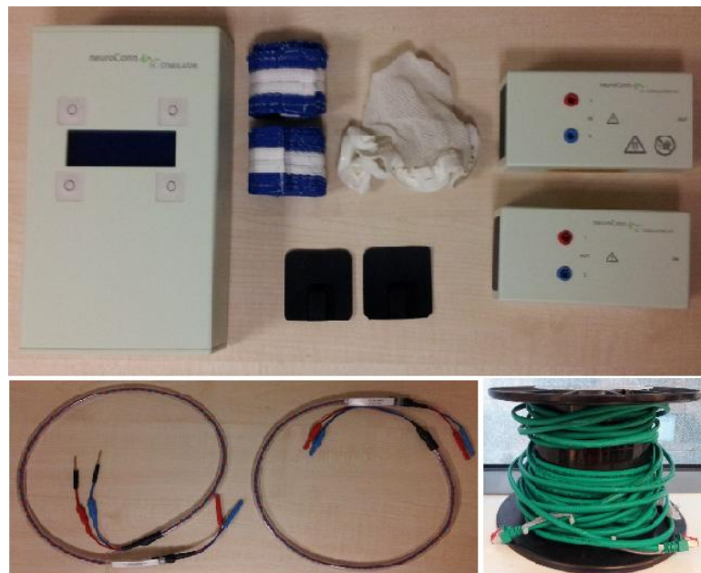
Figure 4.1. tDCS-MEG components. Top-Bottom, Left-Right: tDCS device, head bands with Velcro attachments, scalp cap, tDCS electrodes (25 cm 2 ), non-shielded filter box (located in electronics room), shielded filter box (located in MSR), connector cables (electrode cable; stimulator cable), extension cable.
