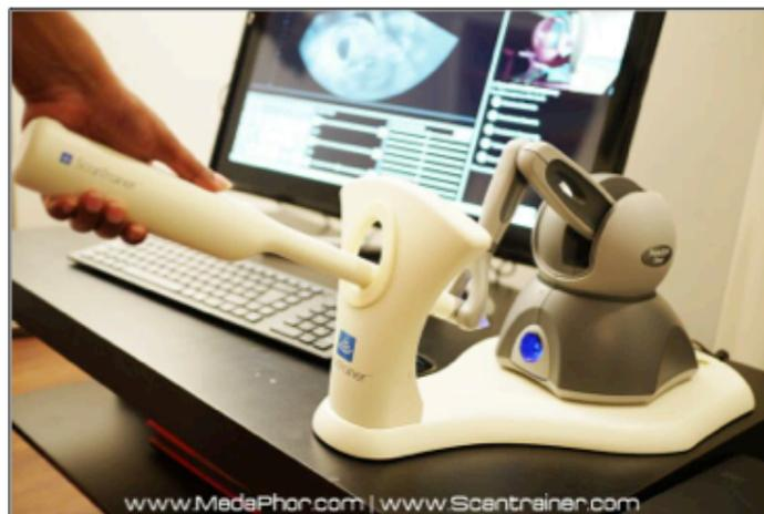
Figure (2.5): The haptic device includes: (1) the base of the device, (2) probe stand, (3) the probe, and (4) the haptic tool which connects to the computer. This figure shows the method of ‘dock and re-dock’ the probe into and out of the haptic body.
