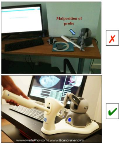
Figure (2.5): The haptic device includes: (1) the base of the device, (2) probe stand, (3) the probe, and (4) the haptic tool which connects to the computer. This figure shows the method of 'dock and re-dock' the probe into and out of the haptic body.
