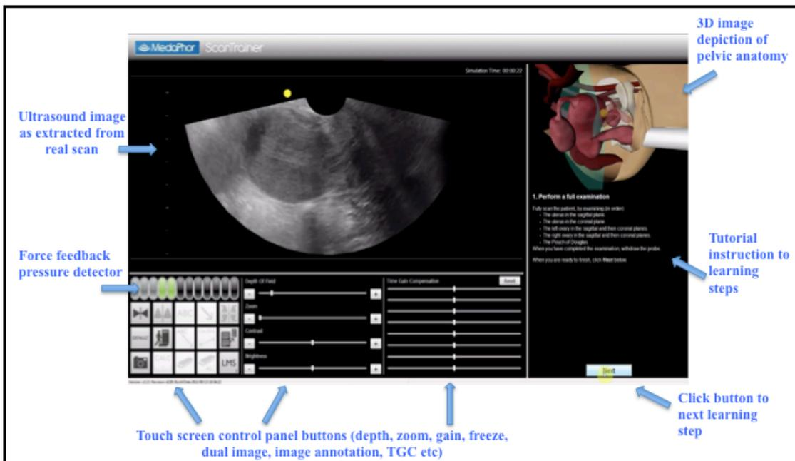
**Figure (2.2):** Learning contents as (it) operated by the ultrasound simulator ScanTrainer<sup>®</sup>
