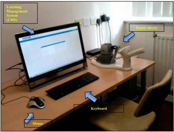
**Figure (2.1)**: The ultrasound simulator ScanTrainer<sup>®</sup> consists of (1) a monitor which represents learning contents as programmed by specific learning software, and connects to (2) a haptic device, (3) mouse and (4) keyboard.
