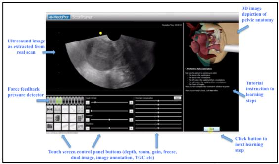
Figure (2.2): Learning contents as (it) operated by the ultrasound simulator ScanTrainer®
