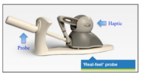
Figure (2.4): Haptic device
