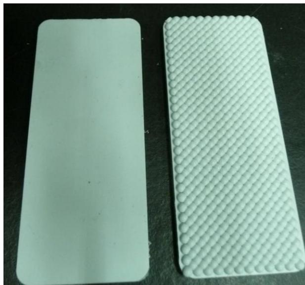
**Figure 5-3: Rectangular samples with flat (left) and textured (right) surfaces.**
