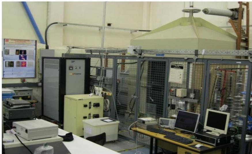
Figure 3-14: Test set-up of fog chamber tester (Cardiff University High Voltage Laboratory).
