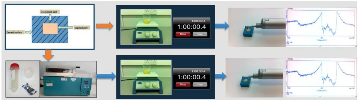
**Figure 77. Surface erosion test. Group A: immersing enamel samples in saliva for 1 hour then acidic solution for another 1 hour then measured by surfometer, Group B: Immersing enamel samples in solution for 1 hour then measured by surfometer.**
