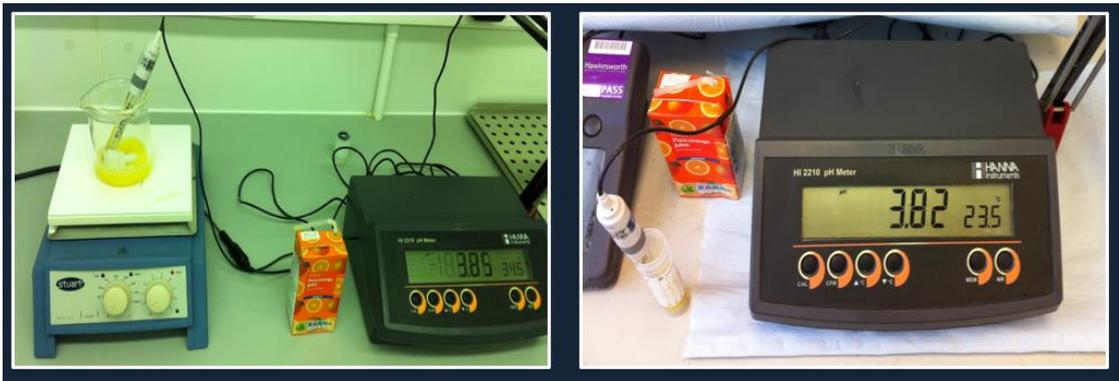
**Figure 55. Measuring pH at room and body temperatures.**
