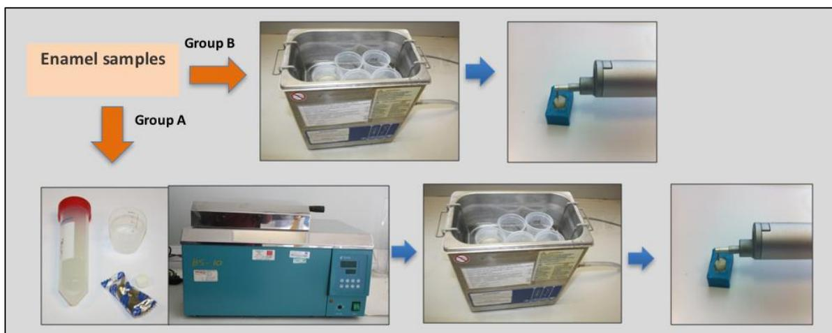
**Figure 82. Subsurface erosion test. Group A: immersing enamel samples in saliva for 1 hour then ultrasonication for 30 seconds then measured by surfometer, Group B: Immediate ultrasonication for 30 seconds then measured by surfometer.**
