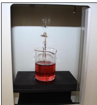
**Figure 60. Enamel sample attached to the electrobalance holder.**
