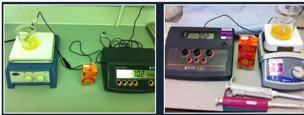
**Figure 57. Measuring neutralisable acidity at room and body temperatures.**
