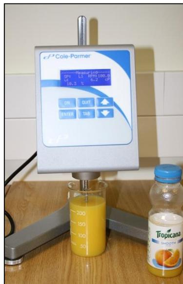
**Figure 66. The rotational viscometer with a sample to test.**
