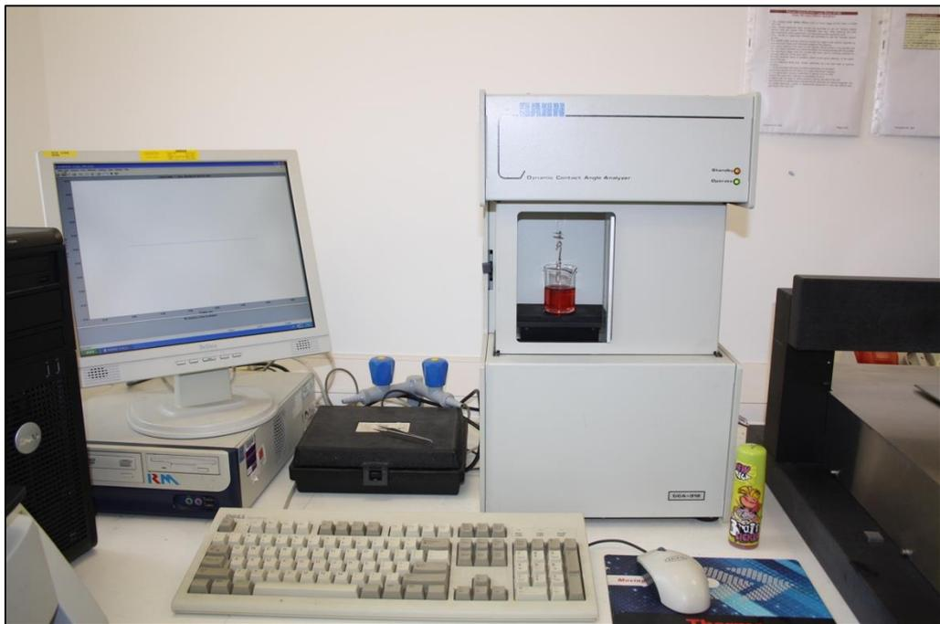
**Figure 61. The dynamic contact angle analyser.**
