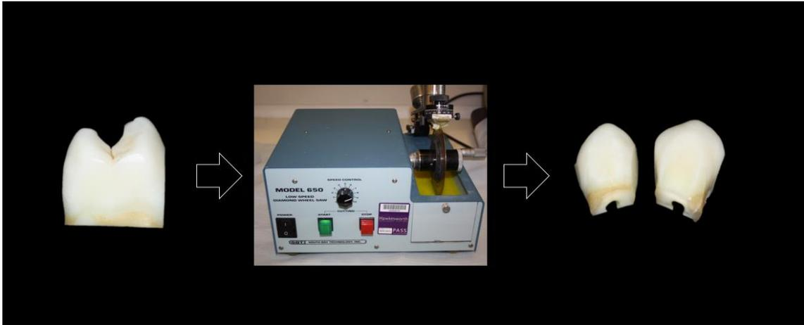
**Figure 52. Crown sectioning to obtain enamel specimens for erosion tests.**
