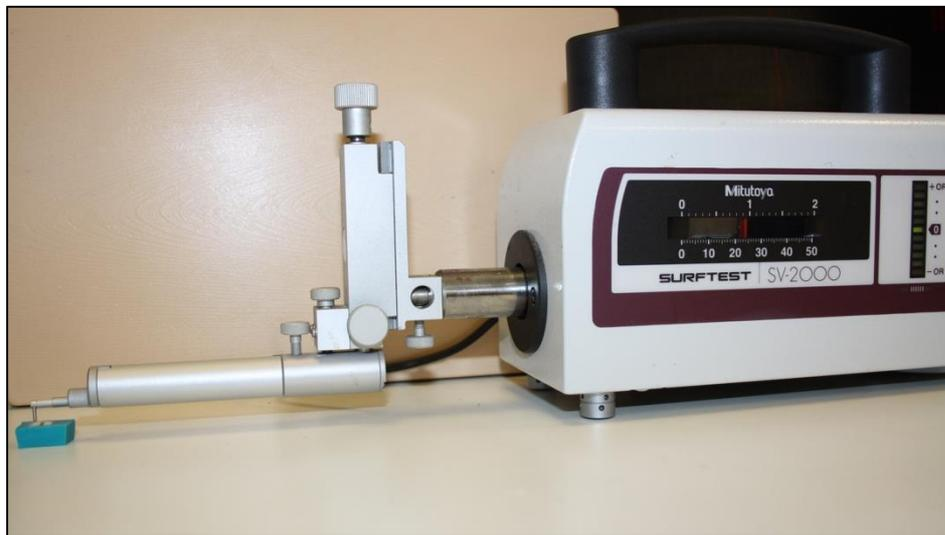
**Figure 50. Three baseline readings using a contact surfometer were undertaken.**
