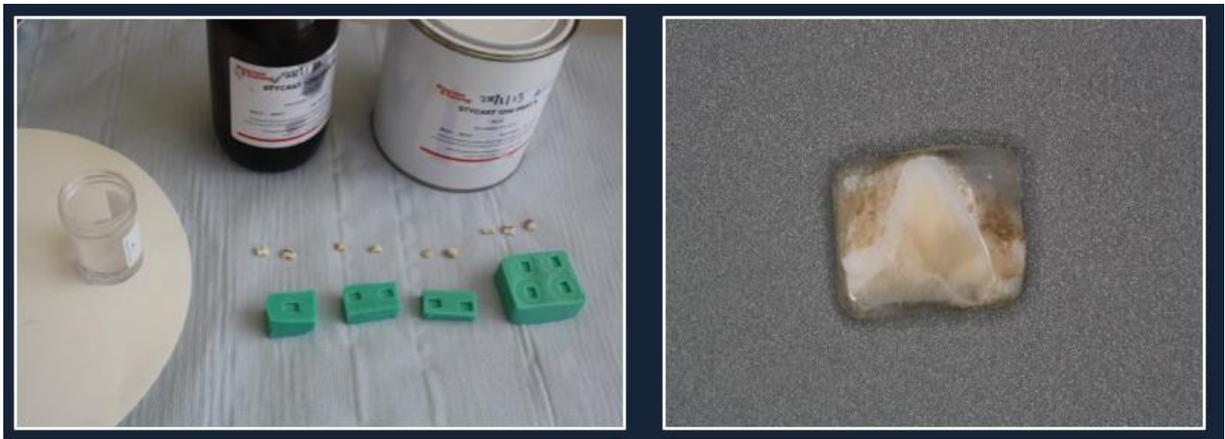
**Figure 53. Placement of enamel specimens in epoxy resin.**
