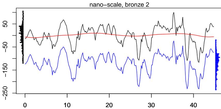
Figure 11: Roughness data of a bronze sample obtained by AFM: original (black), waviness (red) and profile with removed waviness (blue);  $x$ -scale unit is  $\mu m$ . The height distributions are given on the left and the right respectively.
