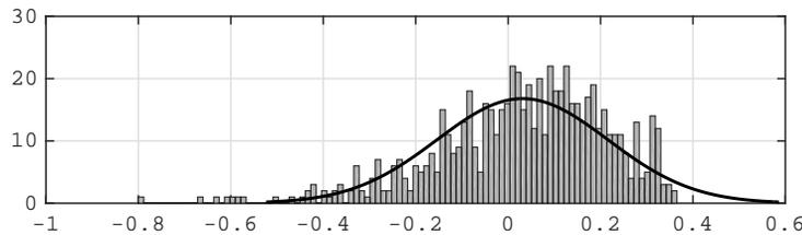
Figure 8: The histogram of heights for roughness data of steel obtained by a profilometre for the segment  $[0, 1000]$  with the fitted normal distribution,  $x$ -scale unit is  $\mu m$ , vertical scale is counts.
