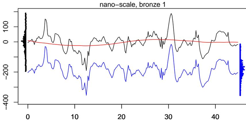
Figure 10: Roughness data of a bronze sample obtained by AFM: original (black), waviness (red) and profile with removed waviness (blue);  $x$ -scale unit is  $\mu m$ . The height distributions are given on the left and the right respectively.
