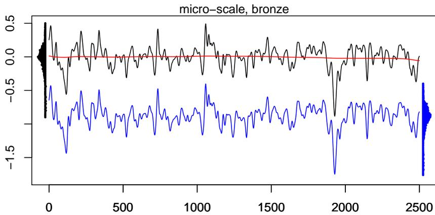
Figure 13: Roughness data of a bronze sample obtained by a profilometre: original (black), waviness (red) and profile with removed waviness (blue);  $x$ -scale unit is  $\mu m$ . The height distributions are given on the left and the right respectively.
