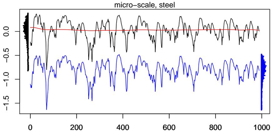
Figure 12: Roughness data of a steel sample obtained by a profilometre: original (black), waviness (red) and profile with removed waviness (blue);  $x$ -scale unit is  $\mu m$ . The height distributions are given on the left and the right respectively.
