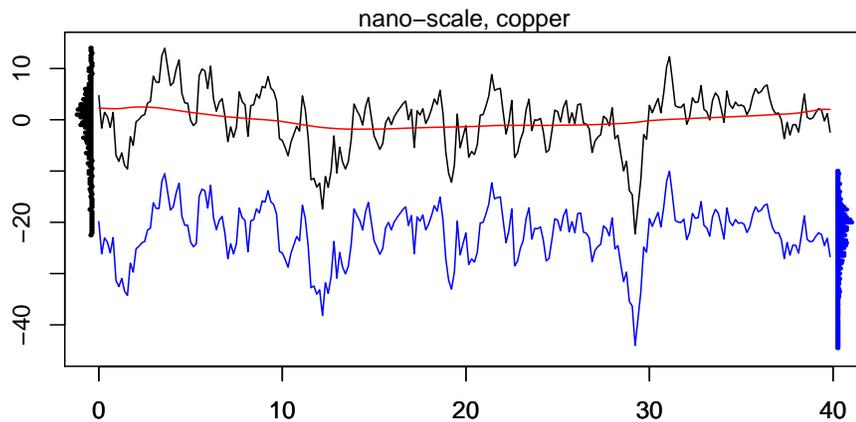
Figure 9: Roughness data of a copper sample obtained by AFM: original (black), waviness (red) and profile with removed waviness (blue);  $x$ -scale unit is  $\mu m$ . The height distributions are given on the left and the right respectively.
