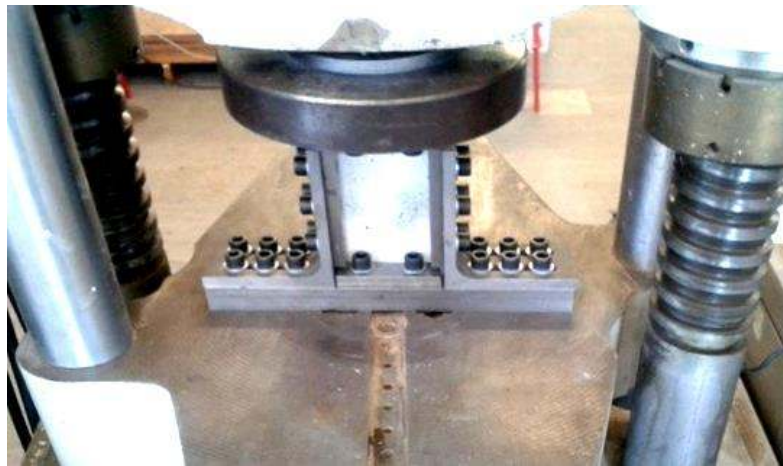
Figure 3: CAI specimen fitted in the compression rig
