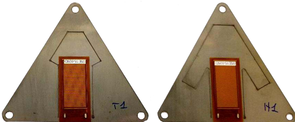
Figure 1: Energy Harvesting Units: tuned (left) and heavy (right)
