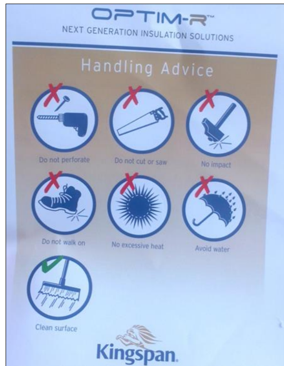
Figure 67: Photograph showing an example of non-verbal communication to installers from manufacturer of vacuum insulation panels
